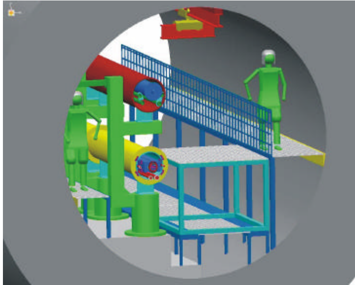
Figure 5.1: Schematic view of the tunnel with two synchrotron rings SIS100/200 [3]
