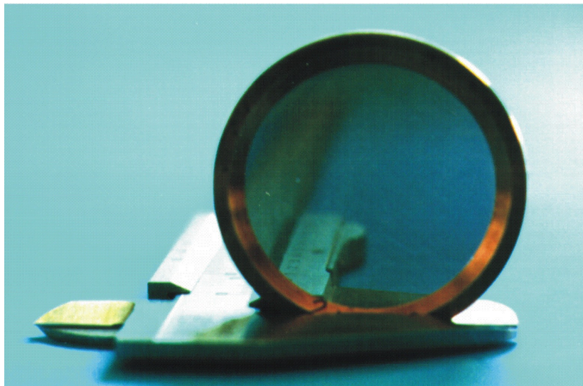
Figure 1.15: Photo of a carbon foil coated by CsI. The ions interact with the foil and produce secondary electrons.
