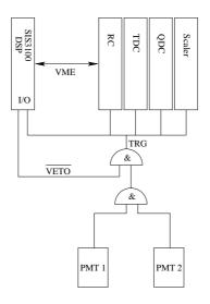
Figure 5.14: Diagram of the test beam trigger. Two PMTs produce the trigger in coincidence. The VETO signal has to be released during event processing.
