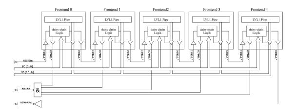
Figure 5.8: Daisy chained connection of five PFMs
