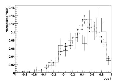
Figure 4.13: The measured angular distributions of the  $pK_S$  system. The solid line is given by the events whose mass corresponds to the mass of the observed peak. The dashed line corresponds to background events out of the two  $\sigma$ -range around a peak.
