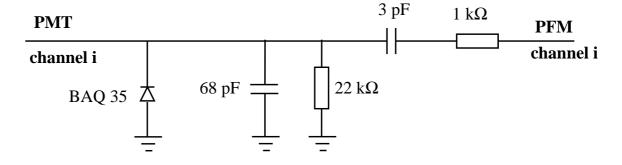
Figure 5.11: Capacitive Coupling Between PMTs and GASSIPLEX Input
