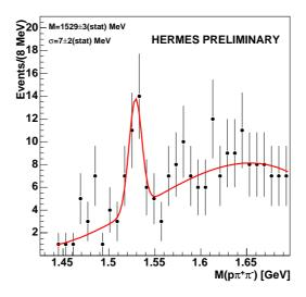
Figure 4.10: The invariant mass spectrum of  $K_S p$  system. Two opposite charged pions and protons are accompanied with the fourth track identified as pion. The events, where pion have together with  $K_S$  invariant mass of  $K^*$  or with p mass of the  $\Lambda$ , are excluded.
