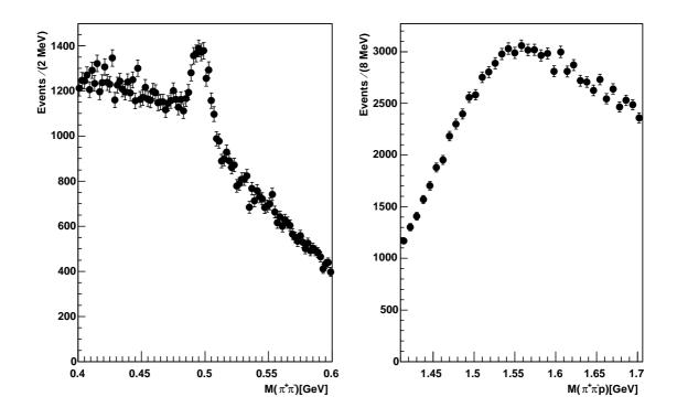
Figure 4.1:  $\pi^+\pi^-$  invariant mass spectrum (left) and  $\pi^+\pi^-p$  invariant mass spectrum (right). No cuts are applied on selected protons and pions. The  $\pi^+\pi^-$  spectrum shows clear  $K_S$  peak while no structure is seen in the  $\pi^+\pi^-p$  spectrum.
