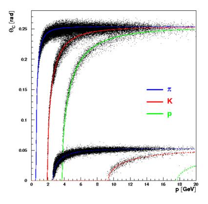
Figure 3.3: Čerenkov angles versus momentum for aerogel and  $C_4F_{10}$  gas. The upper curve shows angles of the Čerenkov light cone coming from the aerogel radiator. The lower curve corresponds to the  $C_4F_{10}$  gas.
