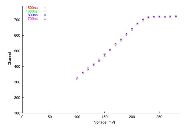
Figure 5.9: The result of the test of the PFMs response on the voltage of the input pulse.
