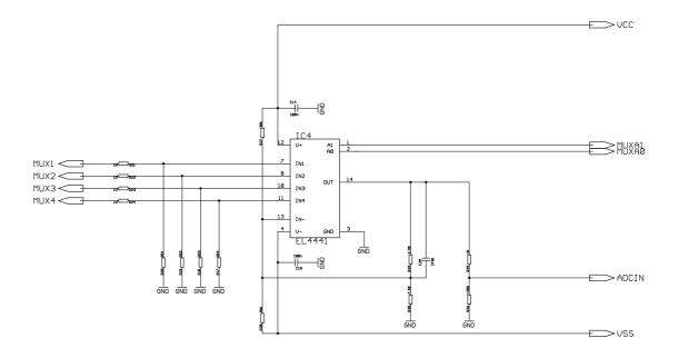
Figure 5.10: Analog Multiplexer Scheme
