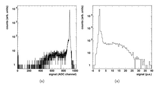
Figure 5.18: (a) Uncalibrated spectrum of a single SFT channel. On the lower ADC boundary the effect of erroneous overflow handling can be seen.(b) Spectrum of same SFT channel employing SPE calibration and including overflow suppression.
