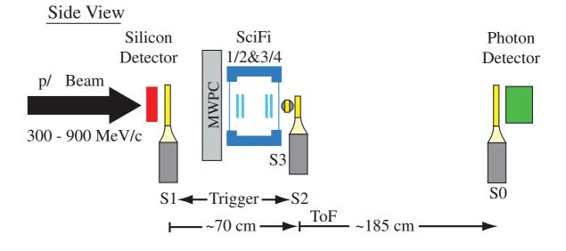
Figure 5.13: The side view of the experimental setup at the GSI in November 2003.
