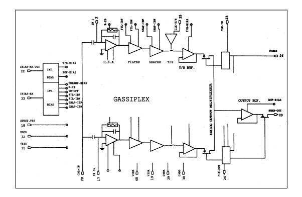
Figure 5.5: Scheme of internal structure of GASSIPLEX
