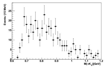
Figure 4.9: Invariant mass spectrum of the system  $K_S \pi$ . The spectrum is generated from events where three tracks of standard  $\Theta^+$  cuts are accompanied by fourth track which is identified as pion.
