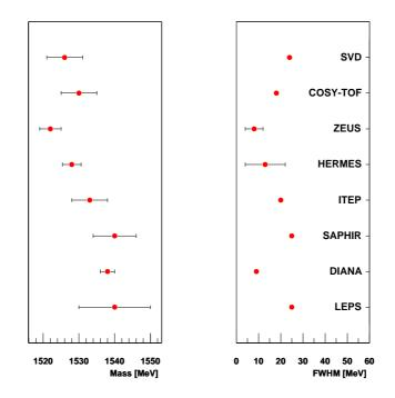
Figure 2.4: Compilation of the world data observed  $\Theta^+$ . Left panel shows the mass values and the right plot shows the FWHM.
