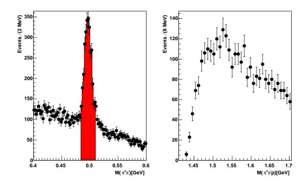
Figure 4.4: The  $\pi^+\pi^-$  invariant mass spectrum left and the  $\pi^+\pi^-p$  invariant mass spectrum right. The applied are extended by causality cut for position between  $\pi^+\pi^-$  production and decay vertex. The  $\pi^+\pi^-p$  spectrum is computed from events witch belong to the filled area of histogram in the left panel plot.
