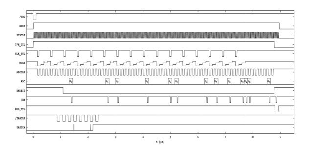
Figure 5.7: Timing of a complete sample cycle
