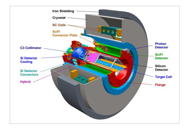
Figure 5.3: 3D View of the Recoil Detector
