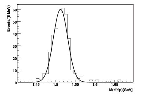
Figure 4.26: The  $pK_S$  system invariant mass spectrum obtained by simulation of  $\Xi^{*0}(1690)$  decaying into  $K_S^0\Lambda$ . The peak has been fitted by means of Gaussian distribution.
