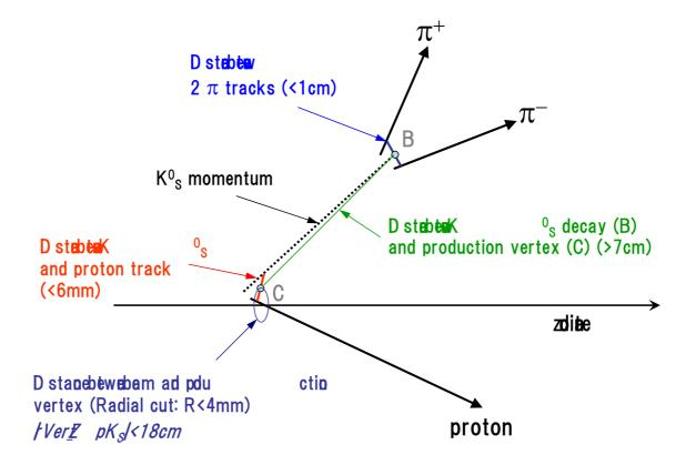
Figure 4.2: Topology of reconstructed three-track events
