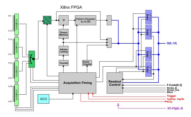
Figure 5.6: Block scheme of the PFM board
