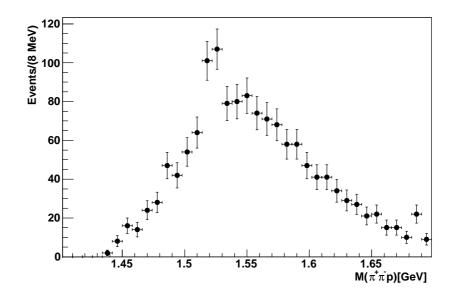
Figure 4.22: The reconstructed mass spectrum of  $pK_S$  system. The generated events are coming from decay of N(1710) decaying into  $K_S\Lambda$ . The  $\pi^-$  from the  $\Lambda$  decay is not reconstructed.
