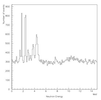
Figure 9.8.: This figure shows the theoretical spectrum of Auger neutrons from  ${}^{91}_{\Lambda}$ Zr, convoluted with the estimated experimental resolution and an additionally added background estimate (the figure was provided by A. Margarian [Margaryan04]). The p and f shell splitting is still clearly visible.
