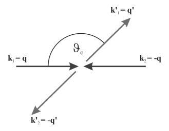
Figure 1.3.: Kinematics of the center of mass frame. The half off-shell scattering matrix depends only on four variables in that frame: the absolute values of the incoming and outgoing momenta  $|\mathbf{q}|$  and  $|\mathbf{q}'|$ , respectively, the scattering angle  $\vartheta_c$  and  $\sqrt{s}$ .
