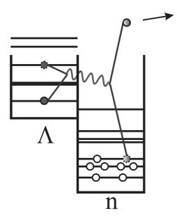
Figure 9.1.: Schematic picture of the hypernuclear Auger effect: A  $\Lambda$  hyperon is deexcited into a lower single particle level, thereby transferring energy and momentum to a valence neutron which is emitted through this process.
