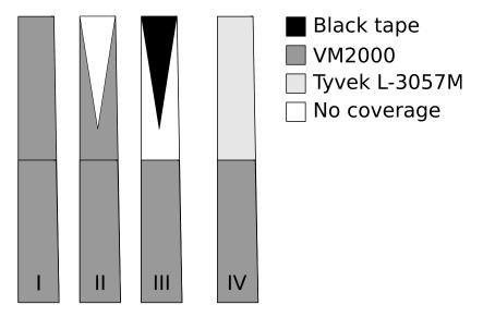
Figure 2.40: Schematical depiction of the wrapping modifications applied to crystal 458.
