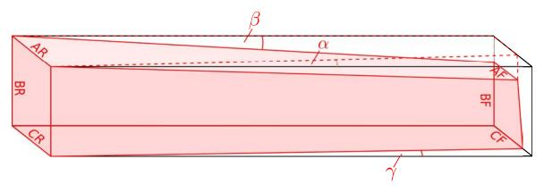
Figure 2.2: Definition of the three tapering angles  $\alpha$ ,  $\beta$ , and  $\gamma$  originating from the length difference of the sides AR - AF, BR - BF and CR - CF, respectively. For all crystal shapes the relations  $AX \perp BX$ ,  $BX \perp CX$  and  $AX \parallel CX$  are valid.
