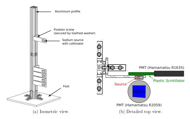
Figure 2.37: CAD of the high rate setup for NUF measurements.
