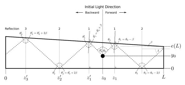
Figure 2.7: Schematic two dimensional view of a tapered crystal used to derive Eq. 2.3 to 2.11.
