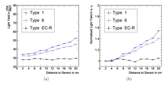
Figure 2.34: Measured LY response at -25 °C to 511 keV photons in dependence on the distance to the PMT in absolute values (a) and normalised to the position closest to PMT (b).
