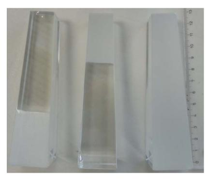
Figure 2.42: Three small crystals with a fully or partly emerised surface.
