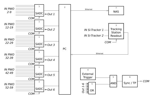
Figure 3.5: Schematic view of the prototype readout during the test beamtime at CERN SPS. For the individual module types, see Tab. 3.1.
