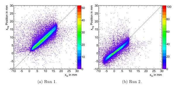
Figure 3.17: Position correlations in x-direction for both runs obtained with logarithmic weighting. The dashed line corresponds to a linear correlation of reference position  $x_{Si}$  and reconstructed position  $x_{log}$ .
