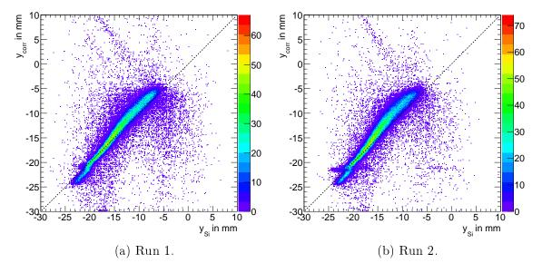
Figure 3.15: Corrected position correlation (S-curve) in y-direction for both runs, obtained with linear weighting. The dashed line corresponds to a linear correlation.
