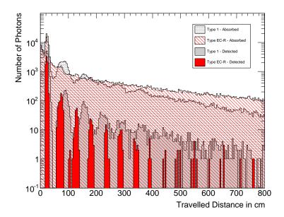
Figure 2.20: Comparison of the number of photons absorbed anywhere in the setup or detected by the PMT for type 1 and EC-R, if the source is at z = 18 cm.
