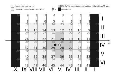
Figure 3.7: Scheme of the PROTO60 crystal matrix in beam direction. Grey italic numbers indicate the physical number of the crystals in the matrix, while black numbers are the crystal indices used in readout and analysis. The positron beam was either impinging on the centre of crystal 28 (run 1) or in between crystal 28 and 29, marked by an open and a filled circle, respectively. The schematics are not true to scale.
