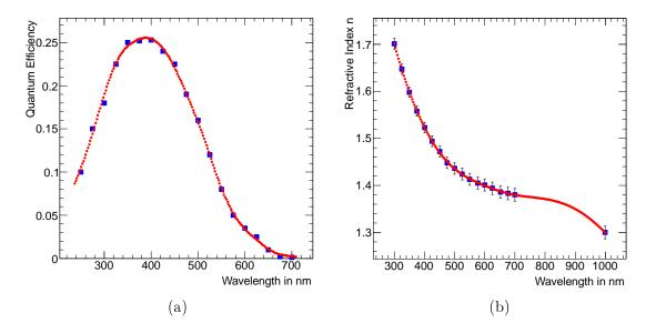
Figure 2.12: Spline fits for implementation of the optical properties of PMT quantum efficiency (a) and refractive index of the optical coupling material (b).
