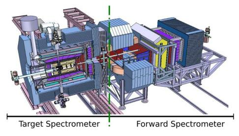
Figure 1.7: Layout of the  $\overline{P}ANDA$  Detector.
