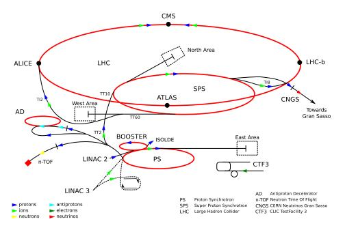
Figure 3.3: Schematic view of the CERN accelerator complex [40]. The experiment described in this work was performed at the H4 beamline located at the North Area. The primary proton beam provided by SPS was converted into secondary beams of either  $15 \frac{\text{GeV}}{c}$  momentum positrons or  $150 \frac{\text{GeV}}{c}$  momentum muons.
