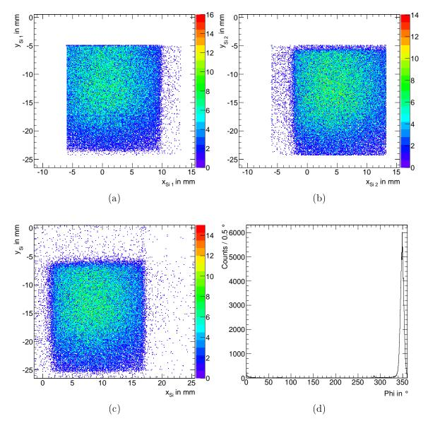
Figure 3.9: Beam spots during run 1 as measured by Si-tracker 1 (a) and Si-tracker 2 (b), respectively. In addition the position extrapolated to the PROTO60 front face is shown (c), which serves as reference position during analysis. For these pictures, the absolute calibration was performed as described in Sec. 3.4.3. In addition, the  $\varphi$  deviation of the particle trajectory, with respect to the symmetry axis of the tracking station is shown (c).
