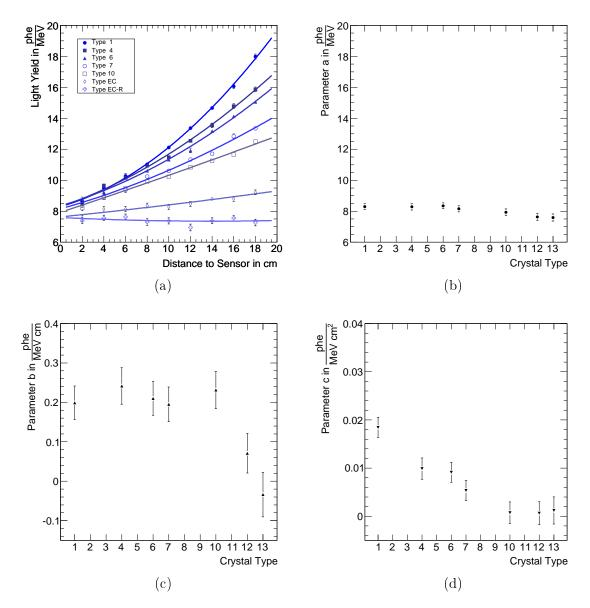
Figure 2.16: Simulated NUF for several types fitted with a second order polynomial (a). The extracted parameters a, b and c are shown in (b), (c) and (d), respectively.
