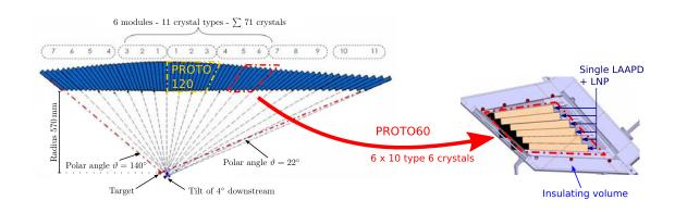
Figure 3.1: Schematic view of the Barrel EMC slice subsection represented by PROTO60, which is marked by the red box. The matrix, consisting of  $6 \times 10$  PWO-II crystals of type 6 geometry, is contained in an insulating volume for standalone operation. Each crystal is read out by a single LAAPD coupled to a Basel LNP. Additionally the section represented by the future prototype PROTO120 is marked in yellow.
