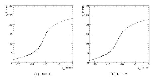
Figure 3.11: Fits to the raw y-direction S-curves obtained with linear weighting.
