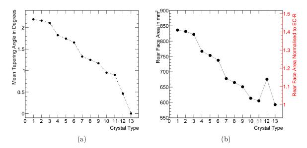
Figure 2.4: Mean tapering angle calculated according to Eq. 2.2 (a) and area of the rear face in  $mm^2$  and relatively to type EC-R (b).
