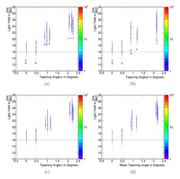
Figure 2.24: Correlations between LY and the tapering angles  $\alpha$  (a),  $\beta$  (b),  $\gamma$  (c) and mean tapering angle  $\mu$  (d). The LY specification limit is marked with a dashed line. A clear correlation of LY and tapering angle is visible.
