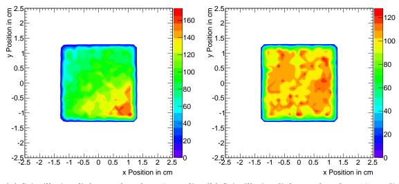
(a) Scintillation light produced at 2 cm dis (b) Scintillation light produced at 18 cm dis tance to photo sensor.
