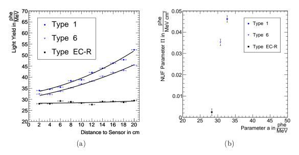
Figure 2.35: Measured LY response at  $-25 \,^{\circ}\text{C}$  to 511 keV photons in dependence on the distance to the PMT fitted by a second order polynomial (a). NUF parameter II in dependence of the constant LY contribution represented by parameter *a* (b).
