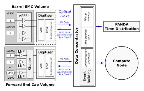
Figure 1.20: Schematic view of the EMC DAQ. The preamplified and shaped signals coming from individual detectors are sent to the Digitiser for digitisation. An on-board FPGA performs feature extraction and hit building. Hit data of several digitiser modules is then transmitted via optical links to the Data Concentrator where the EMC event building takes places. A processed event is then forwarded to the Compute Node where online event reconstruction with data from all subdetectors takes place.
