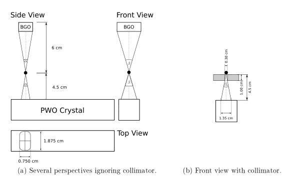
Figure 2.30: Schematic drawing illustrating the beam spot size determination.
