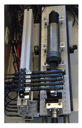
Figure 2.28: Photograph of the installed NUF measurement setup in cosmic ray configuration, contained in a large volume extension of the climate chamber. The upper array of five plastic scintillator detectors, mounted on an aluminium profile, is clearly visible. In the background, the crystal, covered with black shrinking tube and already attached to the PMT is shown. Below, the coupling of the sledge to the positioning gauge can be recognised.
