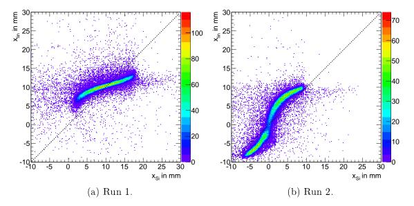
Figure 3.12: Non-linear position correlation (S-curve) in x-direction for both runs, obtained with linear weighting. The dashed line corresponds to a linear correlation.
