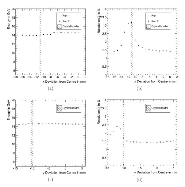
Figure 3.26: Dependence of cluster peak energy and relative energy resolution resolution in dependence of the deviation from the crystal centre. For cluster energy determination, a single crystal threshold of 1 MeV was used.
