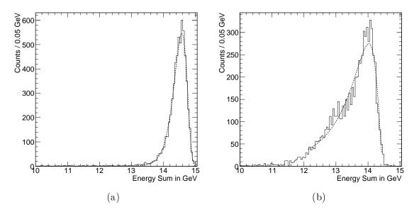
Figure 3.24: Typical line shape of the reconstructed cluster energy for a 15 GeV positron beam located either at the centre of crystal 28 (a) or at its border. In addition, the Novosibirsk function fit to extract cluster energy and resolution is drawn with a dashed line.
