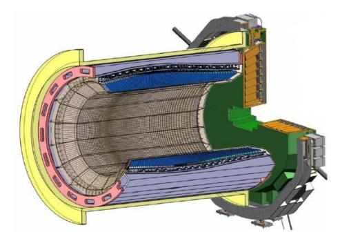
Figure 1.10: Layout of the electromagnetic calorimeter located in the Target Spectrometer.
