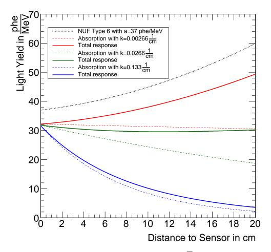
Figure 4.2: NUF parametrisation for a type 6 crystal of PANDA geometry taken from Tab. 2.7. The influence of distinct levels of additional absorption, representing different generations of PWO crystal quality, as observed during crystal production for the CMS-ECAL, is calculated according to Eq. 2.21 and plotted (coloured dashed lines). In addition, the obtained total response resulting from the combination of absorption and type 6 NUF curve is shown.
