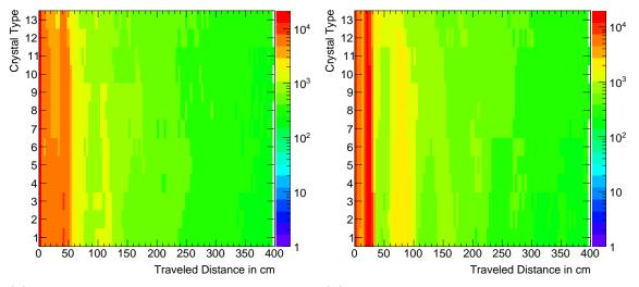
(a) Scintillation light produced at 2 cm dis (b) Scintillation light produced at 18 cm dis tance to photo sensor.
