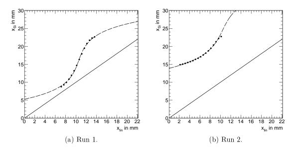
Figure 3.10: Fits to the raw *x*-direction S-curves obtained with linear weighting. For comparison, an ideal linear correlation is marked with a solid line.
