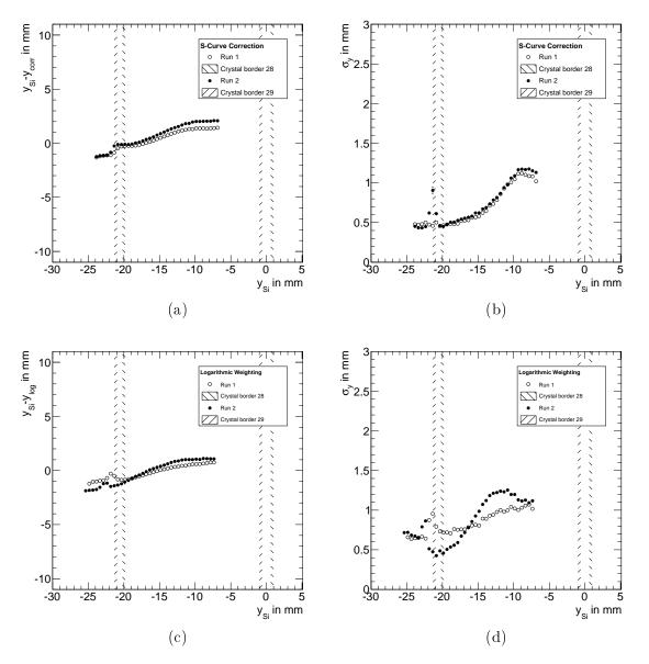
Figure 3.23: Dependence of y-position deviation and position resolution on the incident position obtained with the S-curve correction technique (a-b) and logarithmic weighting technique (c-d). The borders of crystal 28 and crystal 29, which are located at different heights y, are indicated by shaded areas.
