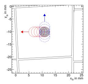
Figure 3.25: Restriction of the beam size to 4 mm diameter achieved by a cut on the reference position  $(x_{Si}, y_{Si})$  provided by the tracking station. Beginning at the centre of crystal 28, the beam centre was successively shifted in steps of 1 mm to the crystal borders, either in x- or y-direction.
