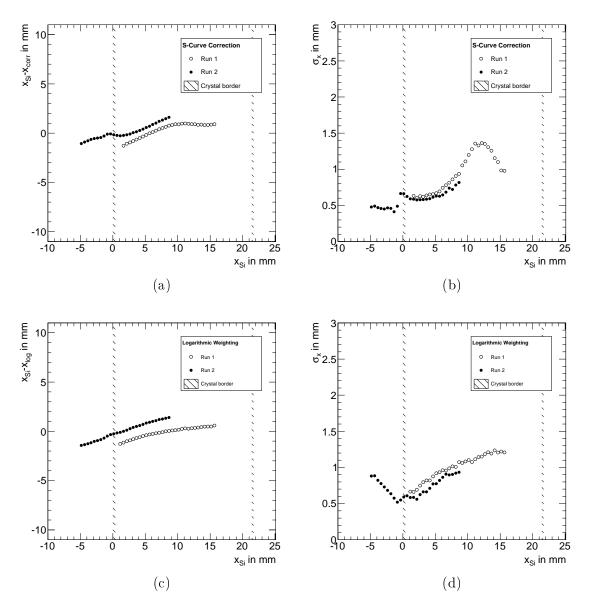
Figure 3.22: Dependence of x-position deviation and position resolution on the incident position obtained with the S-curve correction technique (a-b) and logarithmic weighting technique (c-d). Crystal borders are indicated by shaded areas.
