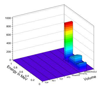
Figure 2.13: Energy deposited by the initial photon in different Volumes of the simulation setup.
