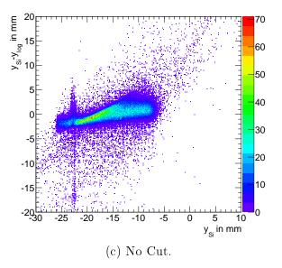
Figure 3.19: Position deviation  $y_{Si} - y_{log}$  in dependence of the reference position  $y_{Si}$  for three different conditions. Apparently, the two branches in (c) belong to the different cases of maximum energy deposition either inside crystal 28 or crystal 29, whose centre coordinates and borders are at different heights y.
