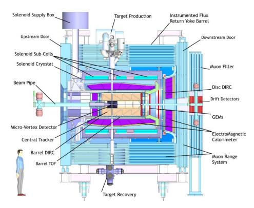
Figure 1.9: Layout of the  $\overline{P}ANDA$  Target Spectrometer.
