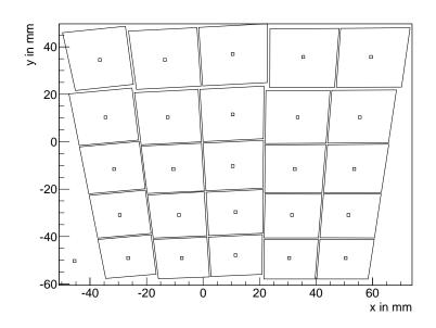
Figure 3.8: Crystal coordinates used in position reconstruction and front face projections of the 25 innermost crystals.
