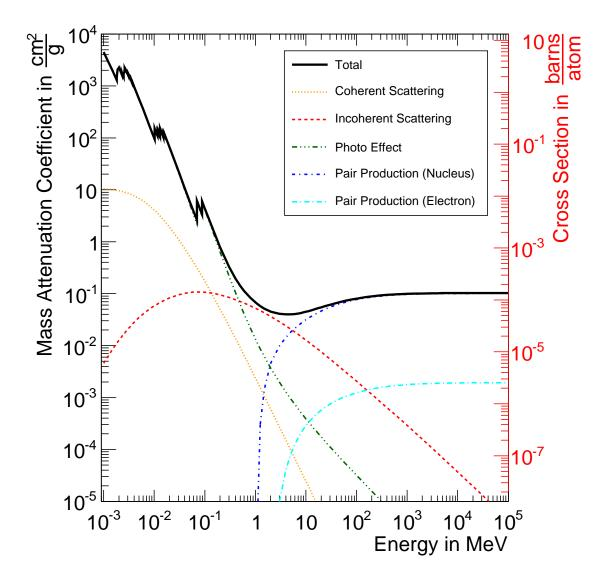
Figure 1.14: Mass Attenuation Coefficient of lead tungstate and corresponding photon absorption cross section as a function of the incident photon energy. Plotted data taken from [17].
