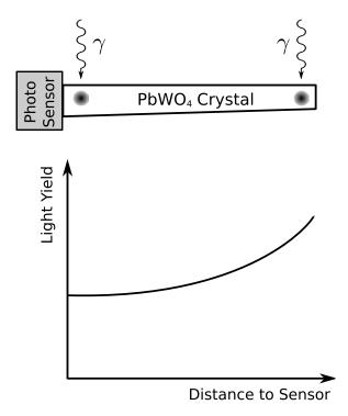
Figure 2.1: Schematic example for a case of light collection NUFs.
