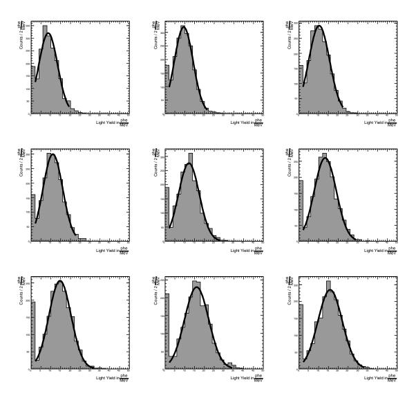
Figure 2.14: Light yield simulated for type 1 geometry at different distances from the photo sensor, fitted with a Gaussian function.
