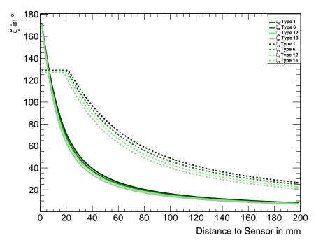
Figure 2.6: Opening Angles  $\zeta$  for scintillation light originating at distance z and reaching the photo sensor directly ( $\zeta_0$ ) or after one reflection ( $\zeta_1$ ). One recognises that for more tapered crystals  $\zeta$  becomes significantly larger. At low distances,  $\zeta_1$  is limited due to the threshold angle  $\theta_{thr}$  for total internal reflection.
