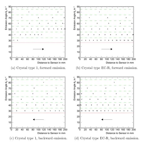
Figure 2.8: Reflection map of the two extreme crystal geometry types 1 and EC-R for forward and backward scintillation light emission under six different angles  $\theta_0$ . Displayed is the reflection number in the plane created by its distance to the sensor  $z_n$  and  $\theta_0$ . The red line indicates the threshold angle for total internal reflection, while the green lines separate the reflection sequences belonging to different  $\theta_0$ .
