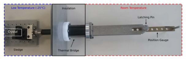
Figure 2.27: Detailed photograph of the sliding mechanism with positioning gauge.
