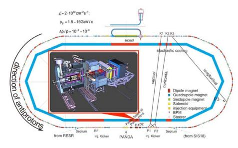
Figure 1.2: Schematic view of the HESR. The positions of electron cooler, stochastic cooling pickup (P1-P3) and kicker (K1-K3) as well as Rapid Frequency acceleration (RF) are indicated by red sections. The centre shows a schematic drawing of the PANDA detector [1].
