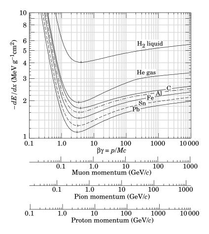
Figure 1.13: Energy loss due to collisions with atomic electrons in different absorber materials as a function of  $\beta\gamma$ . Additionally, the momentum for a muon, pion and proton is given [13].
