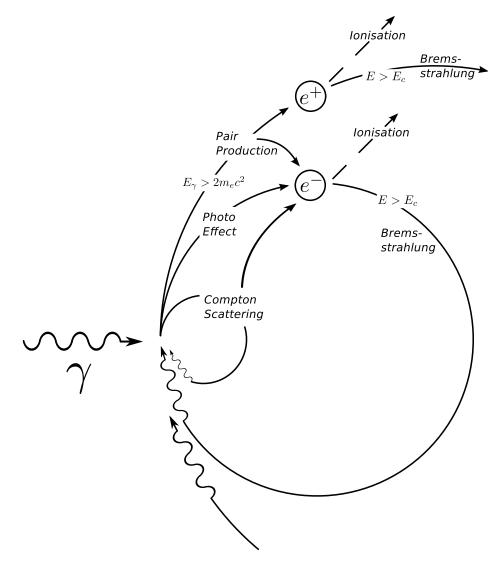
Figure 1.15: Schematic view of the development of an electromagnetic shower.
