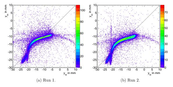
Figure 3.13: Non-linear position correlation (S-curve) in *y*-direction for both runs, obtained with linear weighting. The dashed line corresponds to a linear correlation.
