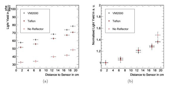
Figure 2.39: Light yield position dependence of crystal 647 (type 1L) for different wrappings in absolute values (a) and normalised to the position closest to the PMT (b).
