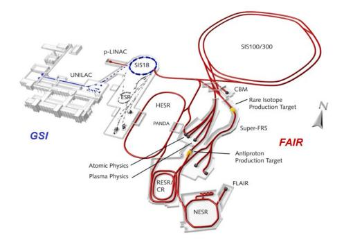
Figure 1.1: Artist's view of the planned FAIR facility (red) and the present GSI (blue). The PANDA detector is located in the centre of one straight section of the HESR.
