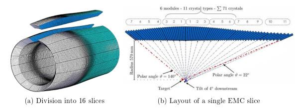
Figure 1.17: Crystal arrangement in the Barrel EMC.
