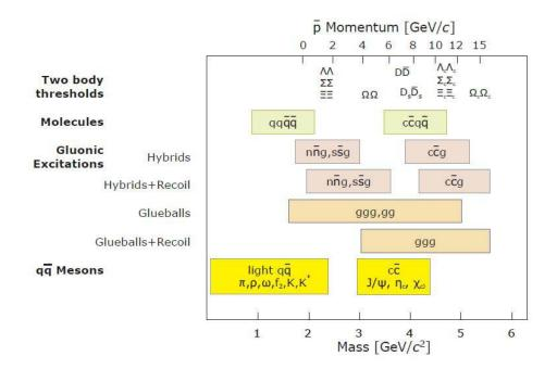
Figure 1.3: Invariant mass range (below) accessible to the PANDA experiment in comparison to the antiproton beam momentum (above). In Addition the producible particles and resonances are indicated.
