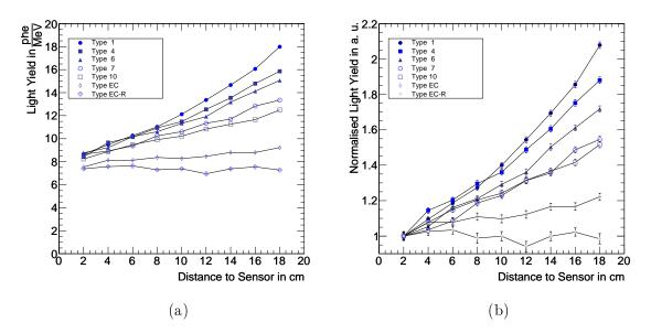
Figure 2.15: Simulated light yield for selected geometry types plotted in dependence of the distance of the  $\gamma$ -source to the PMT in absolute values (a) and normalised to the position closest to PMT (b).
