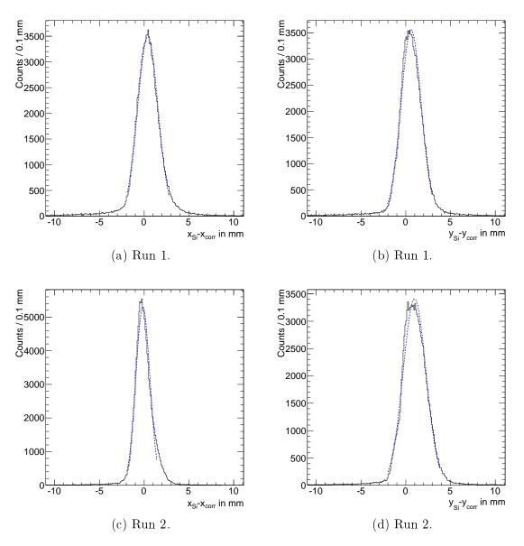
Figure 3.20: Overall position deviation distributions obtained with the S-curve correction technique. Mean and position resolution were determined by a Gaussian fit to the distributions (dashed blue line). The extracted parameters are collected in Tab. 3.5.
