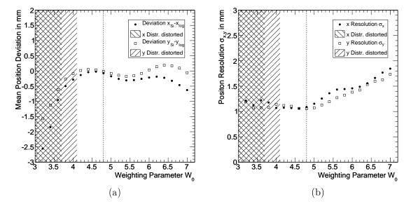
Figure 3.16: Deviation of the reconstructed positions  $x_{log}, y_{log}$  from the tracked positions  $x_{Si}, y_{Si}$  (a) and position resolution  $\sigma_x, \sigma_y$  (b) in dependence of the weighting parameter  $W_0$ . The shaded areas mark the regions, where the obtained position distributions are distorted. The weighting parameter value  $W_0 = 4.8$ , henceforth used for position reconstruction, is marked with a dashed line.
