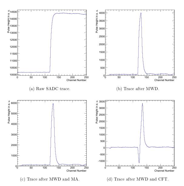
Figure 3.6: SADC traces of crystal 28 during the different steps of feature extraction. The final deposited energy for the selected event is derived from (c), while the time is extracted from (d).
