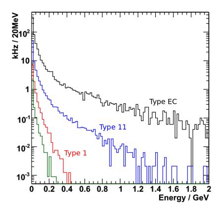
Figure 4.4: Single crystal energy differential rate spectrum expected for the PANDA EMC at 15 GeV/c incident beam momentum, in case of polar angles amounting to 5° (black), 25° (blue), 90° (red) and 135° (green)[21]. In addition, the crystal geometry types located at these angles are marked.
