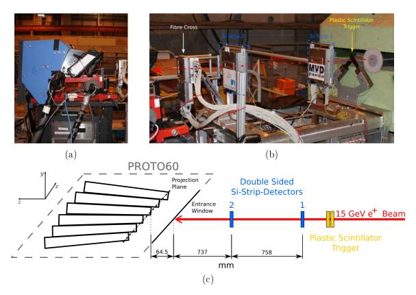
Figure 3.4: Photographs of PROTO60 (a) and tracking station during the test beam time at CERN SPS. In addition, the components and their respective distances essential for analysis are shown in a schematic view (c).
