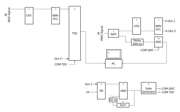
Figure 2.31: Precision setup readout scheme for 511 keV photon measurements. For the specific type of modules, compare to Tab. 2.6.
