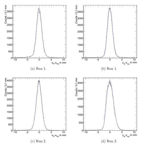
Figure 3.21: Overall position deviation distributions obtained with the logarithmic weighting technique. Mean and position resolution were determined by a Gaussian fit to the distributions(dashed blue line). The extracted parameters are collected in Tab. 3.5.
