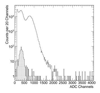
Figure 2.32: Energy deposition in the lead tungstate crystal without (unshaded) and with (shaded) a required coincident response of the BGO crystal within a time window of 8.5 ns. The selected spectrum was recorded for EC-R geometry at z = 10 cm distance to the PMT entrance window.
