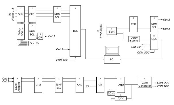
Figure 2.38: High rate setup readout scheme. For the specific type of modules, compare to Tab. 2.6.
