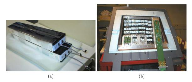
Figure 3.2: Photographs taken during the assembly of PROTO60. Crystals are wrapped with VM2000 and equipped with a single LAAPD and arranged in groups of four crystals (a). They are inserted through the opened backplane (b). From there also aluminium inserts, LNP and readout backplanes are mounted.
