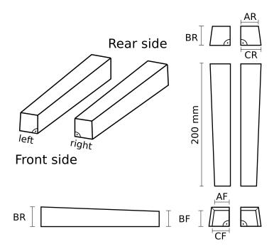
Figure 1.18: Drawing of the crystal geometry (from [21], slightly changed). The individual dimensions of the front face AF, BF, CF and the rear face AR, BR, CF are given in Tab. 1.5.
