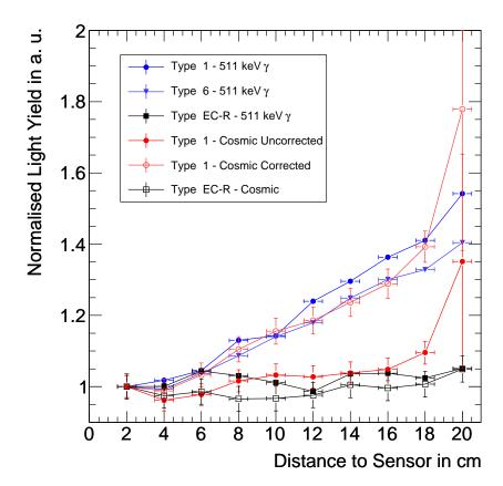
Figure 2.36: Comparison of the normalised response to cosmic muons and 511 keV photons, depending on the distance to the photo sensor.
