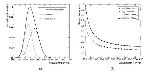
Figure 2.11: Input parameters for the SLitrani simulations. (a) Composition of the experimentally measured scintillation light spectrum out of two Gaussian distribution. (b) Plot of ordinary and extraordinary refractive index  $n_{ord}$  and  $n_{ext}$  given by [23]. Each is parametrised by an fit of the Sellmeier law for extrapolation over the whole wavelength range.
