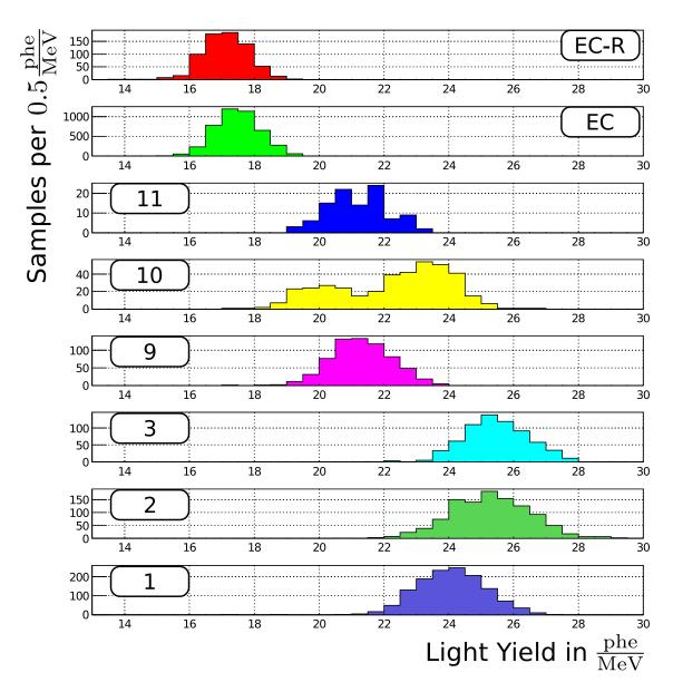
Figure 2.23: LY distributions measured relatively to a reference crystal by ACCOS [33] at CERN and calibrated to absolute values in units of  $\frac{\text{phe}}{\text{MeV}}$  at JLU Gießen [34]. The LY is displayed separately for each geometry. One recognises an increase of the average LY for more strongly tapered shapes.
