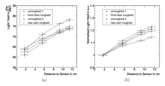
Figure 2.45: Light yield position dependence at  $-25 \,^{\circ}\text{C}$  of two small crystals before and after surface treatment in absolute values (a) and normalised to the position closest to the PMT (b).
