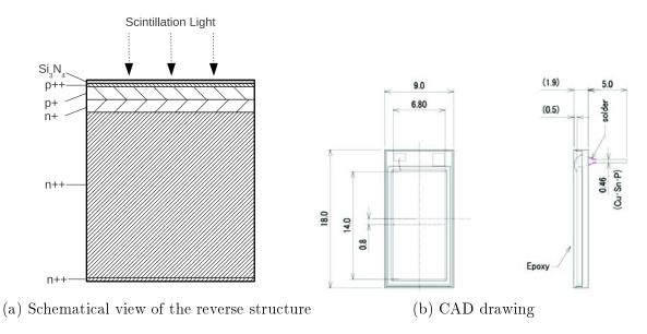
Figure 1.19: Layout of the rectangular  $\overline{P}ANDA$  LAAPDs.
