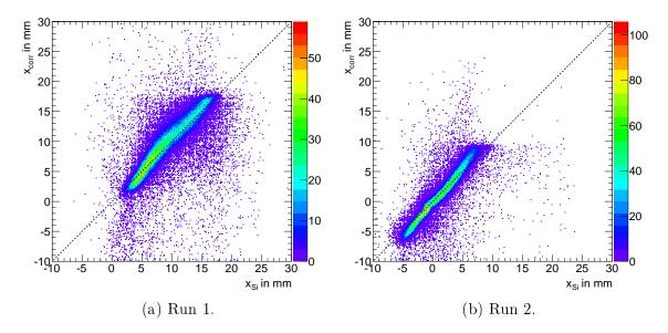
Figure 3.14: Corrected position correlation (S-curve) in x-direction for both runs, obtained with linear weighting. The dashed line corresponds to a linear correlation.
