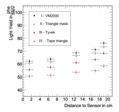
Figure 2.41: Light yield position dependence of crystal 458 (type 1L) for different wrapping modifications, as depicted in Fig 2.40.
