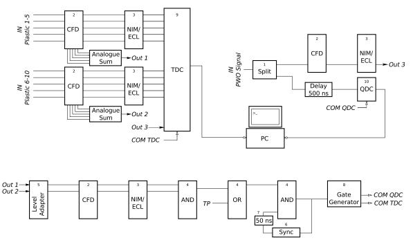
Figure 2.29: Precision setup readout scheme for cosmic measurements. The specific type of modules is listed in Tab. 2.6.
