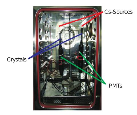
Figure 2.25: Measurement setup at JLU Gießen used for calibration of relative LY values provided by ACCOS at CERN [34].
