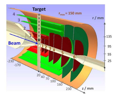
Figure 1.11: Proportionate schematics of the MVD, shown together with beam and target pipe. Red areas represent silicon hybrid pixel detectors, while the green areas indicate double-sided silicon strip detectors. The orange plane marks the inner radius of the central tracker [10].
