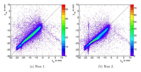
Figure 3.18: Position correlations in y-direction for both runs obtained with logarithmic weighting. The dashed line corresponds to a linear correlation of reference position  $y_{Si}$  and reconstructed position  $y_{log}$ .
