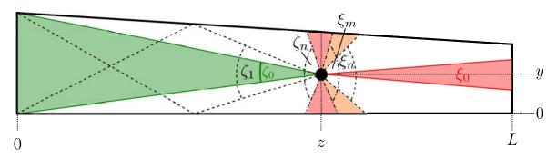
Figure 2.5: Opening angles  $\zeta$  and  $\xi$  for forward and backward scintillation light propagation, respectively. Green colour indicates that light emitted within this angular range is reaching the photo sensor, while red or orange colour represent that light is lost during propagation or not propagated there at all. In these considerations, only total internal reflection is taken into account.
