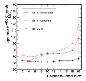
Figure 2.33: Position dependent response to minimum ionising cosmic muons at -25 °C for PWO-II crystals in type 1 and EC-R geometry. For the tapered shape, additionally the LY corrected for the most probable MIP energy deposition (see Tab. 1.3) for the corresponding pathlength e(z) is shown.
