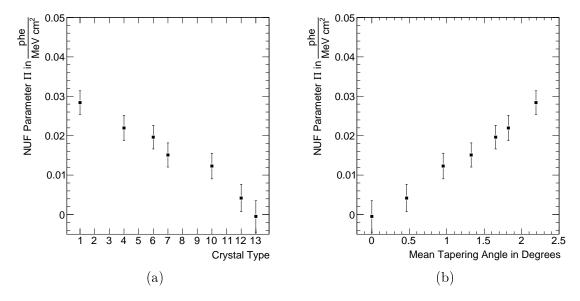
Figure 2.17: Non-uniformity parameter  $\Pi$  as obtained from fit to the simulated NUF curve for the selected crystal types (a) and in dependence of the mean tapering angle  $\mu$  (b).
