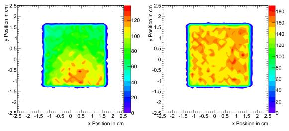
(a) Scintillation light produced at 2 cm dis- (b) Scintillation light produced at 18 cm distance to photo sensor. tance to photo sensor.
