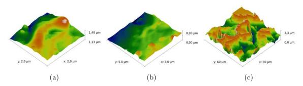
Figure 2.43: Height profiles of a small lead tungstate sample after surface treatment with emery paper. The area dimensions amount to  $2\,\mu\text{m} \times 2\,\mu\text{m}$  (a),  $5\,\mu\text{m} \times 5\,\mu\text{m}$  (b) and  $60\,\mu\text{m} \times 60\,\mu\text{m}$  (c).
