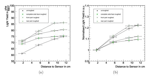
Figure 2.44: Light yield position dependence at  $-25 \,^{\circ}\text{C}$  of four small crystals with different roughed side face areas in absolute values (a) and normalised to the position closest to the PMT (b).
