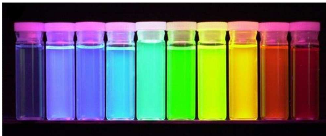
Figure 3.2: QDs display distinctive colors under UV excitation [165]. CdSe QDs of different sizes are excited with a near-UV lamp. Copyright 2001 Nature Publishing Group.
