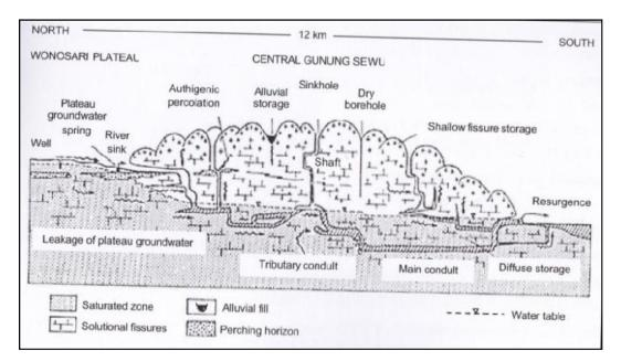
Figure 4.1. Cross-section of the Gunung Sewu Karst Underground (source: LUKAS, and STEINHILPER, 2005)
