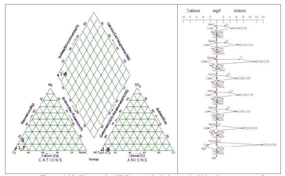
Figure 4.13. Piper and stiff diagram depicting typical bicarbonate water of Gunung Sewu Karst. Samples 1-4 are from surface rivers before sinking and samples 5–8 are from underground river (source: HARYONO, 2008b)
