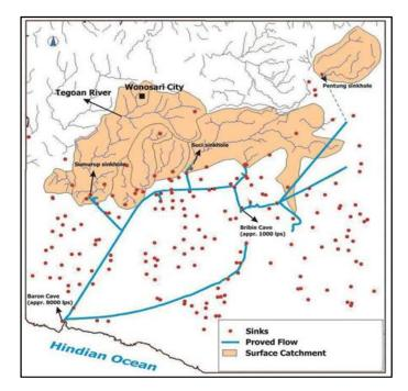
Figure 7.11. Possible recharge of Bribin-Baron Underground Water System with some sinkholes (source: ADJI and SUDARMADJI, 2008:3)
