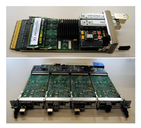
Fig. 6.7.: An AMC card equipped with 2 × 2GB DDR2 RAM, one SFP+ optical transceiver and one SFP+ transceiver for RJ45 cables (upper picture). The lower picture shows a aTCA carrier board fully equipped with four AMC cards.
