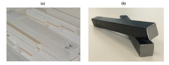
Fig. 4.7.: (a) A prototype PANDA EMC crystal cut into several smaller crystals. As can be seen, the smaller crystals easily break, therefore a bigger one (b) has been chosen for the prototype detector .
