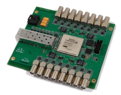
Fig. 6.4.: A picture of the sADC prototype developed by Pawel Marciniewski.
