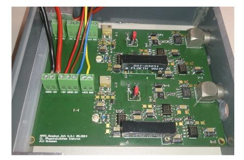
Fig. 6.3.: Picture of the produced 2-channel MPPC readout board, whose principal logic is shown in Fig. 6.2, the elongated black components are the analogue delays.
