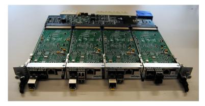
Figure 3.2.: Prototype of AdvancedTCA carrier board equipped with 4 xFP. [59]
