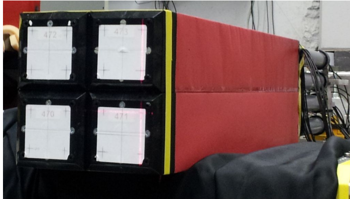
Figure 2.14: Picture of the new shashlyk EMC prototype tested in 2014 with 2 \times 2 modules ( 4 \times 4 cells) of type B.
