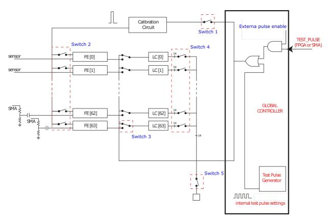
Figure 5.14: Schematic of the all possible test configurations in PASTA.
