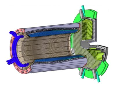
Figure 1.21: Layout of the Electromagnetic Calorimeter [56].
