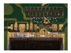
Figure 5.2: Picture of the PASTA wire bonded to the PB with  $17 \, \mu m$  diameter wires[85].
