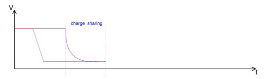
Figure 2.14: Voltage value for the  $C_{TAC}$  (red) and for the  $C_{TDC}$  (violet), after a certain time the two voltage value are equal.
