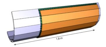
Figure 1.20: Layout of the Scintillating Tiles detector [54].
