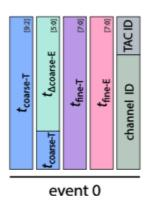
Figure 2.22: Full event mode, useful during the test phase. All the signals coming form the local controller are directly send out with any modifications.
