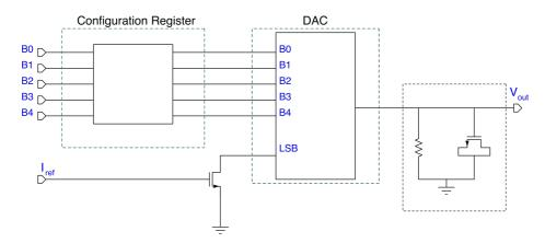
Figure 2.25: General PASTA bias cell schematic made by three structures. A configuration register necessary to buffer the configuration signals coming from the digital part, a DAC that set the needed current that has to be sent to the third group which can vary cell by cell.
