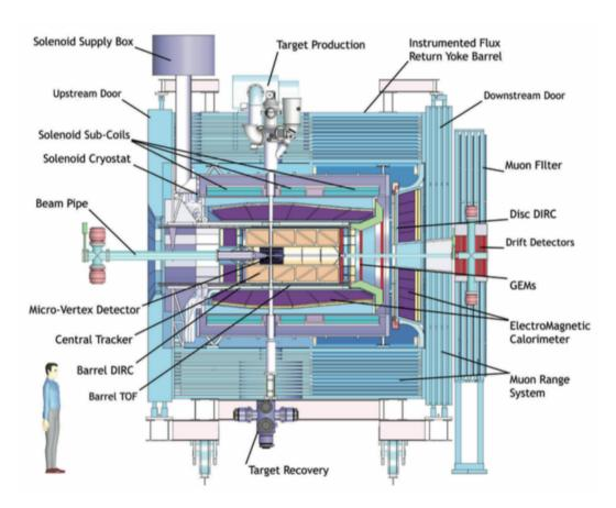
Figure 1.14: Layout of the Target Spectrometer.
