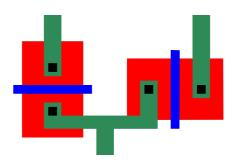
Figure 4.6: General differential input stage.
