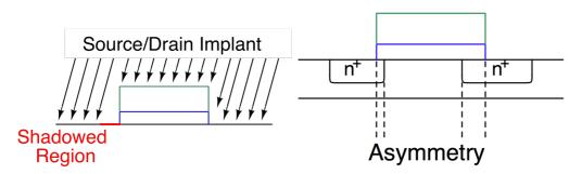
Figure 4.10: Representation of the gate shadow effect.
