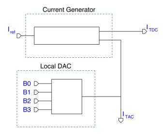
Figure 3.17: Structure needed to have the ratio 32 between the two currents and to tune the current  $I_{TAC}$ .
