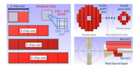
Figure 1.35: Pixel modules used to build disks and barrels [45].
