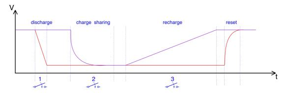
Figure 2.17: Complete process for the TDC, in red is reported the voltage value on the capacitor  $C_{TAC}$  while in violet on the capacitor  $C_{TDC}$ .
