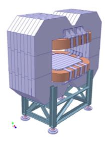
Figure 1.27: Layout of the dipole magnet [58].
