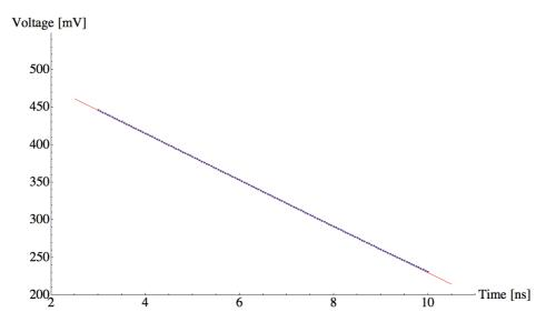
Figure 3.22: Voltage values reached by the folded cascode amplifier for different times (simulations, blue) and best fit to the points (red).
