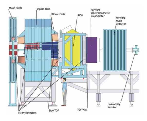
Figure 1.25: Layout of the Forward Spectrometer [58].
