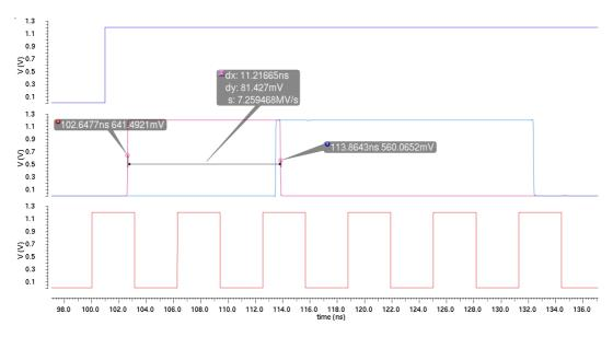
Figure 3.32: Combined simulation of both the local controller and the TDC. The blue signal in the first graph is the DOT, in the second graph the light blue represents the coarse time, the magenta signal is the fine time while the third graph shows the main clock.
