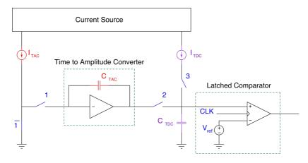
Figure 2.11: Representation of the switch positioning at the TDC starting phase.
