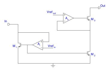
Figure 3.4: Current buffer architecture
