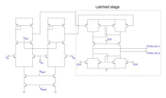
Figure 3.29: Schematic of the latched comparator.
