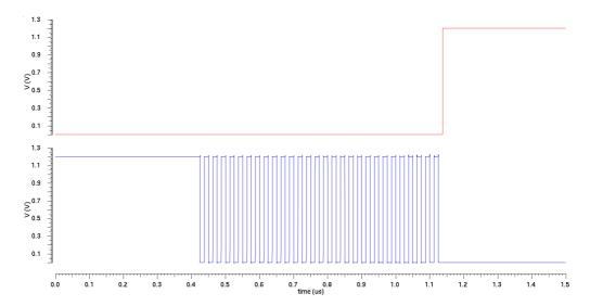
Figure 3.31: Output of the latched comparator using a selective clock.
