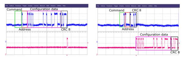
Figure 5.13: The left picture shows the SDI (blue) and the SDO (magenta) when the command "Write channel configuration" is sent to the chip. In the right picture the SDI and SDO are shown when the command "Read channel configuration" is sent.
