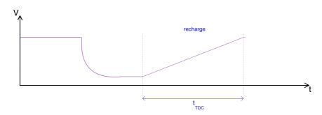
Figure 2.16: Voltage level of  $C_{TDC}$  during the recharging process.
