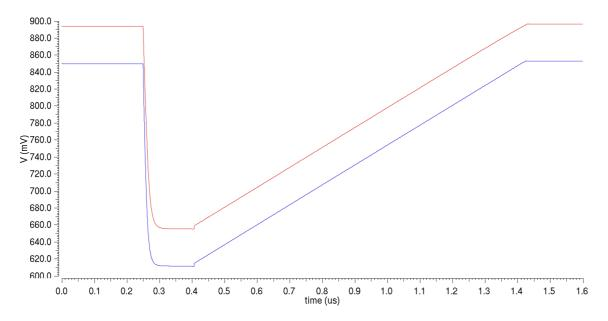
Figure 4.14: Simulated effect of the parasitic resistors between each channel on  $V_{ref}$ . The voltage value on the capacitor  $C_{TDC}$  in the channel "0" (blue) and in the channel "63" (red) are shown. It can be seen that in the last channel the recharging phase is shorter with respect to the first channel.
