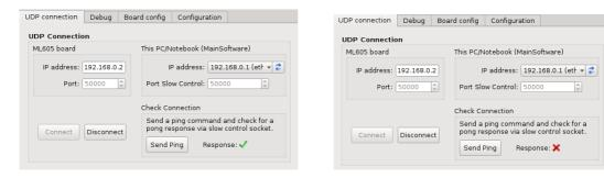
Figure 5.8: Connection interface in the JDRS. In the figure on the left the connection was successful since the response mark is green while on the right figure the mark is red meaning that the connection has failed.
