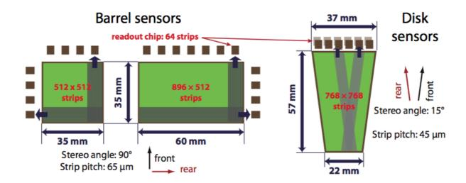
Figure 1.38: Layout of the three different shapes of strip sensors [69].
