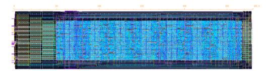
Figure 4.13: Layout of the local controller on which, in the left, there are the metal lines needed for the connections between the analog part of the channel and the local controller.
