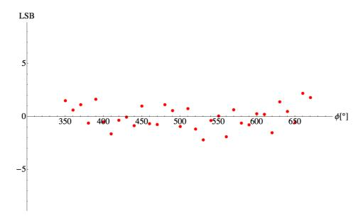
Figure 5.17: Results of the non-linearity of the Wilkinson ADC implemented in the TDC
