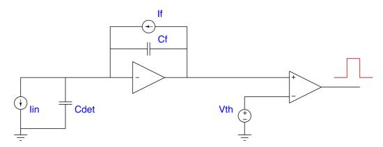
Figure 2.7: General Front End based on a ToT measurement, composed by an amplifier and a comparator.
