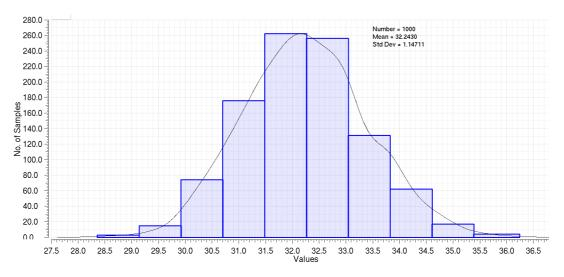
Figure 3.20: Distribution of the ratio of the currents  $I_{TAC}/I_{TDC}$  for the new current source.
