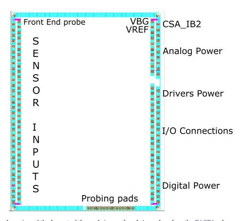
Figure 4.16: Final version of the layout of the pad ring and seal ring, placed on the PASTA edge.
