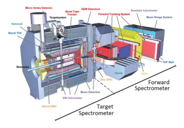
Figure 1.13: Overview of the whole  $\overline{P}ANDA$  experiment.
