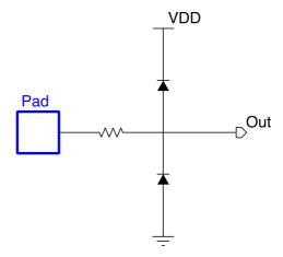
Figure 4.15: Schematic of a simple ESD protection needed by the pads.
