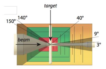
Figure 1.33: Geometrical layout of the MVD [69].
