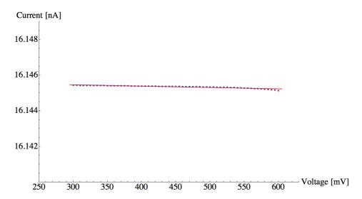
Figure 3.18: Trend current  $I_{TAC}$  (blue points) in the expected working region for the new current source.
