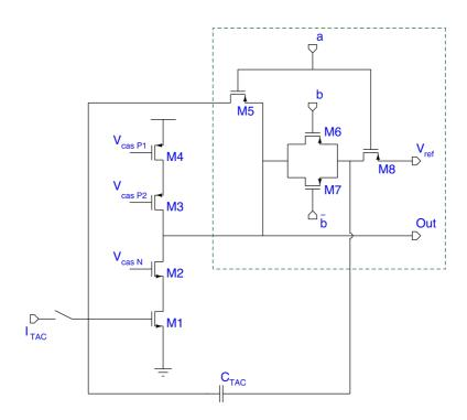
Figure 3.25: Schematic of cascoded amplifier.
