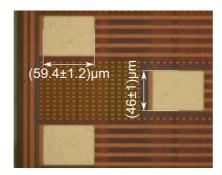
Figure 5.1: High resolution photo of the pads of the chip. The picture is obtained using a microscope [85].
