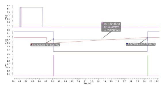
Figure 3.33: The first graph shows the DOT and the coarse time. In the second graph there is the voltage value on the capacitor  $C_{TDC}$  in red while the blue signal is the output of the latched comparator. In the third graph the digital signal SOC can be seen in magenta and the EOC in green.
