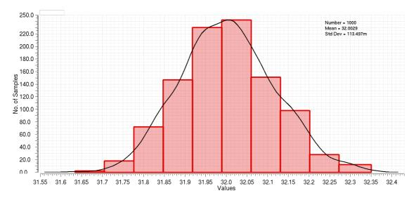
Figure 3.15: Distribution of the ratio of the current  $I_{TAC}/I_{TDC}$  due to the process variations.
