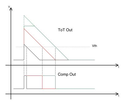
Figure 2.8: In the upper part there is the output signal of the ToT stage while in the lower graph is represented how the ToT is performed. Notice that the output of the comparator is proportional only to the length of the signals.
