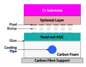
Figure 1.34: Cross-section of the hybrid pixel detector[45].
