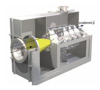
Figure 1.31: Layout of the luminosity detector [67].
