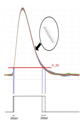
Figure 2.1: Different thresholds problems. In one case the jitter on the trailing edge is much bigger than the second case where the threshold is higher but the time stamp is less precise.
