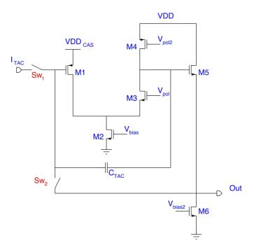
Figure 3.21: Schematic of a folded cascoded amplifier.
