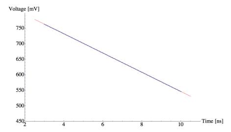
Figure 3.26: Different voltage value reached by the cascode amplifier for different duration of the discharging phase.
