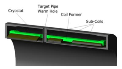
Figure 1.23: Section view of the Solenoid magnet [58].
