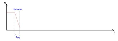
Figure 2.13: Voltage level of  $C_{TAC}$  during the discharging phase.
