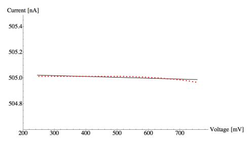
Figure 3.19: Best fit of the  $I_{TDC}$  current.
