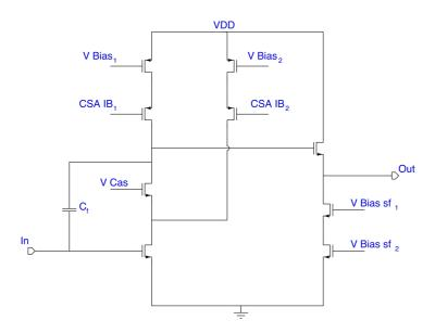
Figure 3.2: Architecture of the CSA implemented in PASTA.
