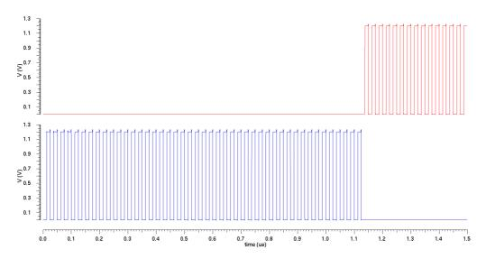
Figure 3.30: Output of the latched comparator (red the positive one, blue the negative one).
