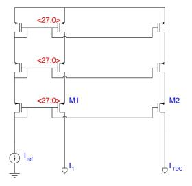
Figure 3.16: Schematic of the new current source based on the old structure.
