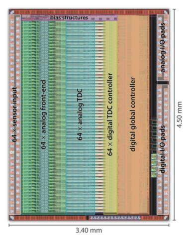
Figure 2.5: The several structures that compose the PASTA chip [80].
