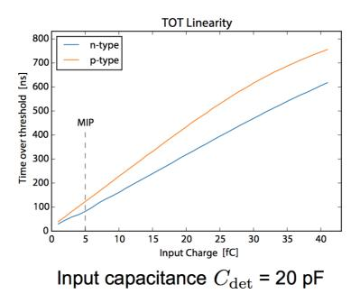
Figure 3.10: Different time duration of the output signal of the Front End chain for different input charge. It shows the expected linearity of the Front End [80].
