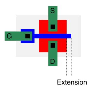
Figure 4.2: Polysilicon line (blue) that exceeds the active area (red).
