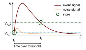
Figure 2.2: In PASTA the ToT is performed using two different threshold: one close to the base line to give a precise time stamp and the other as higher as possible to reduce the jitter in the falling edge of the signal and to be less sensible to the noise [80].
