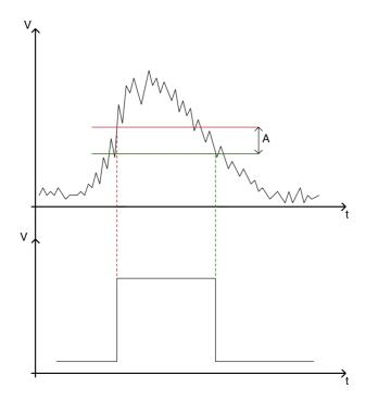
Figure 3.9: The upper graph shows the hypothetical input of the hysteresis comparator, while the lower one is the corresponding output. Notice that, even if the signal crosses every single threshold more than once the output is not effected by multiple firing.
