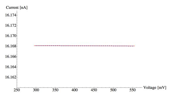
Figure 3.13: In blue the  $I_{TAC}$  current values for several voltage values are shown. The voltage range is the expected working region of the  $I_{TAC}$  branch. The red line is the best fit for the points.
