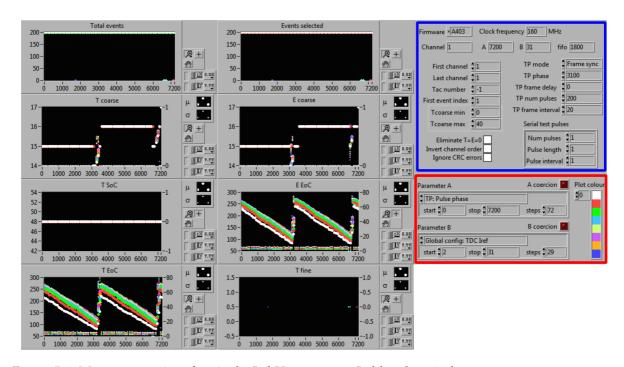
Figure 5.6: Measurement interface in the LabView system. In blue there is the measurement parameters region, in red is the region where the variables that are to be scanned are defined.
