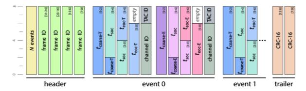
Figure 2.24: Example of a complete output frame in PASTA in the Full event mode [78].
