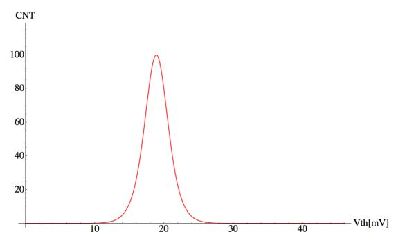
Figure 5.19: Derivative function of the threshold scan with an optimised Front-End:  $\mu$ =18.88 mV,  $\sigma$ =1.80 mV.
