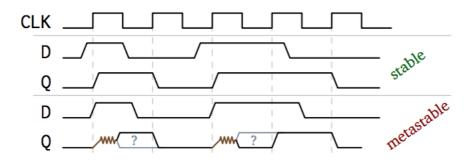
Figure 2.18: Representation of a Flip-Flop output in two cases: in first one the input is sufficiently far form the leading edge of the clock while in the second one is contemporaneous leading to an output that is metastable [78].
