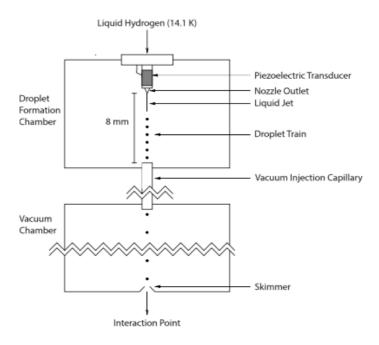
Figure 1.12: Schematic for the pellet target system developed for  $\overline{P}ANDA$  [46].
