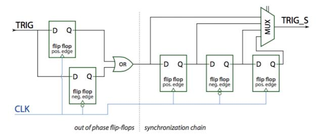
Figure 2.19: The first part is necessary to be sure to don't lose any asynchronous event while the second block is the structure implemented to avoid the metastability [83].
