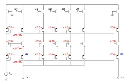
Figure 3.12: Schematic of a double cascoded current source with three branches: reference branch,  $I_{TAC}$  branch and  $I_{TDC}$  branch. The structure in the middle is a DAC used to tune the current  $I_{TAC}$ .
