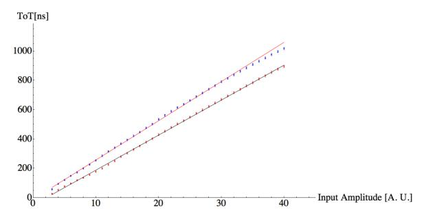
Figure 5.20: The blue (red) dots represent the ToT obtained as difference between "E coarse time" and "T coarse time", in the case of p-type (n-type) strips, as a function of several input amplitudes of the test pulse. The red (black) line is the best fit of the data. The last five points of p-type configuration are not taken into account for the linear fit because there is a compression of the points for high charges.
