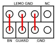
Figure 5.4: Pin header connections to select the biasing of the sensor. The LEMO GND is the ground of the HV used to bias the sensor. It is connected with the n-bulk of the sensor (BN) to the guard ring of the sensor (GUARD) and to the ground of the board (GND).
