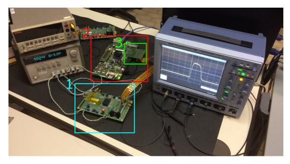
Figure 5.12: Photo of the laboratory setup used during the tests of PASTA. The DISH (azure box), the evaluation board (red box) and the breakout board (green box)
