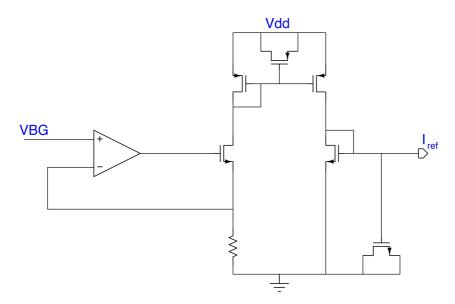
Figure 2.29: Structure that use an external voltage VBG to produce a very stable  $I_{ref}$  that is the current used from all the DACs in all the biasing cells.
