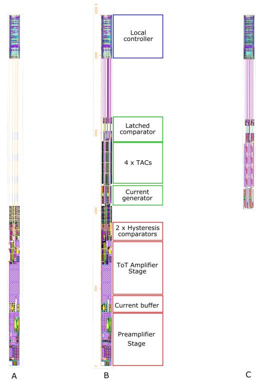
Figure 4.11: In figure B is shown the complete channel layout. The layout of the Front End with the connections to the local controller is shown in Figure A while the TDC and it connections to the local controller is shown in Figure C.
