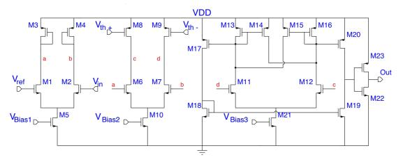
Figure 3.8: Schematic of the hysteresis comparator.
