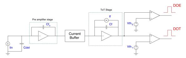
Figure 2.9: Schematic of the Front End chain used in PASTA, made by three stages and the comparators where the two different thresholds are applied.
