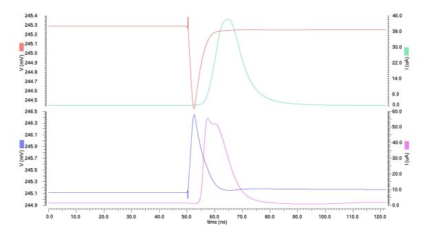
Figure 3.3: The blue line represents the voltage at the input of the preamplifier when a n-strip is connected, while the violet line shows its output current. The voltage signal in red is the input when a p-strip is connected to the preamplifier and the output is represented in green. Notice that the outputs have the same polarity.
