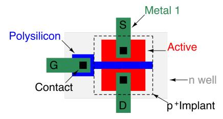
Figure 4.1: Layout of a p-mos transistor.
