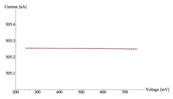
Figure 3.14: The different values of  $I_{TDC}$ , in the working region of its branch, are represented by blue dots. The best fit to the points is shown in red
