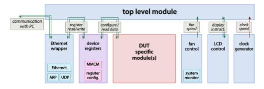
Figure 5.7: Block diagram of the firmware used in the JDRS. The modular structure allows to change only the part of the DUT to test a new ASIC [78].
