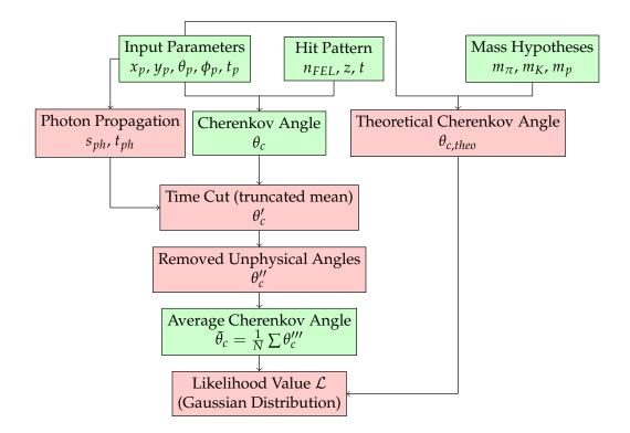
Figure 6.1.: The flow diagram of the online reconstruction algorithm.
