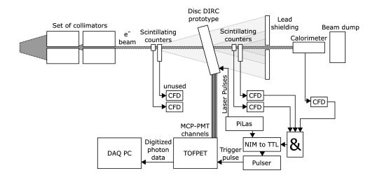
Figure 7.2.: The Disc DIRC prototype setup used for the DESY 2016 testbeam
