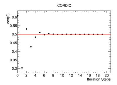
Figure 6.6.: The computed cosine angle with the CORDIC algorithm as a function of the iteration steps. The red line indicates the real value.
