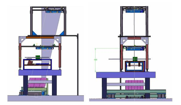
Figure 5.5.: The CAD drawing of the cosmics test stand upgrade with the view into the y-z (left) and x-z (right) plane.
