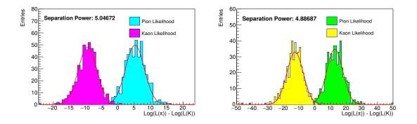
Figure 6.2.: A comparison between the online and offline reconstruction algorithms.
