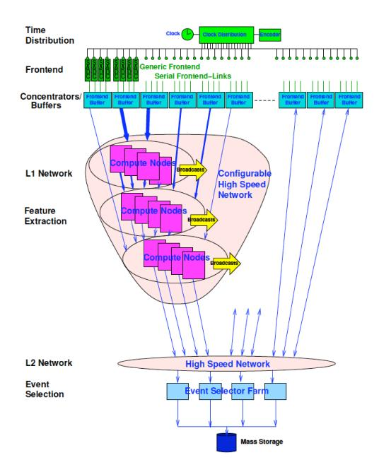
Figure 2.8.: The simplified schematics of the PANDA DAQ system [Wag16]. The hits taken by the FEE are processed to the data concentrators and then sent to Compute Codes, where the online reconstruction is taking place. After the event selection the accepted events are then stored for the offline analysis.
