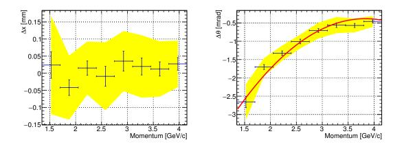
Figure 4.6.: The *x*-position (left) and polar angle (right) resolution of the reconstructed particle track for  $\pi^+$  particles as a function of the particle momentum. The error bars indicate the error of the mean value, and the yellow band represents the resolution.
