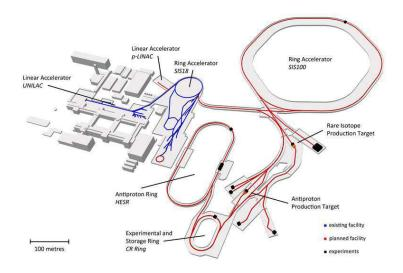
Figure 2.1.: A sketch of the Facility for Antiproton and Ion Research. The PANDA spectrometer is placed in the HESR storage ring for antiprotons which are produced with the antiproton target and cooled in the CR. The existing facility of the GSI is colored in blue while the red lines indicate the planned facility.
