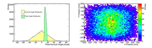
Figure 5.6.: The angular (left) and spatial acceptance (right) range of the cosmics test stand.
