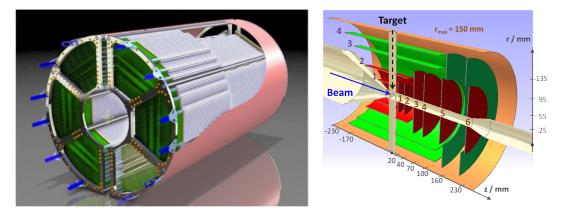
Figure 2.3.: 3D drawings of the tracking subdetectors STT (left) and MVD (right) in the PANDA Target Spectrometer.
