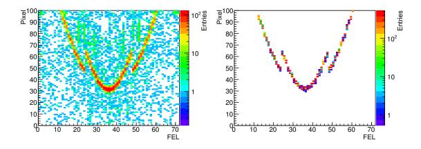
Figure 3.7.: Simulated (left) and reconstructed (right) hit pattern for  $\pi^{\pm}$  and  $K^{\pm}$  for a momentum of p = 4 GeV/c.
