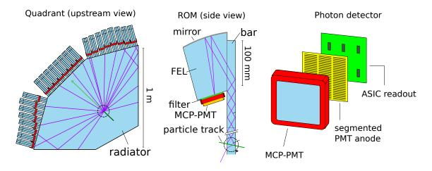
Figure 3.1.: A sketch of one quadrant of the EDD detector including the 24 ROM (left), a sensor element with the bar and FEL (center), and an exploded drawing of the proposed MCP-PMT with the segmented anode and ASIC readout (right).
