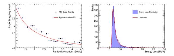
Figure 4.3.: The simulated results of angular straggling of  $\pi^+$  traversing through a fused silica volume with a thickness of 2 cm (left) and the energy loss distribution for  $\pi^+$  with a momentum of p = 4 GeV/c (right).
