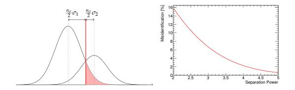
Figure 3.8.: Definition of the separation power between two probability density functions (left) and the calculated misidentification as a function of the separation power (right)
