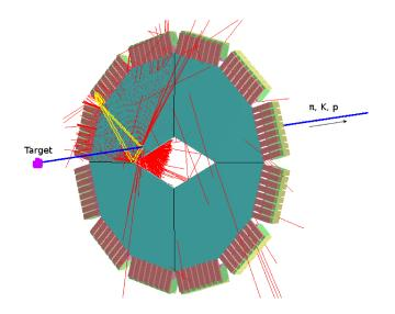
Figure 4.2.: The PandaRoot event display showing the Disc DIRC detector with a charged  $\pi^+$  creating Cherenkov light inside the radiator.
