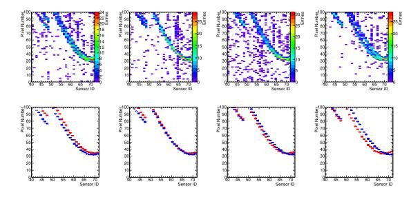
Figure 4.14.: The simulated (up) and reconstructed (down) hit pattern for different azimuth angles regarding the high resolution scan. The four columns show the hit pattern for different positions of the  $\pi^+$  on the radiator plate.
