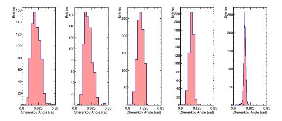
Figure 7.11.: The evolution of the testbeam result for validating the simulation results of one detector quadrant in PANDA starting from the testbeam setup with electrons (left) and reaching to the detector resolution of the final EDD in PANDA (right).
