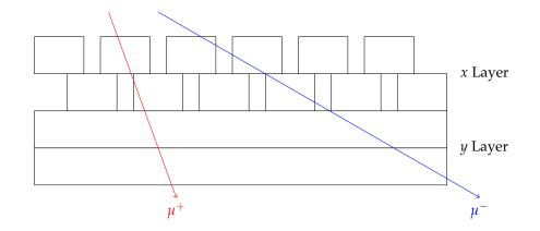
Figure 5.3.: A sketch of the cosmics test stand upgrade using 4 layers of scintillation bars with a pitch of 1/3 of the bar width.
