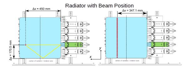
Figure 7.3.: The prototype setup used in the testbeam at DESY with sample beam positions indicated by red circles for the performed angle scan (left) and the *y* axis scan (right) including yellow lines as two possible photon paths.
