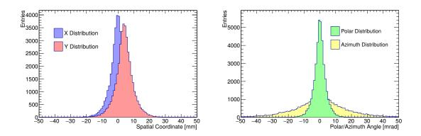
Figure 5.7.: The spatial (left) and polar/azimuth angle (right) resolution of the cosmics test stand.
