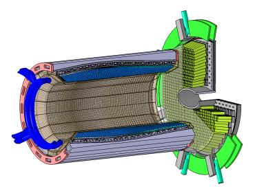
Figure 2.5.: The EMC for PANDA in the TS excluding the backward part. The parts related to the endcap part are colored green and the material of the barrel part is indicated with blue color. The PWO crystals and the supporting frame are also shown.
