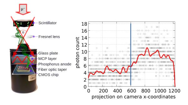
Figure 5.12.: The sketch of the setup with a single photon camera (left) and a plot of measured photon hits with a scintillator (right).
