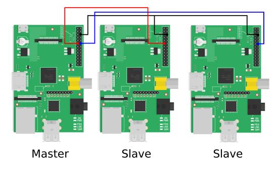
Figure 5.10.: The GPIO network between Raspberry PIs for coincidence measurement.
