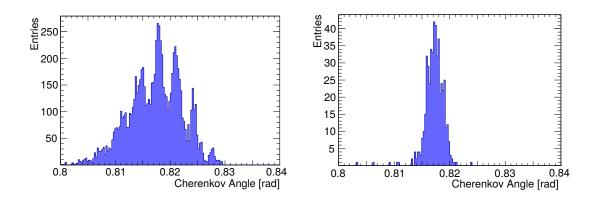
Figure 4.9.: Single photon distribution of the EDD for  $\pi^+$  particles with the momentum p = 4 GeV/c.
