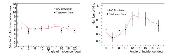
Figure 7.8.: Comparison of the single photon resolution (left) and photon yield (right) between testbeam data and Monte-Carlo simulations
