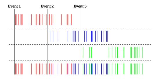
Figure 4.7.: The working principle of time-based simulations. The start time of each event is obtained from the Monte-Carlo simulations. Every row contains the hits related to one specific event which is indicated by a unique color. In the last row the sum of all hits shows the overlap of all detector hits.
