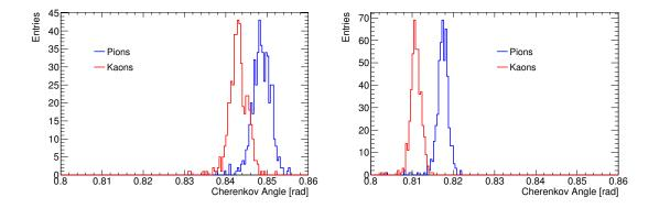
Figure 6.7.: The distribution of the reconstructed Cherenkov angle for 8 bit (left) and 16 bit (right) integer resolution.
