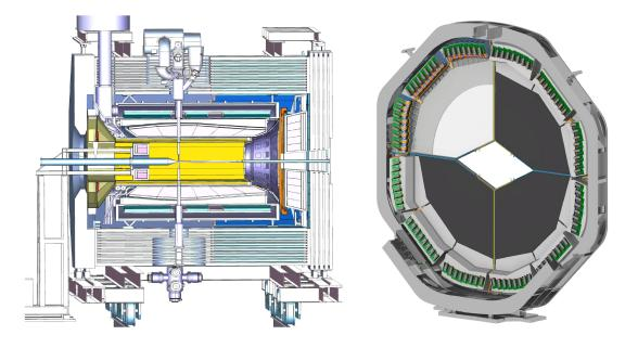
Figure 3.2.: A closer look at the target spectrometer with the EDD marked orange and Barrel DIRC marked yellow (left) and a CAD drawing of the assembled EDD (right).
