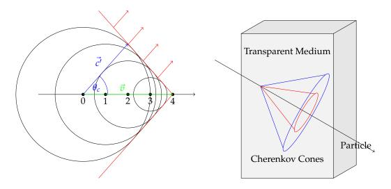
Figure 1.2.: The schematics for the derivation of the Cherenkov cone formula (left) and a 3D representation of Cherenkov angles with two different angles for red and blue photons as a result of dispersion (right).
