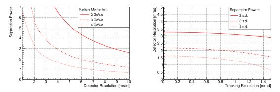
Figure 3.9.: The separation power as a function of the overall detector resolution (left) and the dependency of the required detector resolution as a function of the tracking resolution (right).
