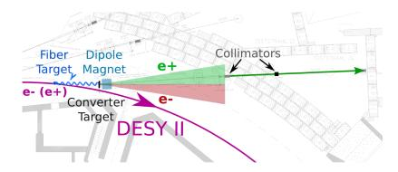
Figure 7.1.: A schematic drawing of the DESY testbeam area including the creation of  $e^+/e^-$  pairs. The testbeam data has been taken in T24. area
