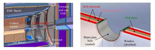
Figure 2.4.: 3D drawings of the PANDA GEM detector (left) and a 3D sketch of one of the three GEM stations (right).
