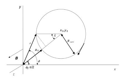
Figure 4.5.: The definitions of all relevant angles and positions for the computation of the helix propagator [Dan98].
