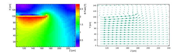
Figure 3.3.: The absolute value of the magnetic field in the EDD area (left) and the direction in every point (right).
