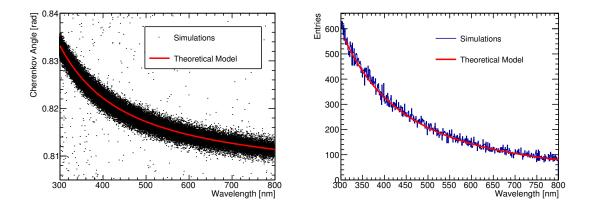
Figure 1.3.: The wavelength dependency of the Cherenkov angle on the wavelength (left) and number of photons per wavelength interval of 1 nm (right) produced by a  $\pi^+$  with the momentum p = 4 GeV/c inside a fused silica plate with a thickness of 2 cm simulated with Geant4 and compared to the theoretical model.
