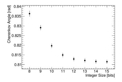
Figure 6.8.: The shift of the mean value of the reconstructed Cherenkov angle distribution as a function of the integer resolution. The detector resolution is indicated by the error bars.
