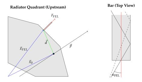
Figure 4.8.: The spatial and angular parameters (left) used for the geometrical reconstruction and the reconstruction of  $\alpha_{FEL}$  for the entering photon (right).
