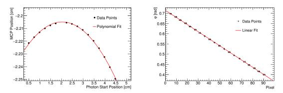
Figure 3.5.: The hit position of every photon on the MCP-PMT as a function of the initial photon position (right) and the calibration line through the photon angles  $\varphi$  against the pixel number of a hit.
