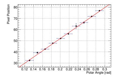
Figure 5.9.: The obtained calibration line between pixel position and polar angle.
