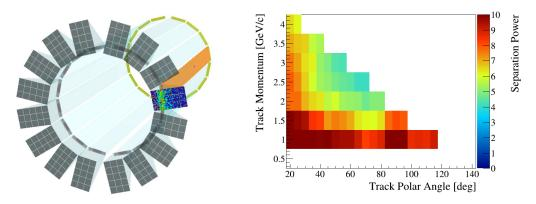
Figure 2.7.: A 3D drawing of the PANDA Barrel DIRC with the view from the forward endcap, showing the bars, expansion volumes, and MCP-PMTs (left), and the separation power for  $\pi/K$  separation with different combinations of particle momentum *p* and polar angles  $\theta$  (right).
