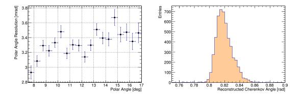
Figure 5.8.: The polar angle resolution as a function of the polar angle (left) and the obtained single photon resolution with the cosmics test stand (right).
