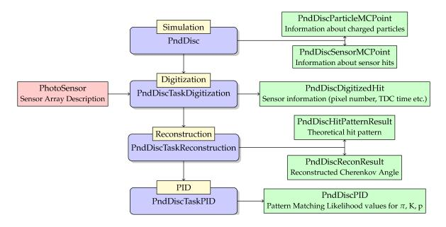
Figure 4.1.: The data flow for the Disc DIRC detector implemented in PandaRoot. The processing classes are marked with blue and the classes handling the input/output data stream are shown in green color.
