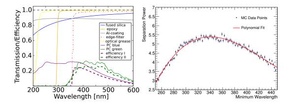
Figure 4.4.: The optical parameters implemented in Monte-Carlo simulations for two different photo cathodes (left) and the separation power between pions and kaons for p = 4 GeV/c as a function of the minimum wavelength of the bandpass filter (right).
