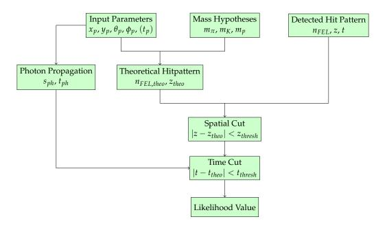
Figure 3.6.: Flow diagram of the reconstruction algorithm to calculate the likelihood value of each hit
