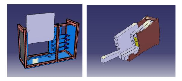
Figure 7.4.: A 3D sketch of the new prototype design including the mechanical holding mechanism (left) and the ROM holder with 3 inserted FELs (right).
