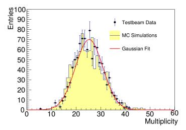
Figure 7.10.: The simulated and measured photon multiplicity with the event combination method.
