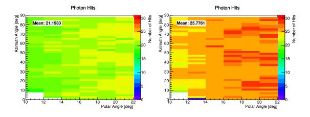
Figure 4.11.: The detected photon hits as a function of the polar and azimuth angles for the blue (left) and green (right) photocathode
