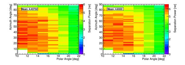
Figure 4.10.: The reconstructed separation power as a function of the polar and azimuth angles for the blue (left) and green (right) photocathode
