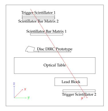
Figure 5.4.: A sketch of the proposed cosmics test stand upgrade including the two scintillator bar matrices, the optical table, the lead block, and the two trigger counters.
