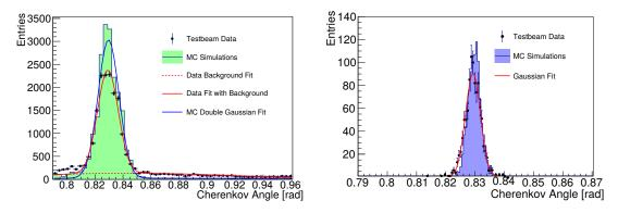
Figure 7.9.: The single photon resolution (left) and the mean angle distribution (right) of the event combination with 30 virtual FELs accumulated by grouping all 30 electron beam positions of the *y*-axis scan into one single event.
