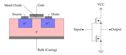
Figure 1.10.: The sketch of a typical *p* typed MOSFET structure with the four connections Source, Drain, Gate and Bulk (left) and a standard CMOS inverter circuit including two MOSFET (right).
