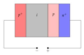
Figure 1.8.: The scheme of an APD including the highly doped layers  $p^+$  and  $n^+$ , the intrinsic layer *i* and the lightly doped layer *p*.
