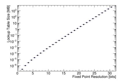
Figure 6.4.: The calculated memory consumption of a 1 dimensional lookup table as a function of the fixed point integer resolution
