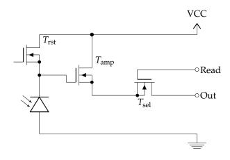
Figure 1.11.: The sketch of a minimal circuit of an APS.
