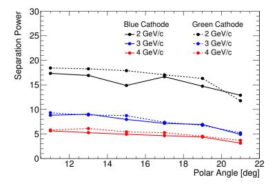
Figure 4.12.: The separation power as a function of the polar angle for two different photo cathode options.
