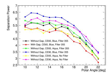
Figure 4.18.: The simulated detector performance of the EDD for different setup combinations of photocathodes, MCP collection efficiencies (CE), filters and geometries.
