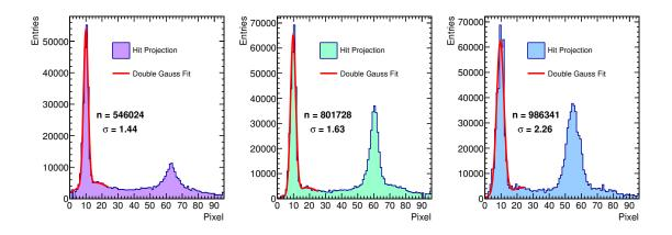
Figure 7.6.: The accumulated pixel distributions for one beam angle and position including the upper FEL0 (left), the center FEL1 (center) and the lower FEL2 (right) showing the number n of entries and the standard deviation  $\sigma$  of the main Cherenkov peak.
