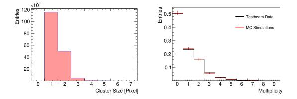
Figure 7.7.: The cluster size of the measured angle scan at  $\theta = 14^{\circ}$  (left) and the comparison of the photon hit distributions between simulation and testbeam data after applying a charge sharing model (right)
