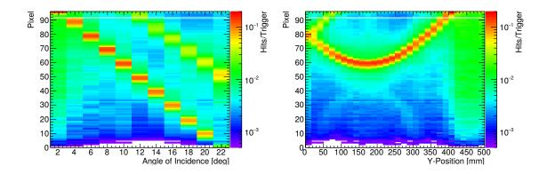
Figure 7.5.: The results from the angle scan (left) including a reflection pattern from the lower plate side and the *y* position scan (right) with a polar angle of  $\theta = 10^{\circ}$ . The exact beam position information can be taken from Figure 7.3
