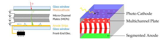
Figure 1.9.: The schematics of an MCP-PMT [GlueX14] with a transmission-line readout (left) and a not-to-scale 3D drawing of an arbitrary MCP-PMT with a hexagonal hole structure. The photon kicks out an electron from the photo cathode, which is then multiplied by microchannels inside a metal coated lead glass MCP. A segmented anode can be used for obtaining the primary photon position.
