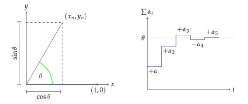
Figure 6.5.: The computation of  $\cos \theta$  and  $\sin \theta$  with the rotation of the unit vector (1,0) (left) and the representation of the iterative calculation of  $\theta$  with the CORDIC algorithm (right)
