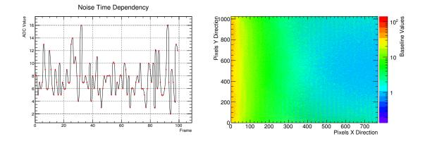
Figure 5.11.: The time behaviour of the measured noise with a CMOS camera modules (left) and the obtained baseline for one pixel of the camera module(right).
