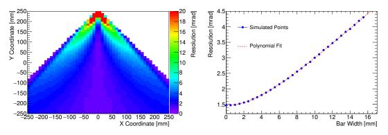
Figure 3.10.: Single Photon Resolution for a grid of different position pairs on the radiator disk (left) and as a function of the bar width (right) determined with a self-written simplified Monte-Carlo tool.
