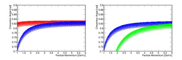
Figure 1.4.: The Cherenkov angle of pions and kaons (left) and pions and protons (right) as a function of the particle momentum including dispersion and number of photons for all wavelengths between 300 nm and 700 nm. The photon yield per wavelength interval is indicated by the density of the dots.
