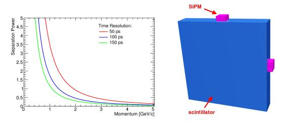
Figure 2.6.: The separation power for  $\pi^{\pm}$  and  $K^{\pm}$  in case of TOF measurements with a distance of L = 50 cm as a function of the particle momentum (left) and the conceptional design of one scintillator tile in the SciTil detector for simulation purposes (right).
