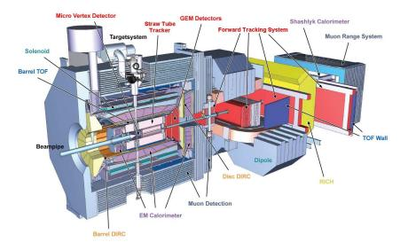
Figure 2.2.: A sketch of the PANDA spectrometer according to the actual proposal. The EDD is marked with the orange text.
