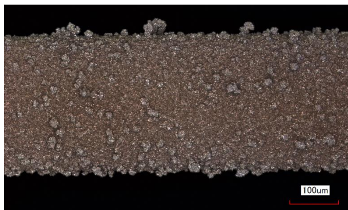
Figure 114 – Confocal laser microscopy image (laser intensity and color) of an aluminum wire on which ZnO was deposited by nitrate-based pulsating current electrodeposition. The structure directing agent EosinY is already desorbed.
