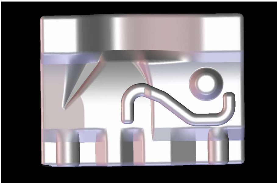
Figure 5.15: The milling result of the workpiece 'daimler'
