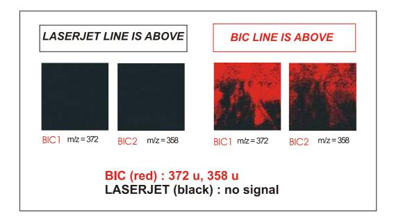
**Figure 4.38** Scanning microprobe images (100 x 100 μm) from the intersection of entries from a black BIC ballpoint pen and a Laserjet printer. The two scanned signals of the BIC pen, for m/z = 372 and 358, are reported in red, while the intensity of the signal from the Laserjet printer was too low to be recorded. When the Laserjet line is above, the images are black (no signals), but when it is below, the images are red (signals of the BIC pen).
