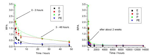
Figure 5.7 obtained by GC/MS ballpoint (E: Drying curves for four solvents PE: ethoxyethoxyethanol, D: dipropylene glycol, P: phenoxyethanol, phenoxyethoxyethanol) from Parker ballpoint pen entries. The Relative Peak Areas (RPA) plotted as functions of time are proportional to the solvent concentration. Drying slowed down considerably with time, and three stages can be distinguished: 0 to 3 hours, 3 to 48 hours and beyond two weeks.
