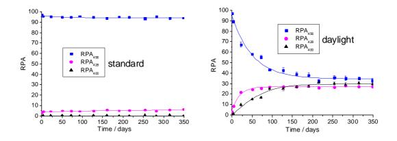
Figure 4.21 Natural aging of ethyl violet contained in ink entries from a BIC<sup>®</sup> ballpoint pen induced by the following treatments over a time of 347 days: a) standard storage in the dark, (b) exposure to daylight.
