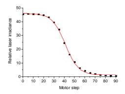
Figure 3.4 Relative laser irradiance as a function of step motor setting. An attenuator consisting of a dichroic quartz plate was placed between laser and sample, and its angle attenuating the laser irradiance transmission was adjusted by step motor. Typical MALDI and LDI mass measurements are made between steps 60 to 90.
