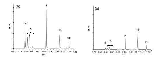
Figure 4.45 SIM Chromatograms of an extract of 1 cm Parker<sup>®</sup> ballpoint pen stroke, (a) at time t = 0, (b) at time t = 10 days after applying the ink to the paper. The x-axis represents the relative retention time (RRT) of the solvents referred to the internal standard (IS). The TIC signals of the 15 ions selected correspond to ethoxyethoxyethanol (E), dipropylene glycol (D), phenoxyethanol (P), the IS at a concentration of 0.0227 mg/ml, and phenoxyethoxyethanol (PE).
