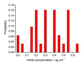
Figure 5.5 Probability histogram (scale with 0.05 steps) for the initial concentration [μg/cm] of solvent P determined by GC/MS in the inks from 31 blue ballpoint pens. There is a 16 % probability that a pen stroke contains an initial solvent quantity of 0.2, 0.3, 0.4 or 0.5 μg. Many of the values have been extrapolated from the SCAN chromatogram, and constitute single values (the error for single values may be rather large because of the fibrous character of the paper).
