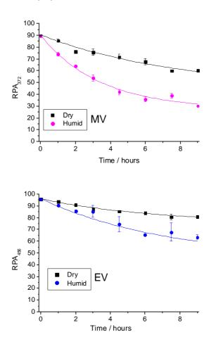
**Figure 4.18** Influence of humidity on the degradation of MV and EV from ink entries of a BIC<sup>®</sup> ballpoint pen during 9 hours of exposure to the light of a high-pressure xenon lamp. The curves show that the degradation of both dyes upon exposure to light was stronger in a humid atmosphere than in a dry atmosphere.
