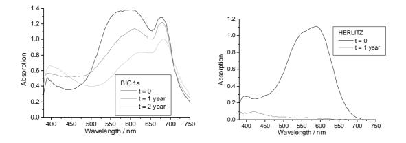
Figure 4.35 Microspectrophotometric absorption spectra of fresh and old entries from ballpoint pens BIC 1a and Herlitz. The old entries were exposed to light for 1 to 2 years, and a decrease of absorption was observed.
