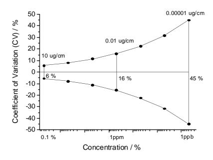
**Figure 5.11** Theoretical "Horwitz-Trumpet" for the quantitative analysis of ballpoint solvents by GC/MS calculated with the equation given by Hall and Selinger [1989]. For a concentration of 1 ppm (corresponding to 0.01 μg solvent in 1 cm ink entry), the coefficient of variation (CV) reaches 16%.
