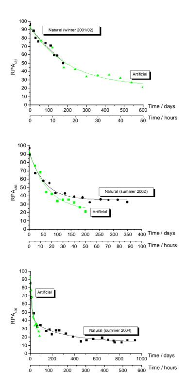
**Figure 4.23** Attempts of modelling the natural aging (NA / days) with artificial aging curves (AA / hours). Very different results were obtained for the three NA experiments (winter 2001/02, summer 2002 and summer 2004) and, except for the winter of 2001/02, the modelling of NA by AA does not yield a prefect fit of the NA curves.
