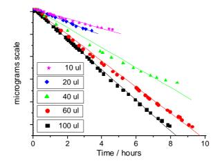
**Figure 4.43** Superimposed curves for the evaporation of 10, 20, 40, 60, and 100 μl of E from paper: the loss of weight in micrograms (Δ=56372 μg) is reported as a function of the time in hours. Lower evaporation rates were found when smaller volume of solvents was initially deposited on paper.
