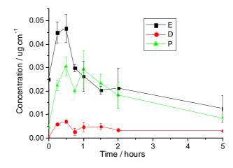
**Figure 4.52** Solvent loss by evaporation and diffusion [µg] determined for ethoxyethoxyethanol (E), dipropylene glycol (D), phenoxyethanol (P) from GC/MS measurements made at a distance of 2mm next to the ink entry, as functions of the time elapsed since apposition of the ink to the paper.
