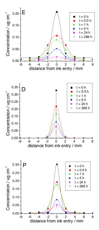
Figure 4.51 Diffusion [ug/cm] of the solvents ethoxyethoxyethanol (E), dipropylene glycol (D), phenoxyethanol (P) away from the ink stroke (0 mm) at different times t after applying the stroke to the paper. The curves represent Gaussian diffusion fits. The error ranges (not shown in the plots) are between 20 and 50% of the small quantities involved.
