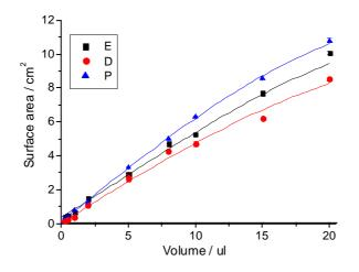
**Figure 4.44** Visible surface area [cm<sup>2</sup>] taken up by the solvents E, D and P a short time after deposition on paper, as functions of the volume deposited [µl]. The surface areas increased with the volume, but were also influenced by the viscosity, density, and volatility of the solvents.
