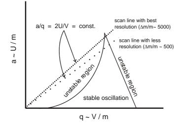
Figure 2.5 Stability diagram for a two dimensional quadrupole mass filter derived from Mathieu's differential equations. U and V are the amplitudes of the dc and rf voltage, respectively.
