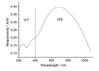
**Figure 3.3** Responsivity in A/W as a function of the wavelength of the UV enhanced photodiode (UDT-UV100).
