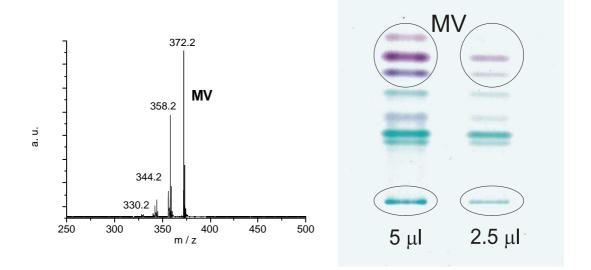
Figure 4.4 LDI mass spectra (to the right) and HPTLC plate (to the left) of the BIC 1b ballpoint pen. While only MV was detected by LDI-MS, at least two additional dyes were detected by HPTLC analysis. One dye did not migrate on the plate.
