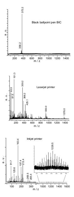
Figure 4.36LDI mass spectra of ink entries from a black BIC ballpoint pen, an HP Laserjet<br/>printer and, an HP Deskjet printer. The ballpoint ink only contained the dye MV.<br/>Signals from the printer mass spectra remained unidentified.
