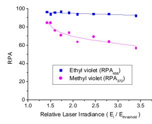
**Figure 4.7** Fragmentation of MV (RPA<sub>372</sub>) and (EV RPA<sub>456</sub>) calculated as a function of the laser irradiance from the LDI-MS spectra of the BIC<sup>®</sup> 1a ballpoint pen. For this particular ink, the dye MV was found to be less stable to laser irradiance than the dye EV. A relative value of 1.5 was chosen for the operative fluence in the measurements.
