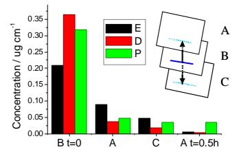
Figure 4.53 Migration of the solvents ethoxyethoxyethanol (E), dipropylene glycol (D), phenoxyethanol (P) from an ink entry to an adjacent sheet of paper during a 15 min contact (values correspond to single measurements): quantities in the stroke at t=0 (B), quantities in a sheet of paper placed over B (A), quantities in a sheet of paper placed under B (C), and quantities in a sheet placed over B (A) 0.5 hours after apposition of the ink entry on B.
