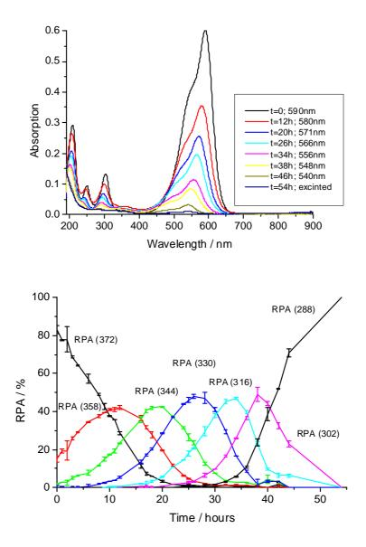
Figure 4.10 Exposure of an aqueous solution of MV (0.009 mg/ml) to xenon light (a) UV/VIS absorption spectra for different illumination times, (b) Relative Peak Area (RPA) values for different ionic species calculated from the MALDI mass spectra as a function of time [hours]. The RPA values describe degradation of the dye and production and further degradation dye fading products.
