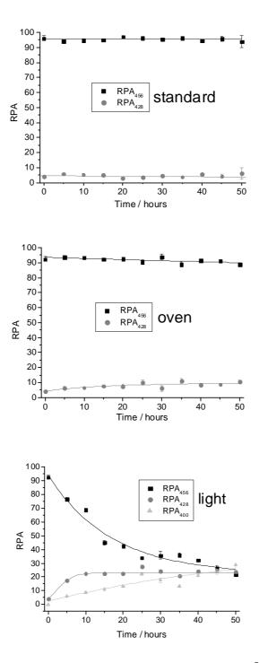
**Figure 4.17** Artificial aging of EV contained in ink entries from a BIC<sup>®</sup> ballpoint pen, induced by the following treatments over a time of 50 hours: (I) storage in the dark at room temperature, (II) storage in an oven 100°C, and (III) exposure to a high-pressure xenon lamp. The aging curves show that heat caused slight degradation of ethyl violet, while light had a strong effect already observed after a few hours exposure.
