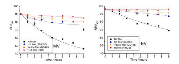
**Figure 4.20** Influence of the wavelength of incident light on the degradation of MV and EV from BIC<sup>®</sup> ballpoint pen entries during 9 hours of exposure to light of a high-pressure xenon lamp. The incident light was filtered using three different filters, each leading to degradation within a restricted wavelength window.
