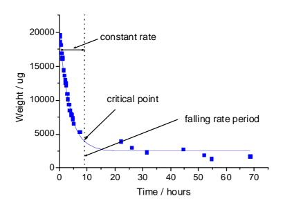
**Figure 4.42** Drying curve recorded with 20 µl of solvent E on paper: the periods of constant and falling rate can be distinguished; the slope of the curve represents the drying rate [µg/hour].
