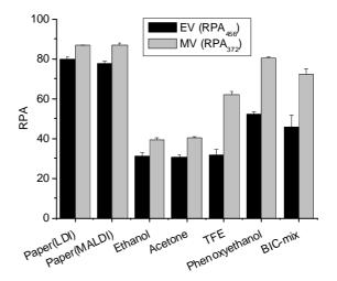
**Figure 4.8** RPA<sub>456</sub> (EV) and RPA<sub>372</sub> (MV) values from LDI and MALDI mass spectra of BIC<sup>®</sup> ballpoint pen strokes on paper as well as from MALDI mass spectra of extracts of the paste from BIC<sup>®</sup> ballpoint pen entries (about 2 cm) in diverse solvents. The results with the minimal fragmentation were obtained for the measurements performed directly on the paper (high RPA values).
