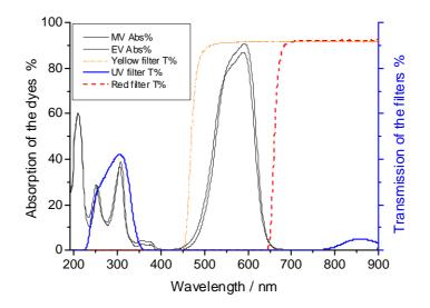
Figure 4.19 Absorption spectra of MV and EV, and spectral transmission curves of three filters: UV (SB300F), yellow (GG445) and red (RG5).
