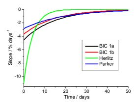
**Figure 4.28** Plots of the slopes of degradation of MV [%·s<sup>-1</sup>] extrapolated from the theoretical exponential fittings as functions of time [days] show that Herlitz MV degraded very strongly during the first ten days, while Parker MV degradation was least pronounced over the first few days, but was very close to MV fading in BIC1a and BIC1b inks. After 50 days, degradation had slowed down considerably for all four ballpoint pens.
