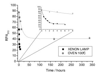
**Figure 4.9** Comparison of the degradation of methyl violet (~1 mg/ml in ethanol) provoked by light from a high-pressure xenon lamp (d = 17cm) over a period of six hours, and by heat in an oven at 100°C over a period of 336 hours (14 days). Upon exposure to light, the RPA<sub>372</sub> values dropped from ~97% to ~25 % after 3 hours. The RPA<sub>372</sub> value of sample stored in the oven had dropped to ~40% after 7 days treatment and remained roughly constant upon further exposure.
