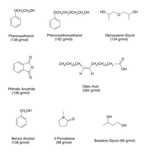
Figure 2.2 Structure of solvents typically used in ballpoint inks: phenoxyethanol, phenoxyethanol, dipropylene glycol, phthalic anhydride, oleic acid, benzyl alcohol, 2-pyrrolidinone and butylene glycol.
