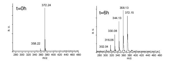
Figure 4.1 MALDI-MS Spectra of MV (methyl violet; M<sup>+</sup>=372.2 u) dissolved in ethanol (~1mg/ml) prior to and after 6 hours of exposure to the light of a high-pressure xenon lamp: signals from five of six degradation products of MV (Δ=14 u) are present. The sixth degradation product with m/z = 288.0 u was observed after longer exposure.
