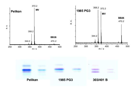
Figure 4.5 In the LDI-MS spectra (above) of the ink entries from ballpoint pens Pelikan and 1985 PG3, signals from the dyes MV and BB26 have been identified. On the TLC plate (below), ink entries of the ballpoint pens Pelikan, 1985 PG3 and 303/401 B spots from MV (violet) and BB26 (blue) have also been identified, but they are partly superposed because they did elute together. When one of the dyes is markedly more concentrate than the other, it is difficult to identify both dyes.
