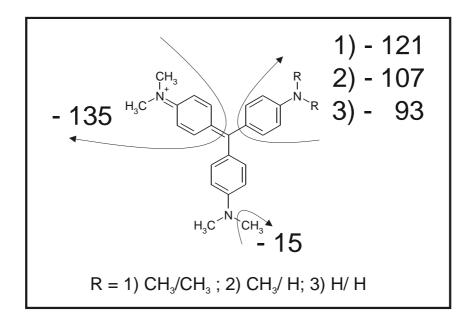
Figure 4.13 The fragmentation pattern suggested for MV, and the *N*-demethylated degradation products of MV, observed with the linear trap and identified by massloss analysis as follows: -15 u (corresponding to the loss of a methyl group), -93 u (loss of an aminobenzene), -107 u (loss of a methylaminobenzene), -121 u (loss of a dimethylaminobenzene) and -135 u (loss of p-methyldimethylaminobenzene moiety).
