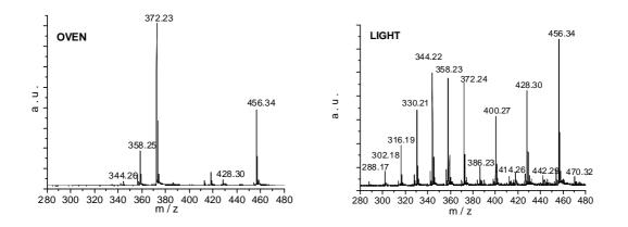
**Figure 4.16** LDI-MS spectra of a BIC<sup>®</sup> blue ballpoint entries on paper recorded at time t = 50 hours: (a) spectrum of ink entries stored in an oven at 100°C, (b) spectrum of ink entries exposed to a high-pressure xenon lamp.
