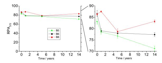
**Figure 4.32** Degradation values (RPA<sub>372</sub>) for the *N*-demethylation of MV in entries of three ballpoint pens provided by the BKA. A very slight fading was observed after 5 and 14 years, but remains within the limits of the relative standard deviation of 10%.
