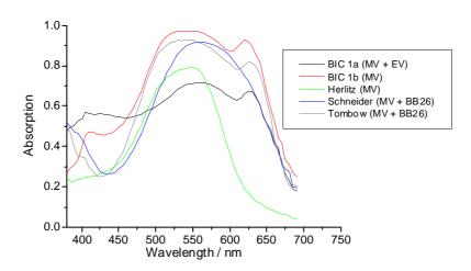
**Figure 4.34** Comparison of microspectrophotometric absorption spectra of five ballpoint pens containing MV (Bic1a, Bic1b, Herlitz, Schneider and Tombow). The RSD for ten spectra can be as high as 25 %, therefore, only the spectrum obtained fo the Herlitz ballpoint pen ink was significantly different.
