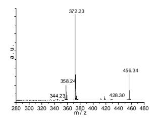
Figure 4.15 LDI-MS spectrum of a BIC<sup>®</sup> blue ballpoint pen entry on paper at time t = 0. The ink contained the dyes methyl violet (M<sup>+</sup> = 372.2 u) and ethyl violet (M<sup>+</sup> = 456.3 u). Smaller signals at m/z = 428.4 u, 358.3 u represent degradation products of the molecular ions and / or compounds contained in the ink paste composition.
