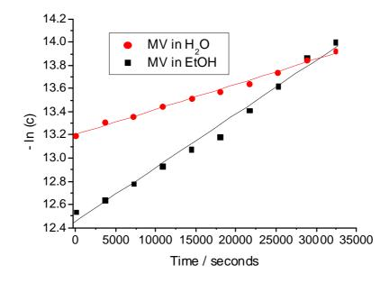
**Figure 4.10** Representation of the negative logarithms of MV concentrations in water and ethanol as a function of the time [s]. The slopes as obtained from the linear regression equations yield the rate constant k [s<sup>-1</sup>] of the pseudo first-order fading reaction. Fading is about twice faster in ethanol than in water.
