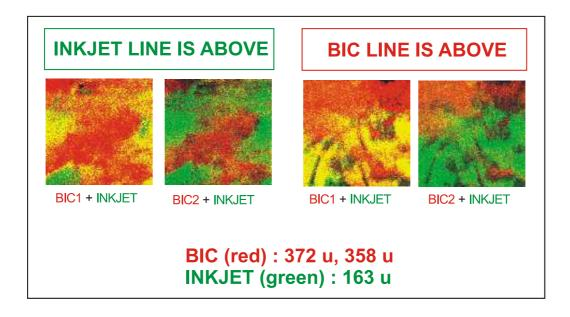
**Figure 3.40** Scanning Microprobe images (100 x 100  $\mu$ m) from the intersection of entries from a black ballpoint pen BIC and an inkjet printer. The two scanned signals of the BIC pen m/z = 372 and 358 u are reported in red, the signal from the inkjet printer m/z = 163 u is reported in yellow and the superposition of the two type of signals is reported in green. These are limit cases, where it is impossible to identify which signal is above from the obtained results.
