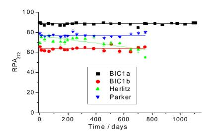
Figure 4.25 Relative peak areas (RPA<sub>372</sub>) for m/z= 372 u plotted against time in days provide a basis for comparison of the fading of methyl violet from four ballpoint pens on paper during storage in the dark. Measurements have been carried out over a period of three years for the BIC1a (no fading) and during two years for the BIC 1b (no fading), Herlitz (slight fading) and Parker (no fading).
