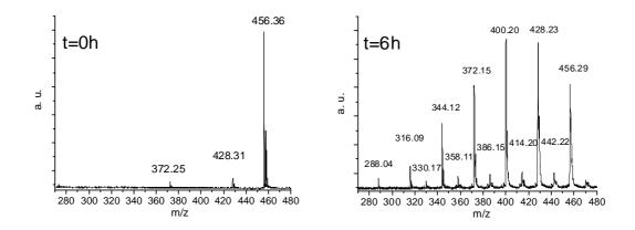
**Figure 4.2** MALDI-MS Spectra of EV (ethyl violet;  $M^+$ =456.4 u) dissolved in ethanol (~1mg/ml) prior to and after 6 hours of exposure to the light of a high-pressure xenon lamp: strong signals from six degradation products ( $\Delta$ =28 u) and, between them, another set of five weaker signals from six degradation products ( $\Delta$ =14 u).
