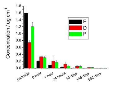
Figure 4.47 Masses per unit stroke length of the solvents ethoxyethoxyethanol (E), dipropylene glycol (D), phenoxyethanol (P) and phenoxyethoxyethanol from a Parker<sup>®</sup> ballpoint pen, determined from the cartridge weight loss and from GC/MS measurements of residual concentration at different times after application on paper.
