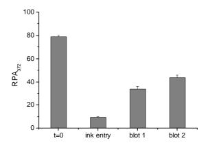
**Figure 4.31** The Parker ballpoint pen during writing produced small blots that were thicker than the ink entries. Their analyses by LDI-MS after a time of about two years produced higher RPA<sub>372</sub> values in the blots than in the rest of the entry, demonstrating the influence of the local amount (or concentration) of the dye on fading during exposure to light.
