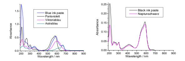
Figure 4.3 Absorption spectra of blue ink paste and its dye component mixtures (Parisviolett, Viktoriablau, Astrablau), as well as black ink paste and its dye component mixture (Neptunschwarz). The powders were dissolved to 0.01 mg/ml in ethanol for UV/VIS analysis.
