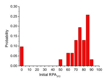
**Figure 5.4** Probability histogram (on a scale of 5% steps) for the initial RPA<sub>372</sub> values obtained by LDI-MS for the dye MV in 31 blue ballpoint pens inks. There is 26 % probability that a pen has an initial value of 85%, a 10% probability that a pen does not contain MV and a 0% probability that a pen has initial RPA<sub>372</sub> values as low as 55% or as high as 95%.
