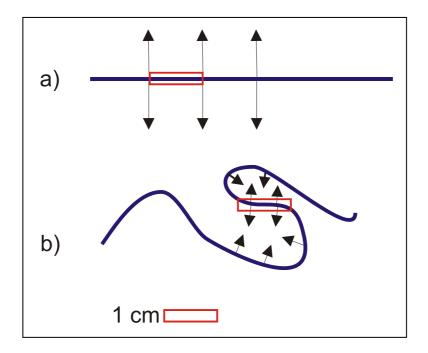
**Figure 5.6** Solvents diffusion from two ink entries: (a) diffusion away from a straight line, (b) diffusion inside the loops of a curved line. The solvent concentration might significantly be larger in 1 cm of (b) compared to 1 cm of (a).
