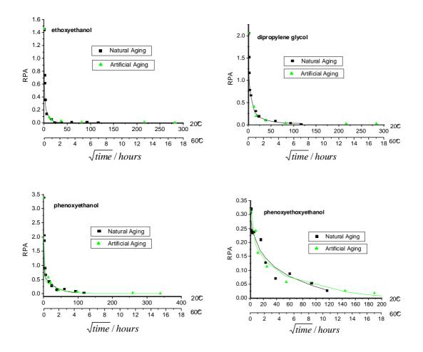
**Figure 4.50** Attempt to model the natural aging (20°C) by artifi cial aging (60°C) curves. RPA values are reported as functions of the square root of time. Different results were obtained for the four solvents E, D, P and PE. Surprisingly, it is the solvent P with a high boiling point, whose aging is most strongly accelerated by an increase of the temperature.
