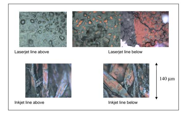
**Figure 4.37** Microscopic images of heterogeneous crossing of lines created with a black ballpoint pen and with two printers. The images reveal which entry is above, in the case of Laserjet lines, but not in the case of Inkjet lines. This can be explained in terms of different surface structures of inks that have been deposited.
