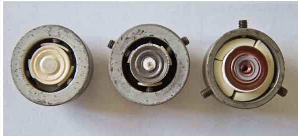
Figure 6.1: Targets used for the preparation from left to right: YSZ, \text{Sc}_2\text{O}_3 , \text{Lu}_2\text{O}_3 .
