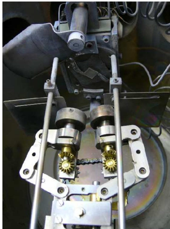
Figure 6.2: a) Sctech of the high-vacuum chamber used for PLD-preparations. b) Photo showing the interior of the PLD chamber.
