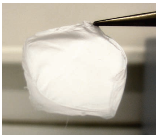
Figure 3-16: Digital photograph of a “textile” of PVP-ZIF-8 hybrid nanofibers
