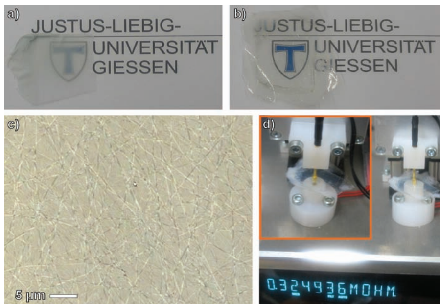
Figure 2-15: Digital photograph of ATO nanofiber mats a) in air and b) inside PS, c) of ATO-PS film with a laser microscope and d) the setup for the conductivity measurement
