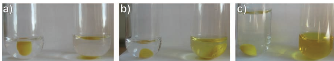
Figure 4-13: A drop of 10 wt% \text{FeCl}_3 in EtOH (left) and of 30 wt% \text{FeCl}_3 in DMF (right): a) after dropping, b) after mixing and c) after addition of more EtOH (left) or two of drops of DMF (right) and mixing
