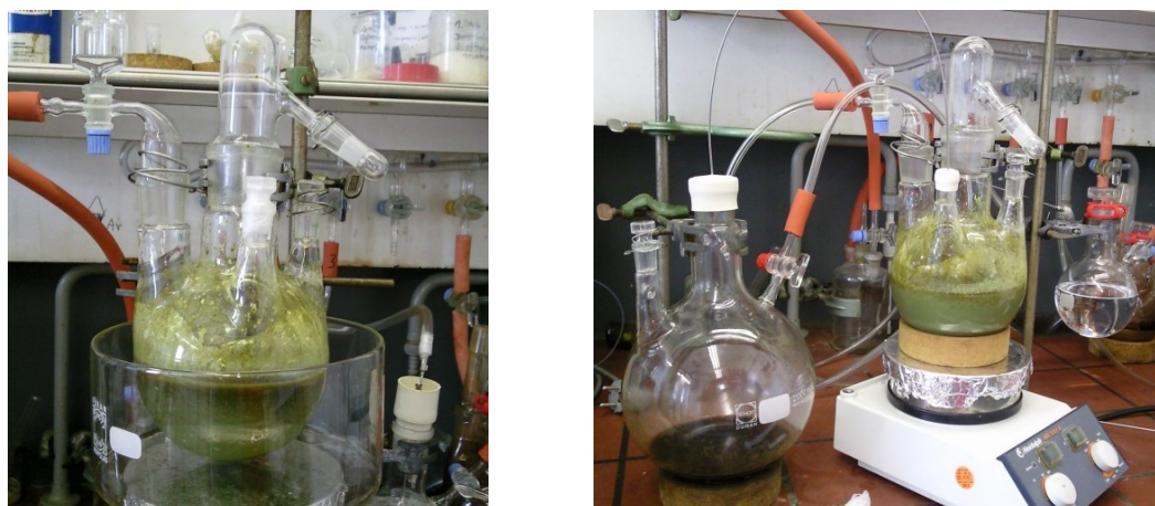
Figure 7-2: a) Final product before separation. b) Separation of the final product with benzene. The benzene was transferred into a flask with potassium hydroxide.
