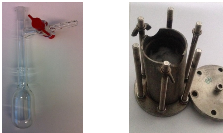
Figure 7-1: a) The bomb tube for the synthesis. b) Vessel with which the bomb tube was placed in the oven.
