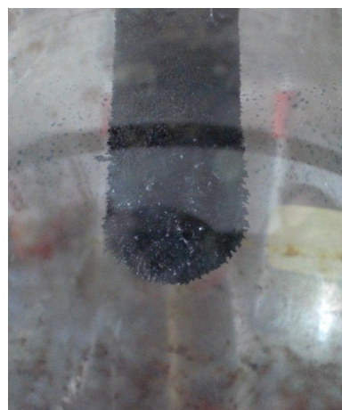
Figure 7-4: a) Sublimation of bis(benzene)chromium. b) Cold trap with crystals of bis(benzene)chromium.
