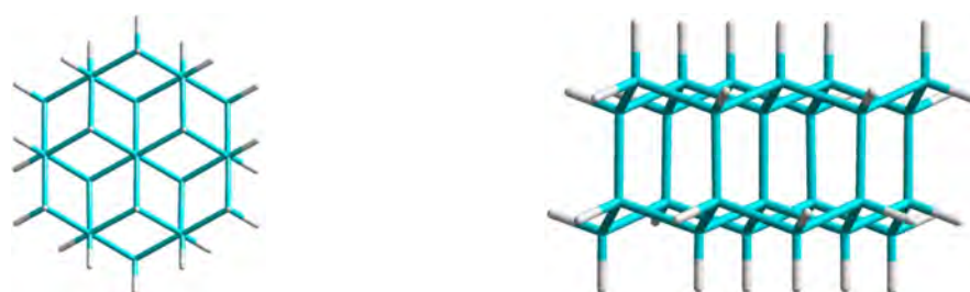
Figure 1.2. Carbon framework of cyclohexamantane C_{26}H_{30} based on single-crystal X-ray diffraction with a view along a diamond (111) crystal-lattice plane (left), and “wheel-like” side view of the same molecule (right).
