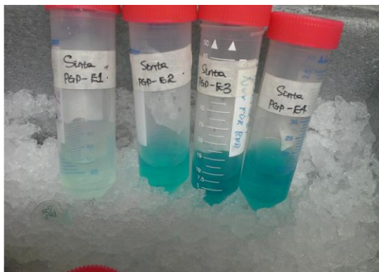
Figure 3.18. Blue-green protein solution from the original purification protocol. The blue-green coloration of in vivo assembled PGP in different fractions from the Ni-NTA column allows the elution process to be monitored by eye.
