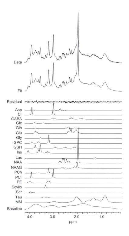
Figure 6: The method of basis spectrum fitting. The entire spectrum is fit to a linear combination of model spectra or basis spectra. Each basis spectrum corresponds to an individual metabolite, and the amplitude of the basis spectra represents the metabolite concentrations (Stagg et al., 2013).
