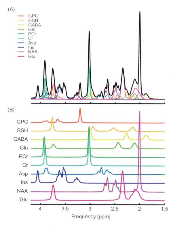
Figure 5: Quantification of <sup>1</sup>H MR spectra as a linear combination of model spectra (LCModel). (A) <sup>1</sup>H spectra comprise a sum of signals from the apparent neurochemical profile. (B) The spectrum contains a combination of the spectral patterns from individual metabolites. The necessary scaling corresponds to the apparent concentration of the substances. (Stagg et al., 2013).
