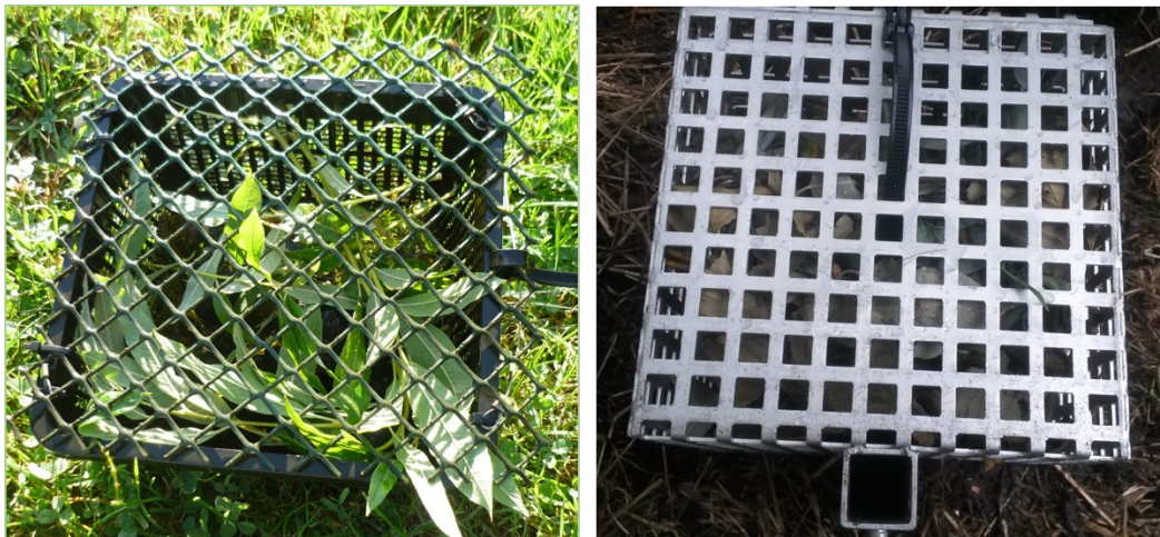
Fig. 6: Baskets for attracting macroinvertebrates (filled with basalt stones and leaf material). Left: basket for case study I, right: basket for case study II.
