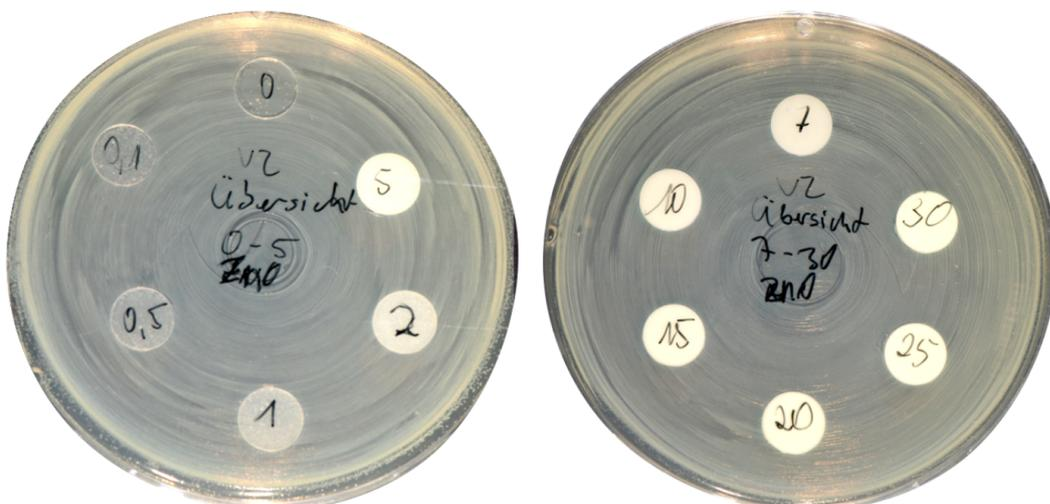
fig. 34) Zinc oxide, no inhibition zones. Test series two.
