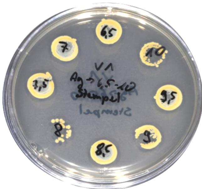
fig. 50) Growth control from underneath the specimens, follow up experiment – agar plate with high concentrations. High reduction of bacteria at 8.0% and 10.0% silver 2-ethylhexanoate. Test series one.
