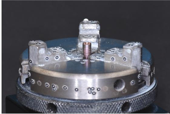
fig. 26) Three point holding device with implant
