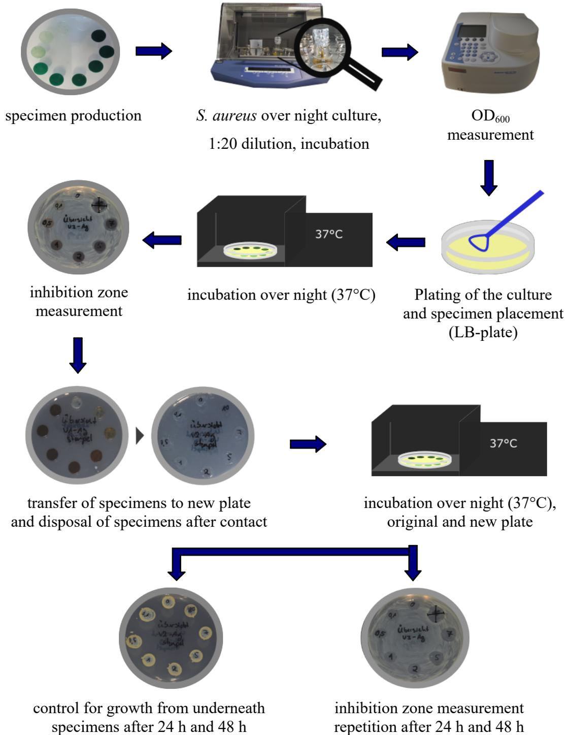
fig. 21) Outline experiment "agar diffusion test / bacterial growth inhibition on agar", (OD<sub>600</sub> = optical density at 600 nm; LB = lysogeny broth)
