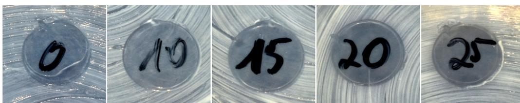
fig. 48) Close-ups from the growth control plate. 0-15% copper naphthenate similar bacterial smear layers, at 20% and more noticeably at 25% reduced smear layer.
