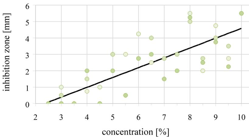
fig. 42) Silver 2-ethylhexanoate specimens' inhibition zones sizes, day three, with linear trend line.
