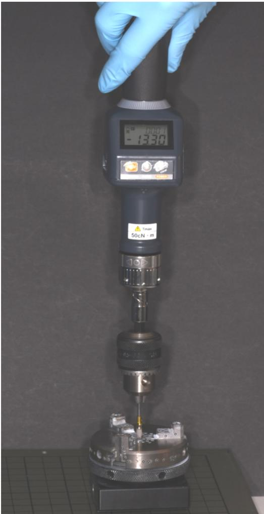
fig. 32) Unfastening the implant-abutment connection
