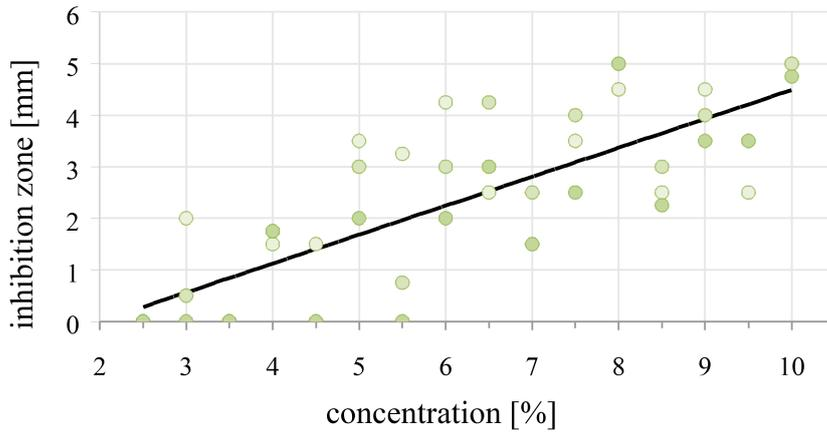
fig. 40) Silver 2-ethylhexanoate specimens' inhibition zones sizes, day one, with linear trend line.
