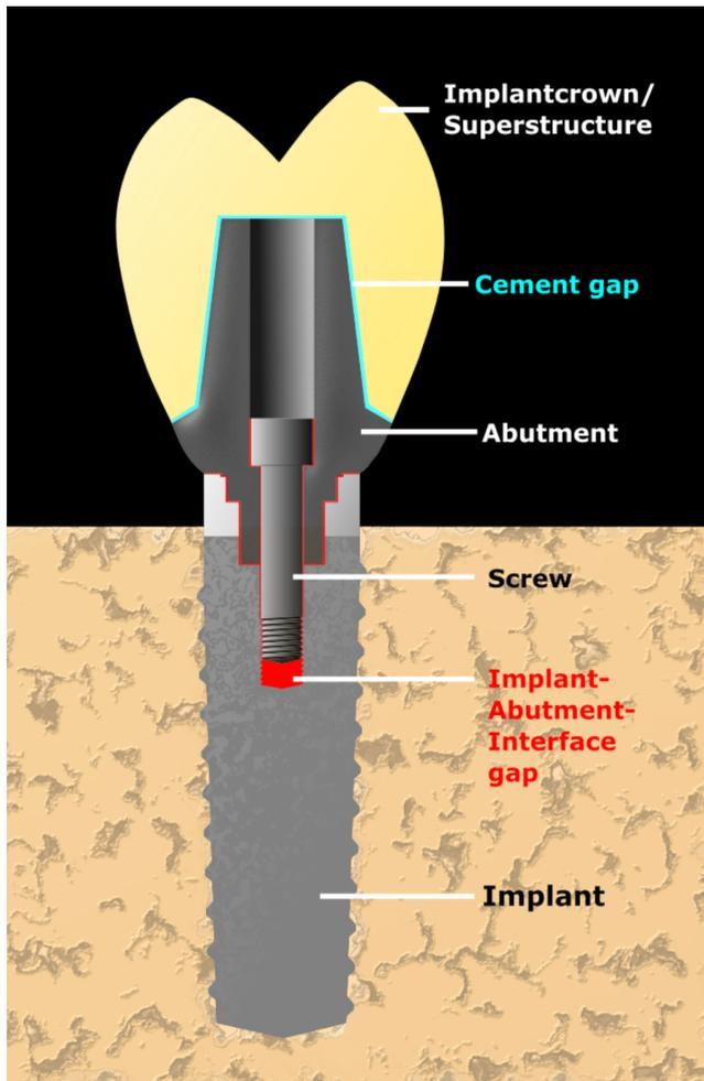
fig. 1) Structure of an implant with a screw retained abutment and cemented crown as superstructure
