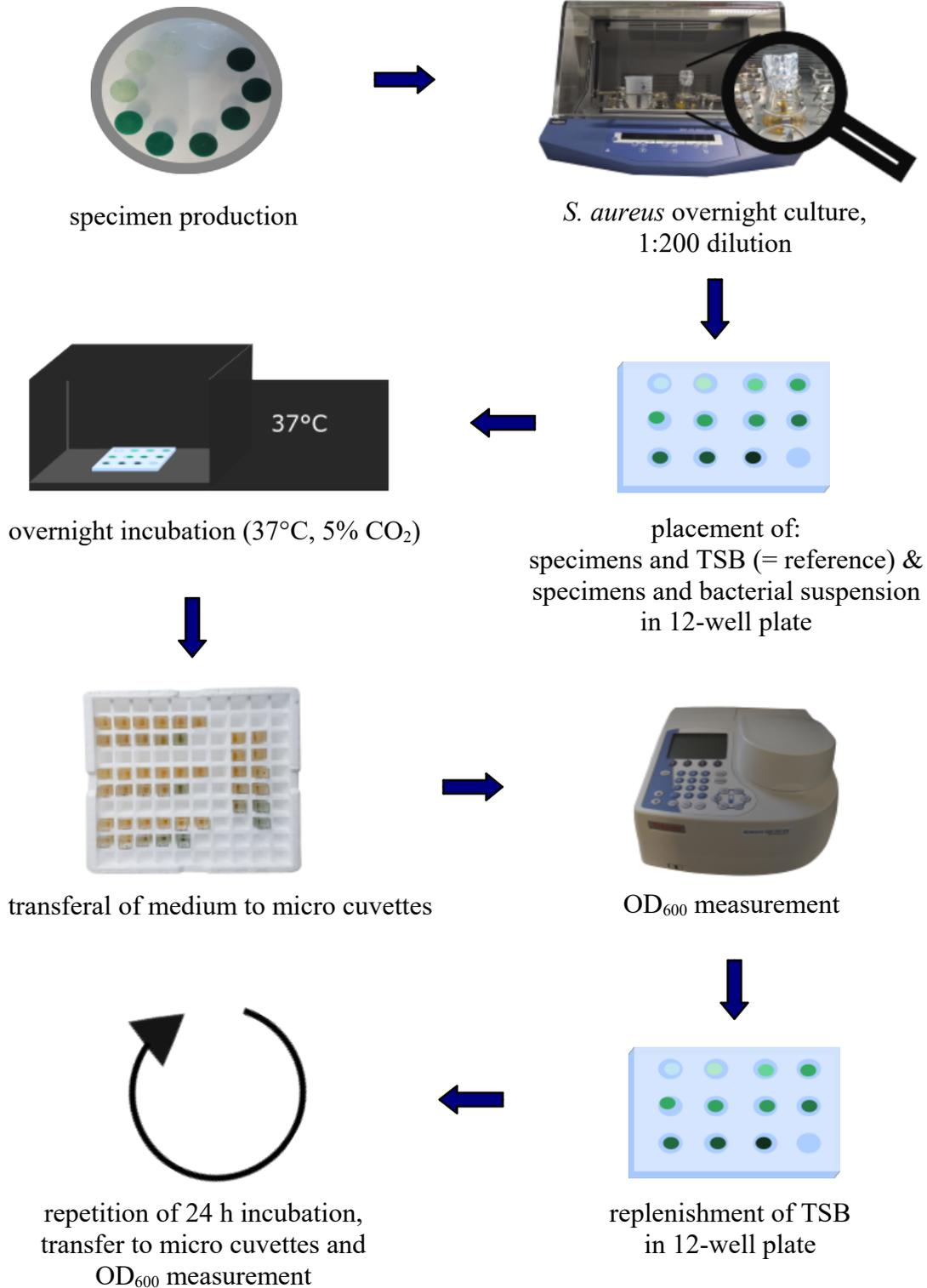
fig. 23) Outline experiment "growth inhibition in liquid medium" (TSB= tryptic soy broth; OD<sub>600</sub>= optical density at 600 nm)
