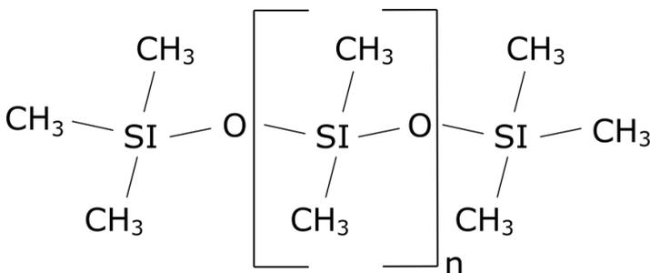
fig. 3) General chemical structure of silicones
