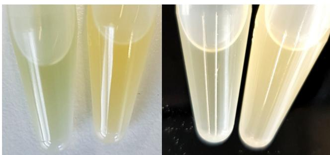
fig. 24) Surrounding tryptic soy broth of 25% copper naphthenate (see chapter 4.1.2.2) specimen (green tinge) and 0% copper naphthenate specimen (yellow tinge), at the end of biofilm incubation in front of black and white backgrounds.
