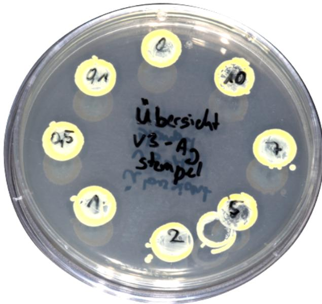
fig. 49) Growth control from underneath the specimens' preliminary experiment. Reduced density of bacteria in the centre at 10% silver 2-ethylhexanoate.
