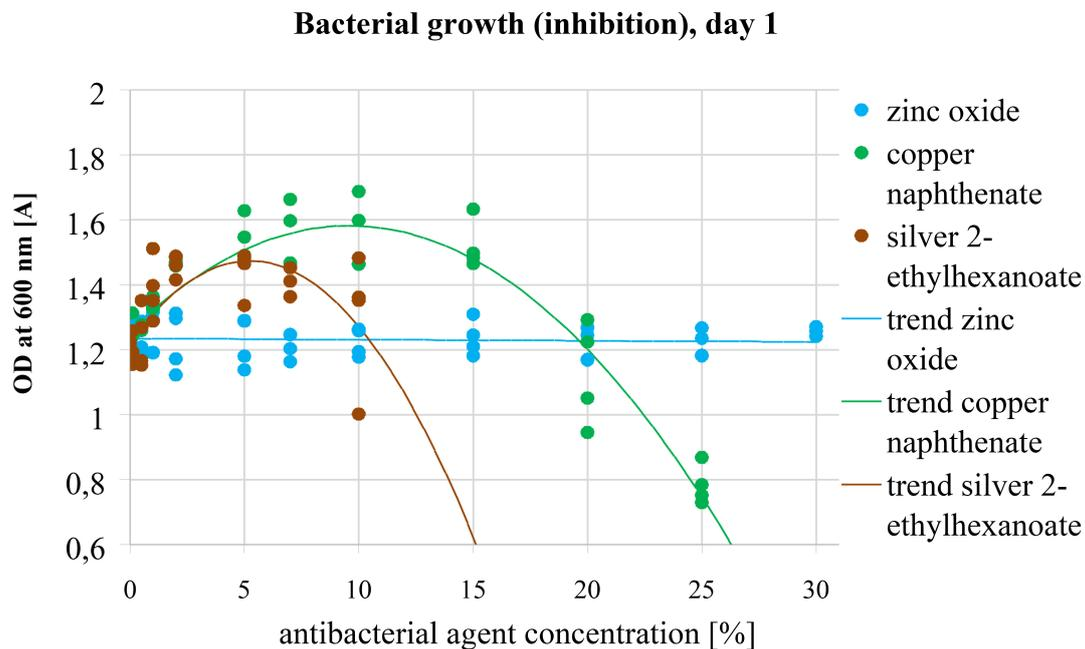
fig. 54) Bacterial growth (inhibition) in liquid medium, day one
