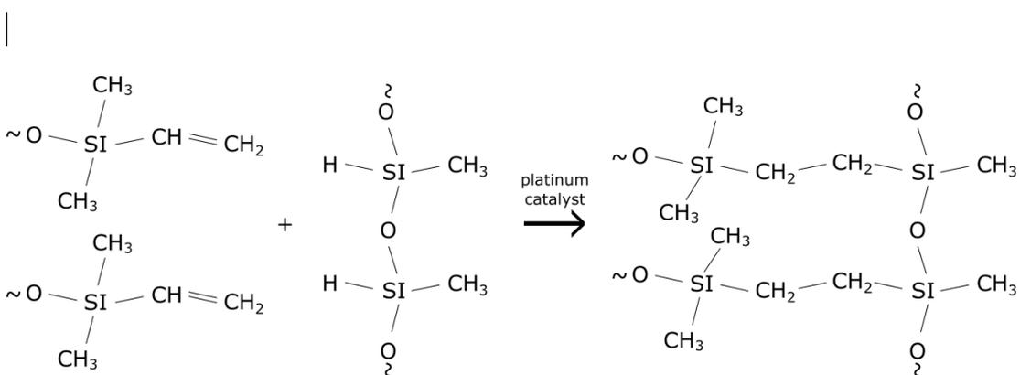
fig. 4) A-silicone, simplified setting reaction
