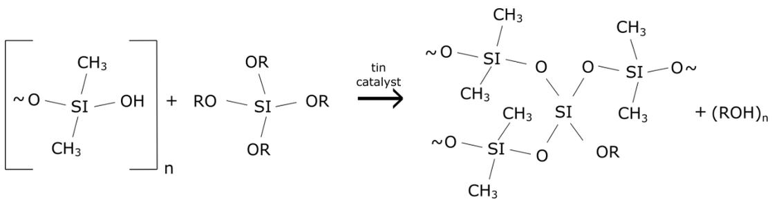
fig. 5) C-silicone, simplified setting reaction
