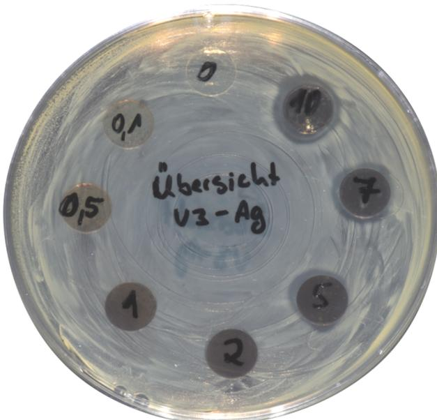
fig. 36) Inhibition zones on silver 2-ethylhexanoate preliminary concentrations. Test series one.
