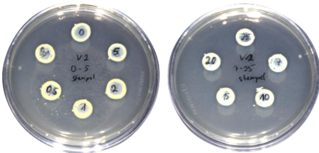
fig. 45) Growth control from underneath the copper naphthenate specimens
