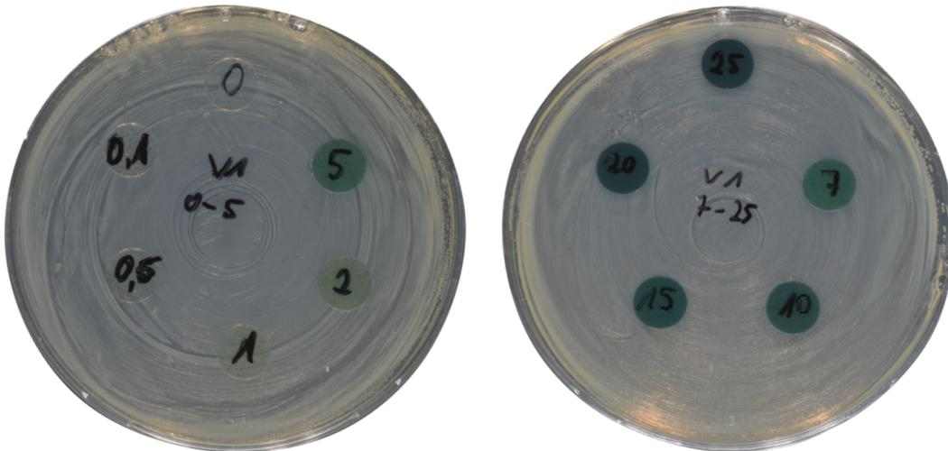
fig. 35) Copper naphthenate, no inhibition zone. Test series one.
