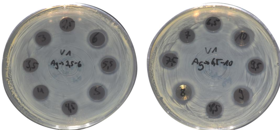
fig. 38) Silver 2-ethylhexanoate inhibition zones, concentrations of 2.5% - 10.0%. Test series one.
