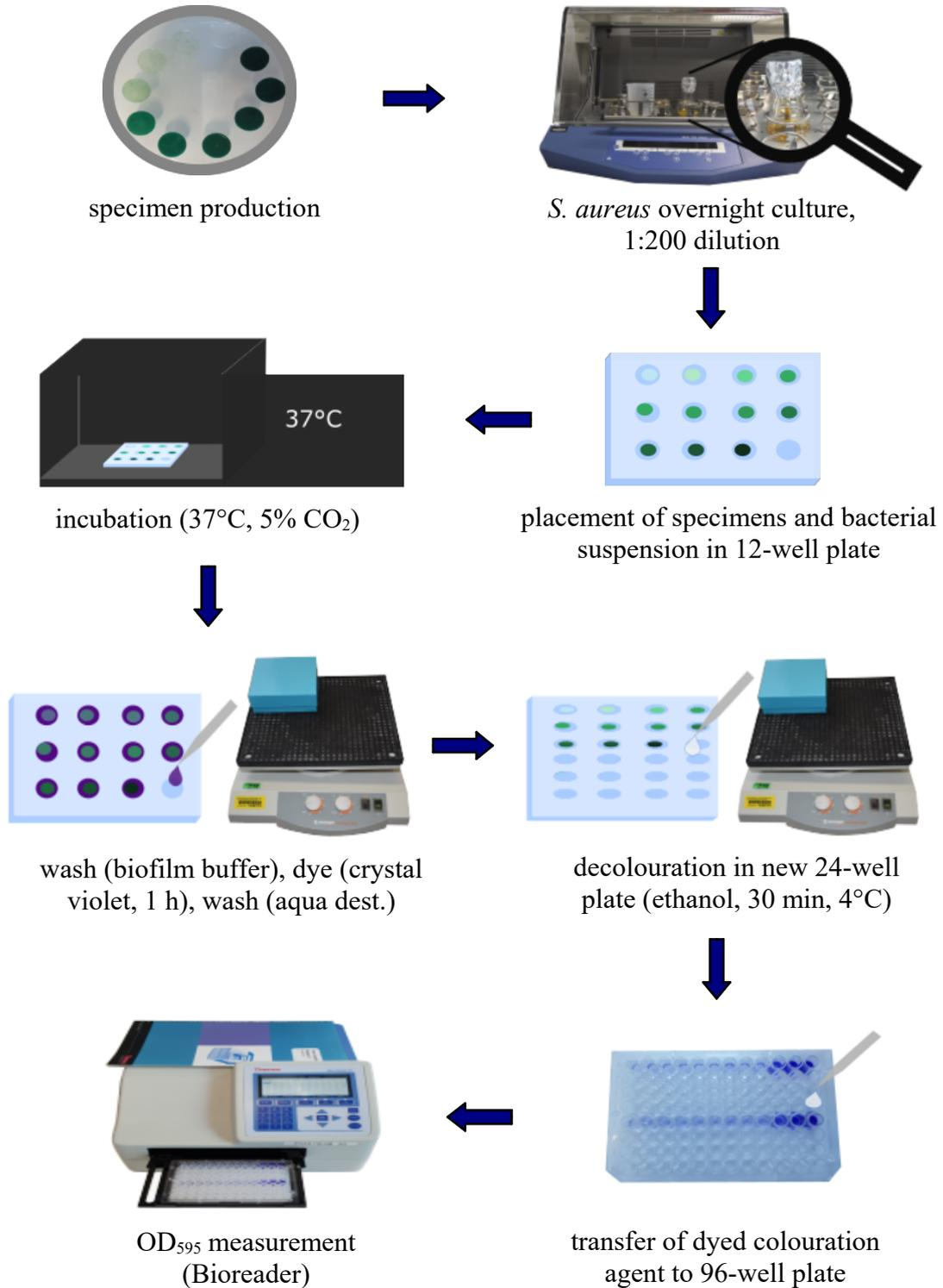
fig. 22) Outline experiment "biofilm assay" (OD<sub>595</sub> = optical density at 595 nm)
