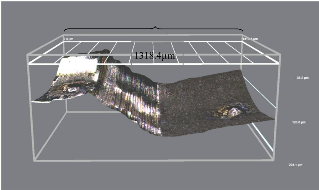
fig. 30) Inverted 3D reconstructed image of the implant-abutment interface
