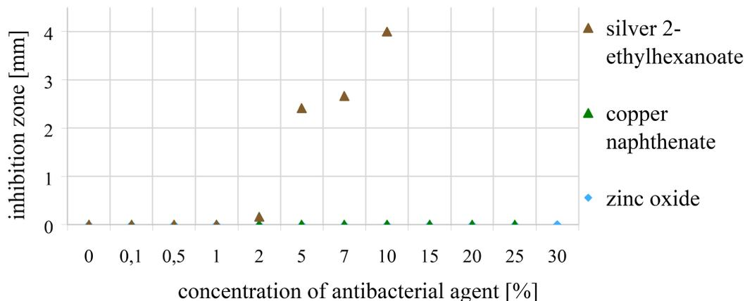
fig. 37) Mean of inhibition zone sizes per preliminary concentrations of antibacterial agent.
