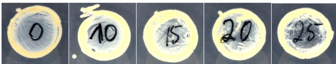
fig. 46) Close-ups from the growth control plate, 0%-15% had no change in density of bacterial lawn, slight decrease in the centre at 20%, and more of a decrease at 25% copper naphthenate.
