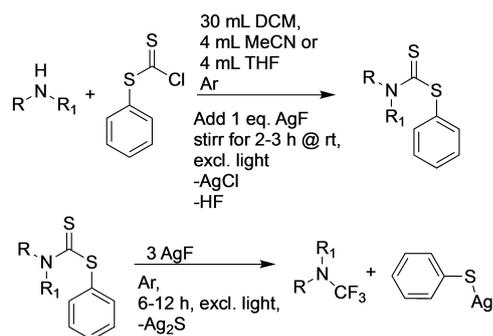
**Scheme 2.** Method c, improved new method for the synthesis of trifluoromethyl amines ( $R, R_1$  = different carbon chains, any secondary amine).
