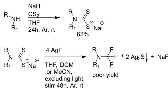
Scheme 1. Method a, based on a combination of previous work by Tyrra and Tamejira.<sup>[4]</sup> R, R<sub>1</sub> = different carbon chains.
