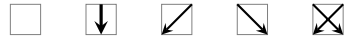
Figure 1: The states of the CA F_A in Section 3.1, where the first state is called BLANK , and the second state is called WALL . The last two states contain a right arrow, and the third and the last states contain a left arrow.
