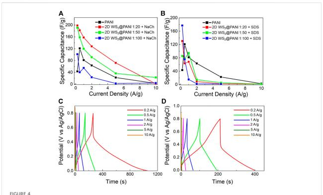
Electrochemical performance of 2D WS2@PANI nanohybrids at neutral pH (in 0.5 M Na2SO4 electrolyte). Specific capacitance as a function of current density for 2D WS2@PANI nanohybrids at different molar ratios prepared in the presence of (A) NaCh and (B) SDS. The data for pure PANI are also provided for the sake of comparison. GCD curves at increasing current densities for (C) the 1:20 2D WS2@PANI nanohybrid prepared in the presence of NaCh and (D) for pure PANI.
