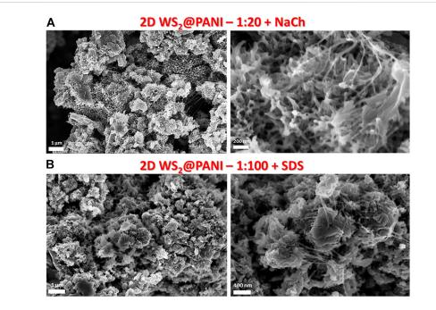
FIGURE 2 SEM images at different magnifications of prototypical nanostructured 2D  $WS_2@PANI$  nanohybrids obtained with different LPE  $WS_2/PANI$  molar ratios and with different surfactants favouring the proper mixing of the two individual components in the composite. (A) 2D  $WS_2@PANI$  with 1: 20 molar ratio prepared in the presence of NaCh as surfactant. (B) 2D  $WS_2@PANI$  with 1:100 molar ratio prepared in the presence of SDS as surfactant.
