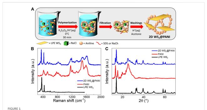
(A) Schematic representation of the template-assisted synthesis of nanostructured 2D WS<sub>2</sub>@PANI nanohybrids. (B) Raman spectra and (C) P-XRD diffractograms of the nanostructured 2D WS<sub>2</sub>@PANI nanohybrids, of template-assisted synthesized pure PANI and of LPE WS<sub>2</sub> (the P-XRD pattern of this last one has been obtained from the filtered powder).
