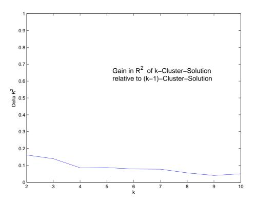
Figure 10.8: K-Means-Clustering of MC-parameter study results: Plot shows gain in  $R^2$  for k-cluster solution as compared to (k-1)-cluster solution.
