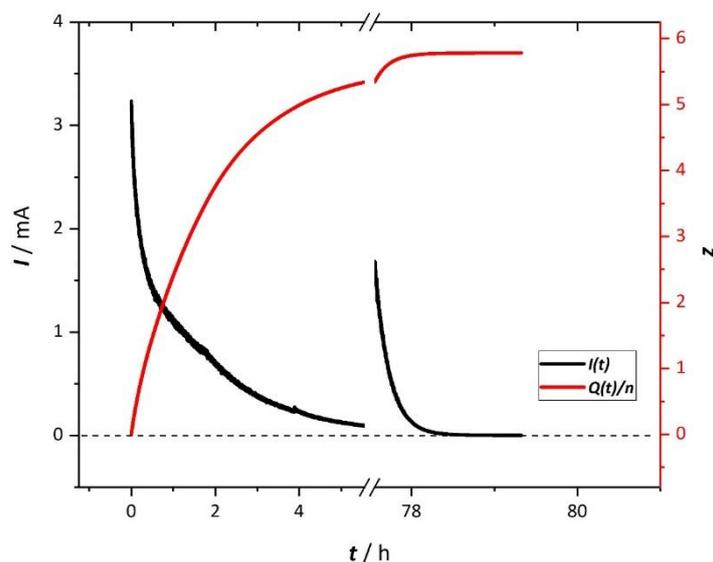
Figure 15: Overoxidation of DHP. Measured by Hofmann et al.<sup>172</sup> The gap in the curve was caused by pausing the experiment
