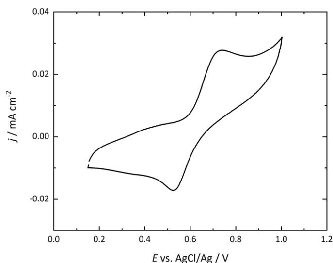
Figure 13: Cyclic voltammogram of **459** ( $E_{1/2} = 655$  mV, 2 M HCl, scan rate 10 mV/s) measured by Hoffmann et al.<sup>206</sup>
