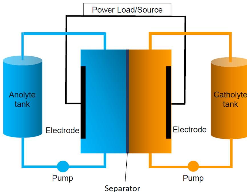
Figure 2: Redox flow battery.<sup>10</sup>
