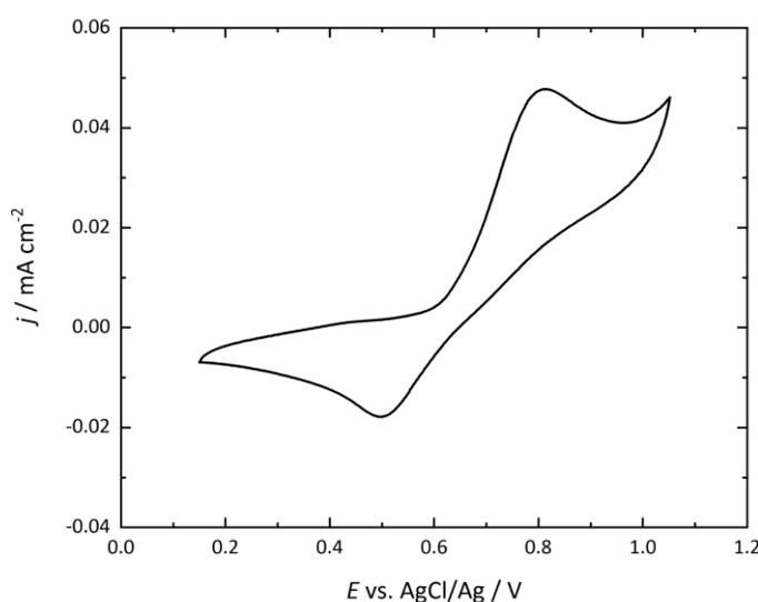
Figure 14: Cyclic voltammogram of **460** ( $E_{1/2}$  = 632 mV, 2 M HCl, scan rate 10 mV/s) measured by Hofmann et al.<sup>206</sup>
