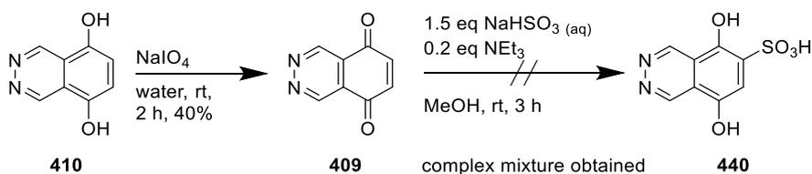
Scheme 174: Successful oxidation of DHP to DNQ and attempted reductive sulfonation.
