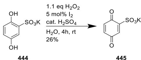
Scheme 171: Synthesis of 1,4-benzoquinone-2-sulfonic acid potassium salt.
