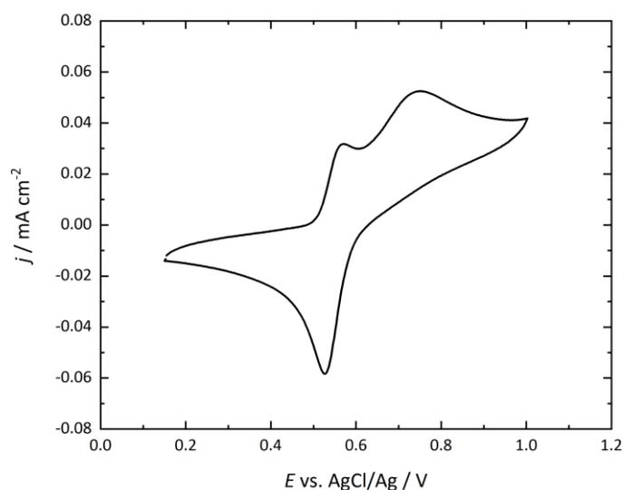
Figure 12: Cyclic voltammogram of DHP(SiPr) (2 M HCl, scan rate 10 mV/s) measured by Hoffmann et al.<sup>206</sup>
