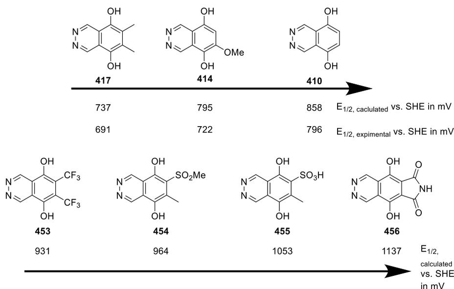
Scheme 181: Calculated potentials of DHPs based on computational studies of Mollenhauer et al. and experimental data measured by Hofmann et al.<sup>172</sup>
