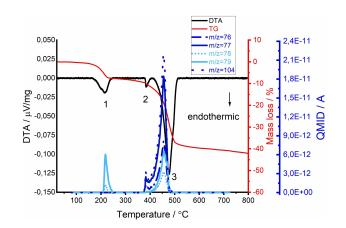
**Figure 8.** Simultaneous DTA/TG analysis together with mass spectrometry of  ${}^{33}_{\infty}$ [Tb(4-PyPz)<sub>3</sub>] (9) representing the series of isotypic frameworks 5–10. Two consecutive thermal decomposition steps are numbered in the heat-flow plot. The investigation was performed under a constant flow of argon (50 mL·min<sup>-1</sup>) with a heating from RT to 1000 °C at 5 K·min<sup>-1</sup>.
