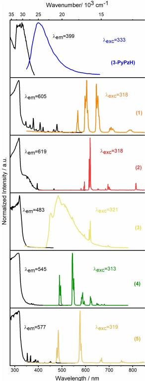
Figure 5. Normalized solid-state excitation (black) and emission (colored) spectra of  ${}^{3}_{\infty}$  [Ln(3-PyPz)<sub>3</sub>], Ln = Sm, Eu, Gd, Tb, Dy (1–5) at 77 K. Wavelengths for which the spectra were recorded are reported in the legends.
