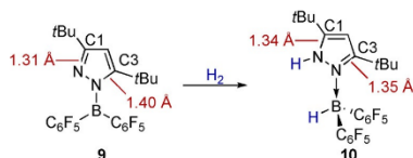
Scheme 5. Changes in the bond lengths of the heterocycle upon hydrogen activation by 9 derived from SCXRD structures.
