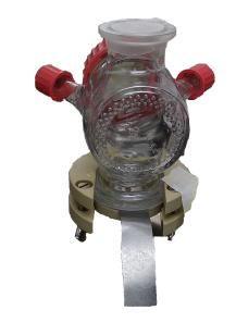
FIGURE 3.5: One WE chamber is shown, prepared for LbL-coating. The ITO electrode and graphite paper were mounted to the glass body and coating solution was added through the second flange. During incubation the flange was covered with parafilm. Reactors were incubated shaking in this upright position.
