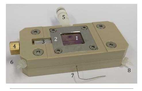
FIGURE 3.8: Flow cell with ITO (1) anode and steel frame for attachment on top (2), Pt-contacting (3) to the brass screw (4) used for anode contacting, inserted RE (5), WE chamber influx (6), Pt-wire for cathode contacting (7), CE chamber efflux on the right (8).
