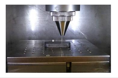
FIGURE 3.6: A sample in the HR-SKP chamber with the tip positioned few  $\mu$ m above the measured surface.
