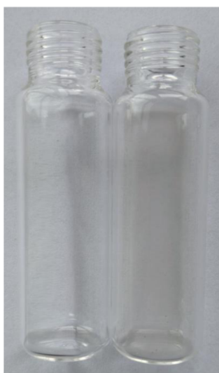
Fig. 4 Reaction vials with an inner PDMS layer for the experiments with embedded Pd/Al 2 O 3 catalysts. Left: pure PDMS without Pd/Al 2 O 3 ; right: PDMS including Pd/Al 2 O 3 (0.3 mg).
