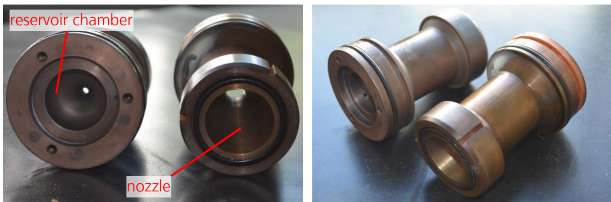
Fig. 40: Nozzle core parts with 2 mm and 10 mm throat diameter
