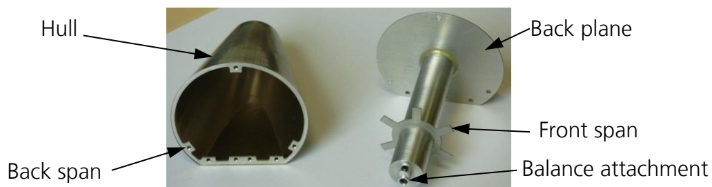
Fig. 23: Light weight COLIBRI test article, hull (left), inner structure (right)
