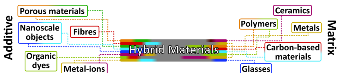
Figure 5. An overview of the concept of hybrid material design, which involves the combination of various additives and matrices. It should be noted that this overview does not imply the completeness of additives and matrices used for hybrid material synthesis, as only selected examples are given.
