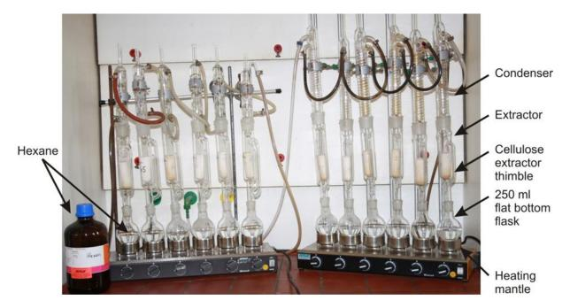
Figure 13: Soxhlet apparatus used for measurement of oil content
