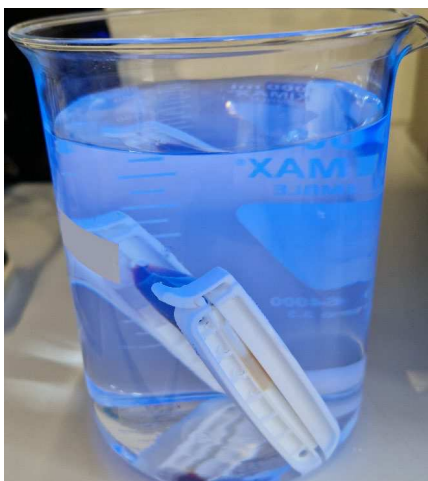
Figure S30. Fluorescent dialysate under UV irradiation (365 nm) of CA-1 CNDs after 12 hours of dialysis.
