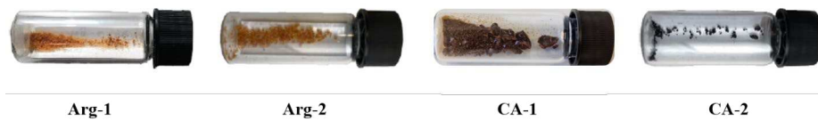
Figure S15. Visual appearance of the different CNDs ( Arg-1 , Arg-2 , CA-1 , and CA-2 ) after purification and freeze-drying.
