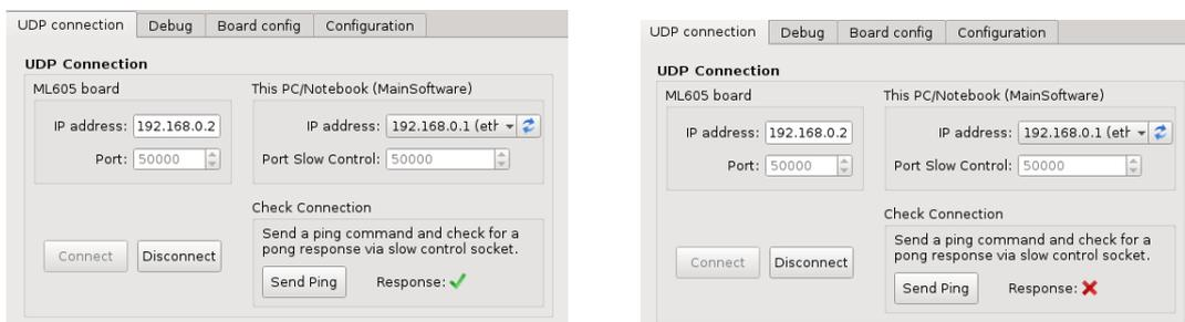
Figure 5.8: Connection interface in the JDRS. In the figure on the left the connection was successful since the response mark is green while on the right figure the mark is red meaning that the connection has failed.
