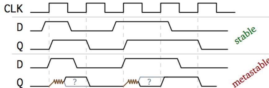
Figure 2.18: Representation of a Flip-Flop output in two cases: in first one the input is sufficiently far from the leading edge of the clock while in the second one is contemporaneous leading to an output that is metastable [78].
