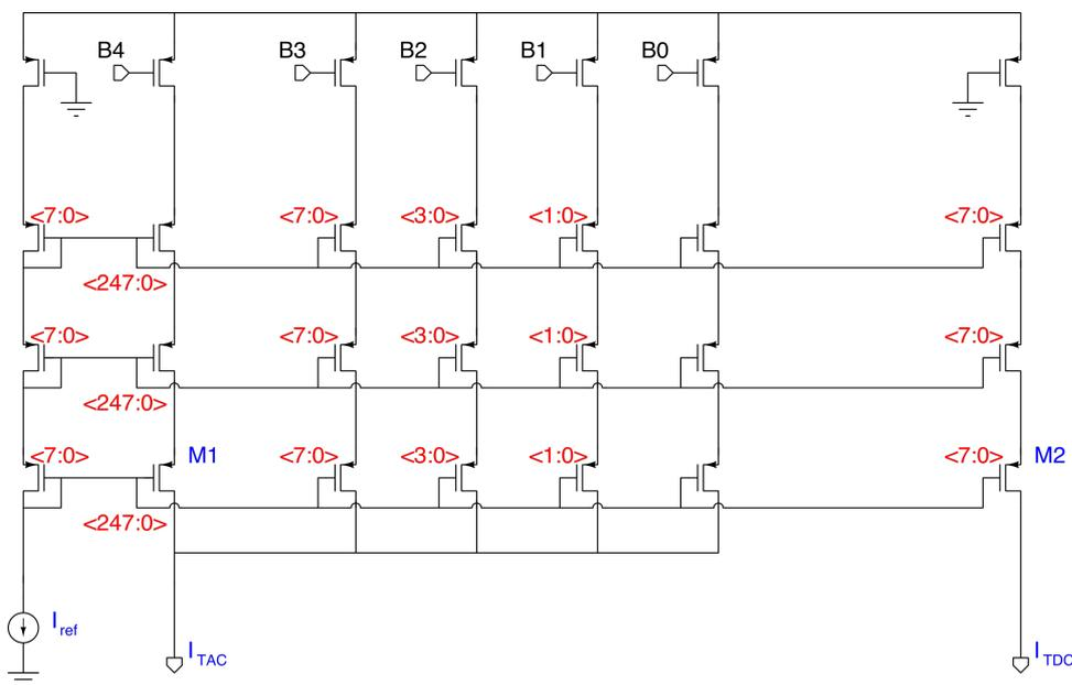
Figure 3.12: Schematic of a double cascoded current source with three branches: reference branch,  $I_{TAC}$  branch and  $I_{TDC}$  branch. The structure in the middle is a DAC used to tune the current  $I_{TAC}$ .
