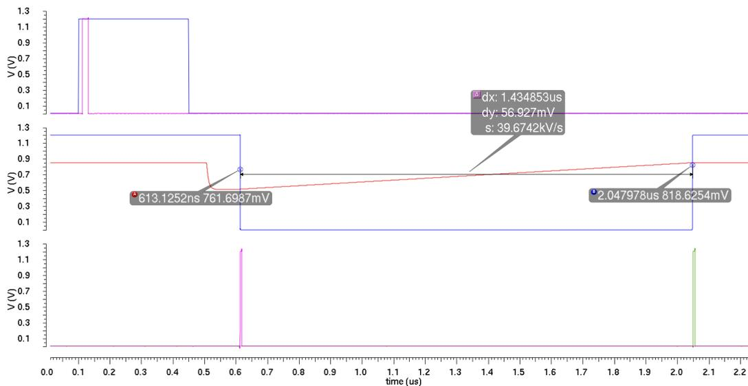
Figure 3.33: The first graph shows the DOT and the coarse time. In the second graph there is the voltage value on the capacitor  $C_{TDC}$  in red while the blue signal is the output of the latched comparator. In the third graph the digital signal SOC can be seen in magenta and the EOC in green.
