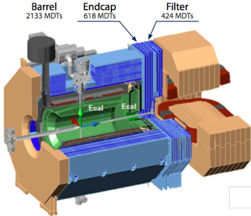
Figure 1.24: Layout of the muon detector with the respective MDTs [59].
