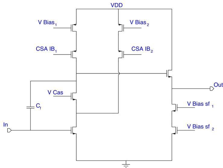
Figure 3.2: Architecture of the CSA implemented in PASTA.
