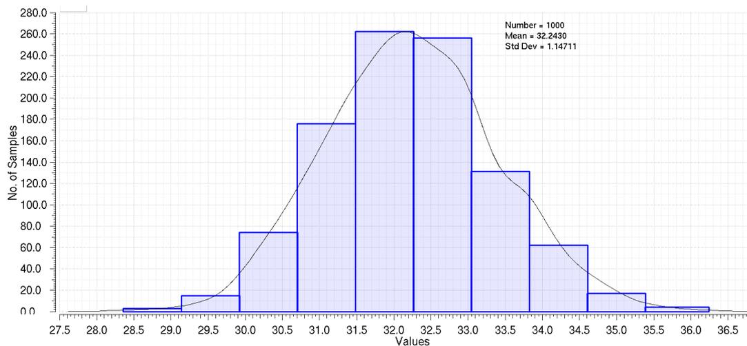
Figure 3.20: Distribution of the ratio of the currents  $I_{TAC}/I_{TDC}$  for the new current source.
