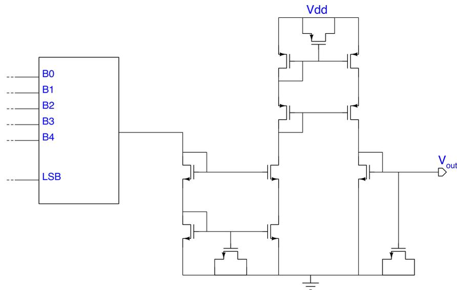
Figure 2.27: Third stage for a N-MOS connection, in this specific case with only voltage output.
