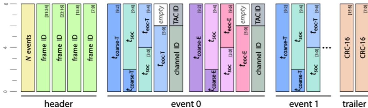
Figure 2.24: Example of a complete output frame in *PASTA* in the Full event mode [78].
