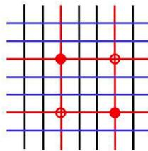
Figure 1.37: The two full dots are the real hits, the other two are the ghost points.
