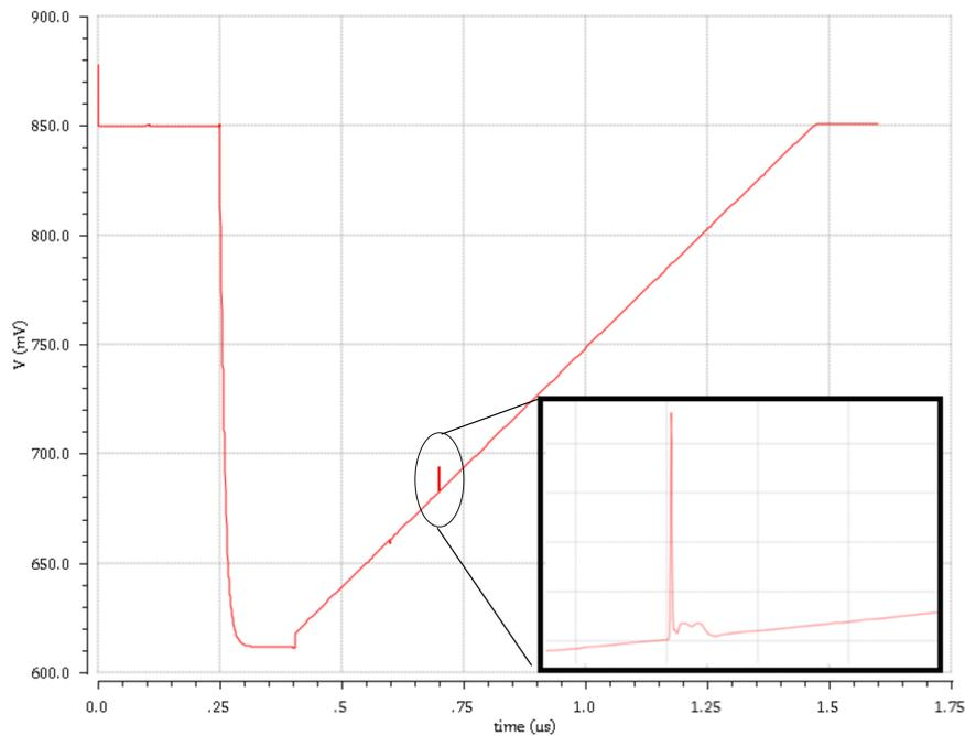
Figure 4.12: Shown in red is the voltage value on  $C_{TDC}$  during a simulation with the schematic generated by the PEX. It is possible to see that in the middle of the recharging ramp there is a glitch injected through a parasitic capacitor. On the right there is a zoom of the spike.
