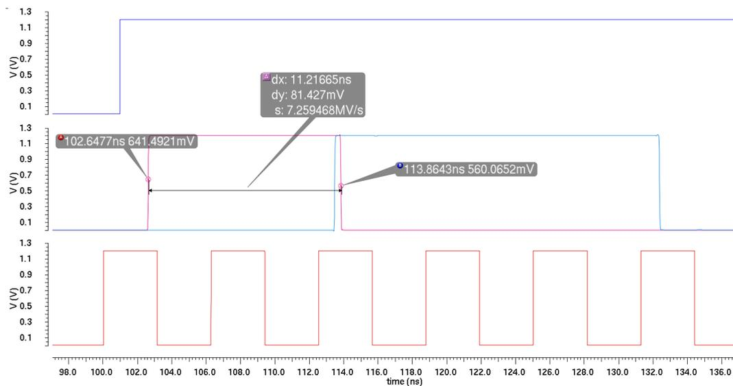
Figure 3.32: Combined simulation of both the local controller and the TDC. The blue signal in the first graph is the DOT, in the second graph the light blue represents the coarse time, the magenta signal is the fine time while the third graph shows the main clock.
