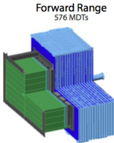
Figure 1.30: Layout of the muon detector for the forward spectrometer [63].
