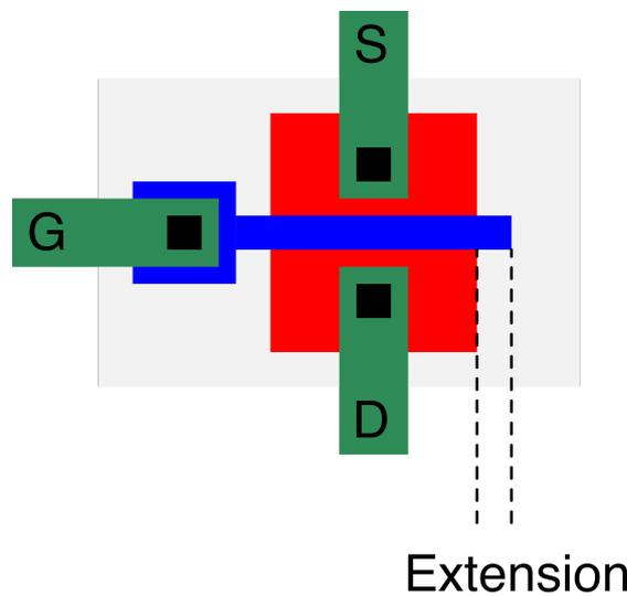
Figure 4.2: Polysilicon line (blue) that exceeds the active area (red).
