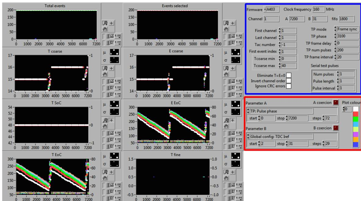
Figure 5.6: Measurement interface in the LabView system. In blue there is the measurement parameters region, in red is the region where the variables that are to be scanned are defined.
