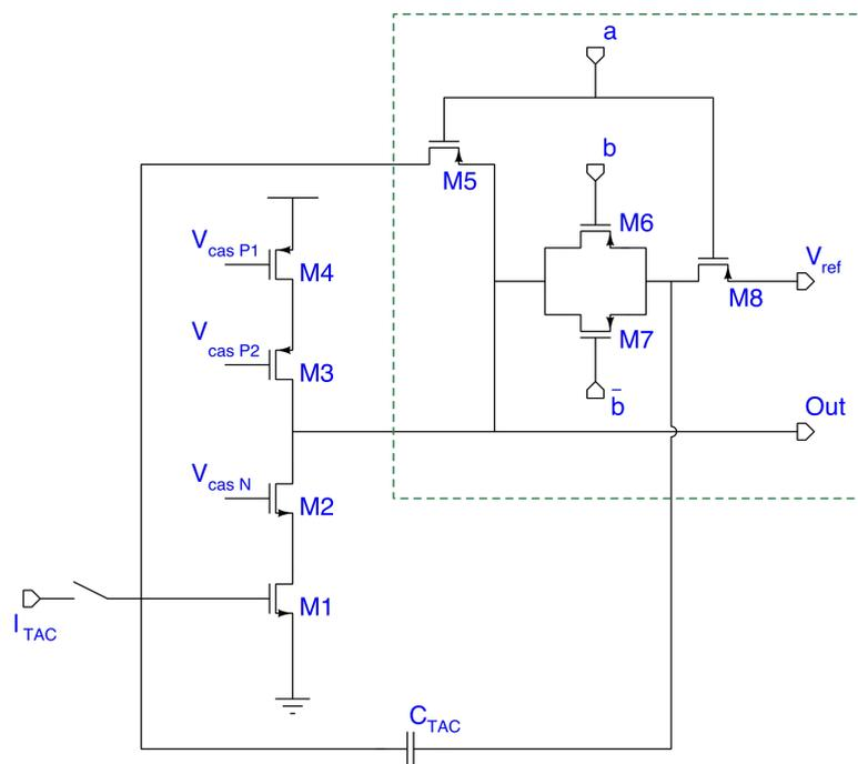
Figure 3.25: Schematic of cascoded amplifier.
