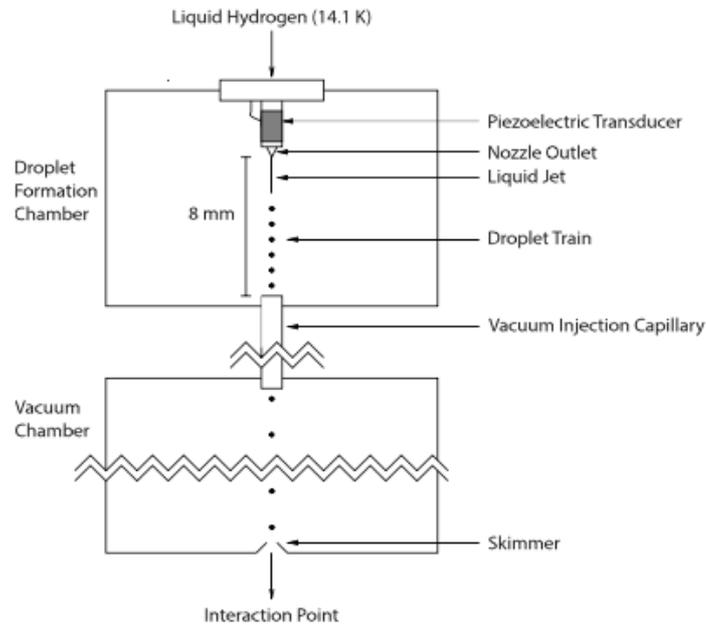
Figure 1.12: Schematic for the pellet target system developed for  $\bar{P}ANDA$  [46].
