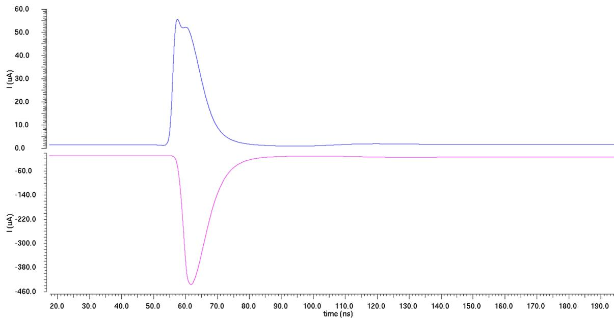
Figure 3.5: The output of the preamplifier stage is injected to the current buffer and is represented by the blue signal. The output of the current buffer is shown in purple.
