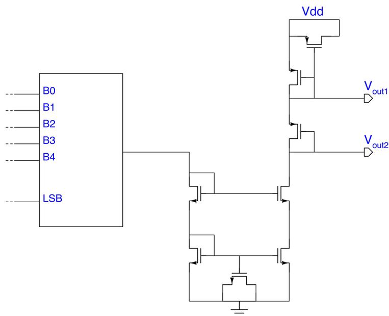
Figure 2.26: Third stage for a P-MOS connection with two voltage outputs.
