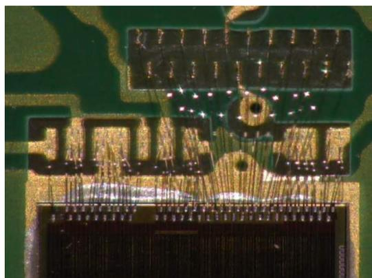
Figure 5.2: Picture of the PASTA wire bonded to the PB with 17  $\mu\text{m}$  diameter wires[85].
