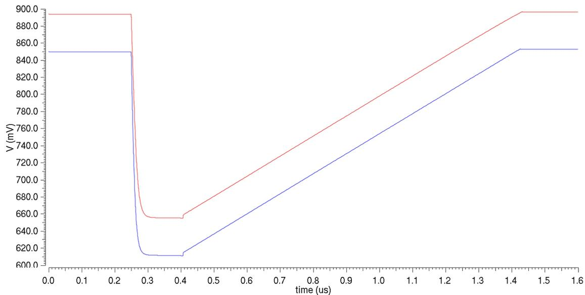
Figure 4.14: Simulated effect of the parasitic resistors between each channel on  $V_{ref}$ . The voltage value on the capacitor  $C_{TDC}$  in the channel “0” (blue) and in the channel “63” (red) are shown. It can be seen that in the last channel the recharging phase is shorter with respect to the first channel.
