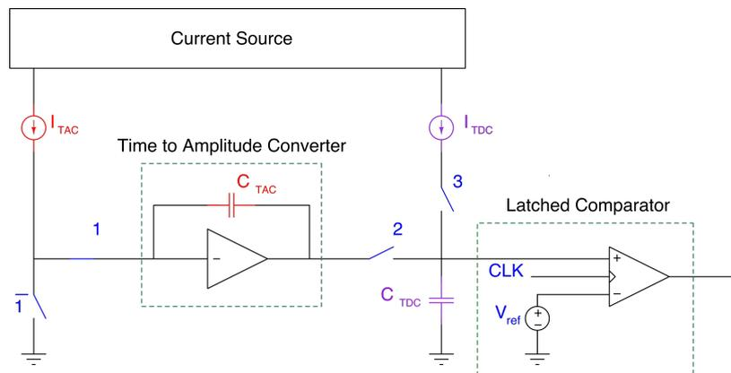
Figure 2.12: During the discharging phase of TDC the value of the switch number 1 is changed .
