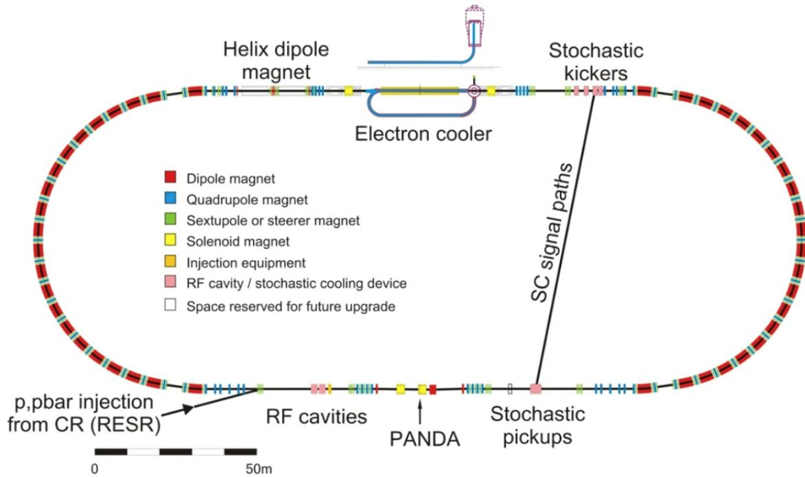
Figure 1.10: Scheme of the HESR used to accelerate and store antiprotons [45].
