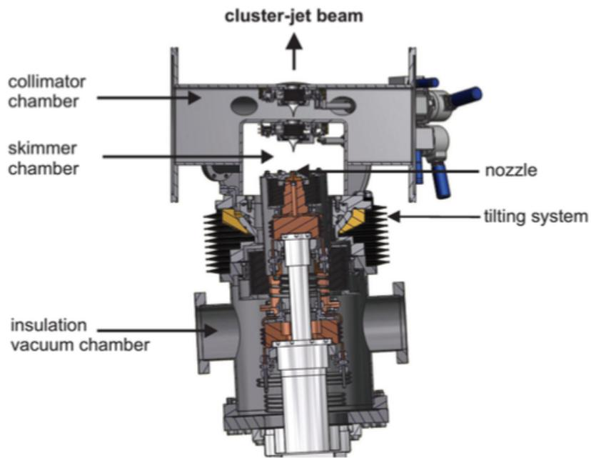
Figure 1.11: Design for the jet cluster target system developed for  $\bar{P}ANDA$  [46].
