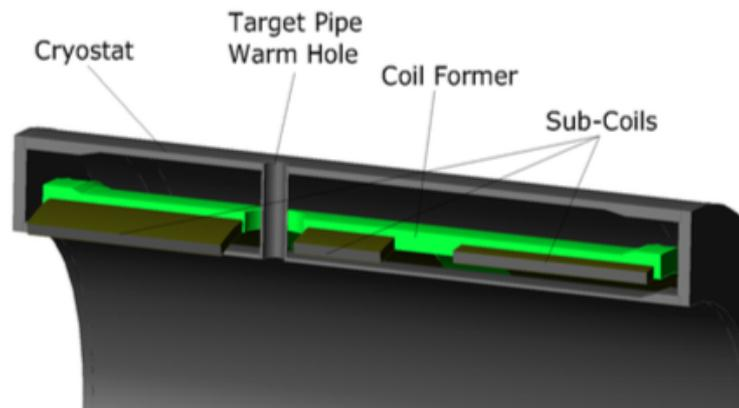
Figure 1.23: Section view of the Solenoid magnet [58].
