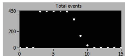
Figure 5.18: Events registered from the chip as a function of several threshold levels.
