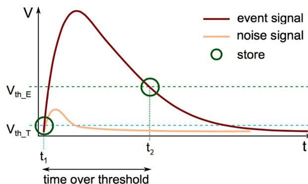
Figure 2.2: In *PASTA* the *ToT* is performed using two different threshold: one close to the base line to give a precise time stamp and the other as higher as possible to reduce the jitter in the falling edge of the signal and to be less sensible to the noise [80].
