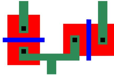
Figure 4.7: Asymmetric layout, that can cause mismatching between the two transistors.
