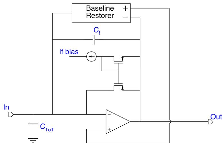
Figure 3.6: ToT amplifier stage made by an amplifier with a high gain with feedback circuits: a constant current generator, a capacitor  $C_f$ , and a baseline restorer.
