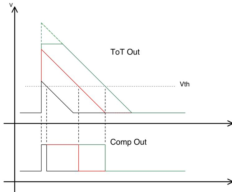
Figure 2.8: In the upper part there is the output signal of the ToT stage while in the lower graph is represented how the ToT is performed. Notice that the output of the comparator is proportional only to the length of the signals.
