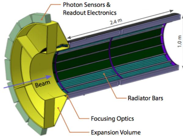
Figure 1.18: Layout of the Barrel DIRC detector [50].
