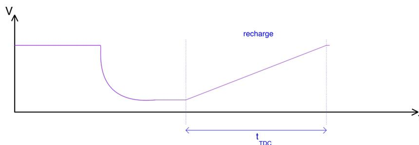
Figure 2.16: Voltage level of  $C_{TDC}$  during the recharging process.
