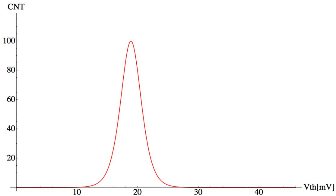
Figure 5.19: Derivative function of the threshold scan with an optimised Front-End:  $\mu=18.88$  mV,  $\sigma=1.80$  mV.
