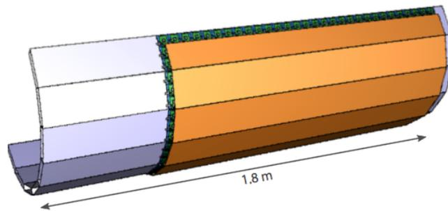
Figure 1.20: Layout of the Scintillating Tiles detector [54].
