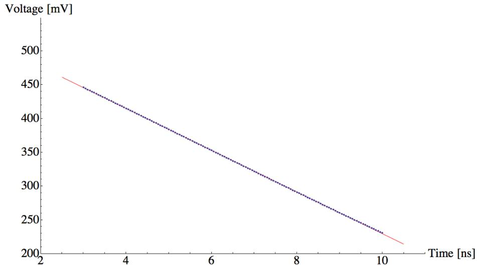
Figure 3.22: Voltage values reached by the folded cascode amplifier for different times (simulations, blue) and best fit to the points (red).
