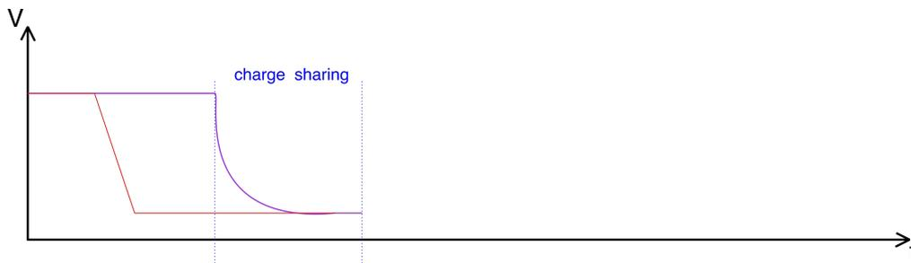
Figure 2.14: Voltage value for the  $C_{TAC}$  (red) and for the  $C_{TDC}$  (violet), after a certain time the two voltage value are equal.
