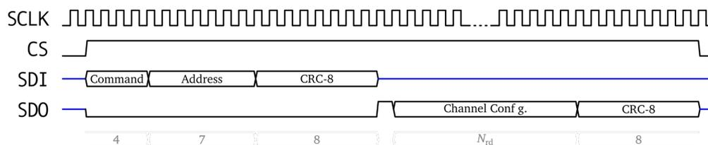
Figure A.2: Example of a reading command for the local configuration [78].
