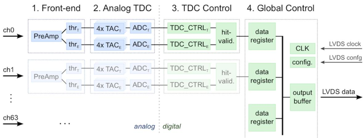
Figure 2.6: Building blocks for the PASTA core, in blue it is represented the analog environment while in green the digital domain [78].
