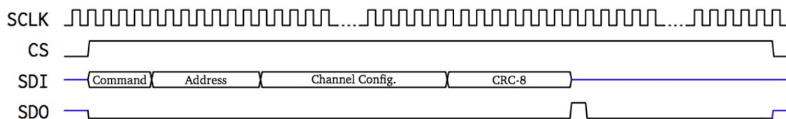
Figure 2.20: SDI structure for a channel configuration [78].
