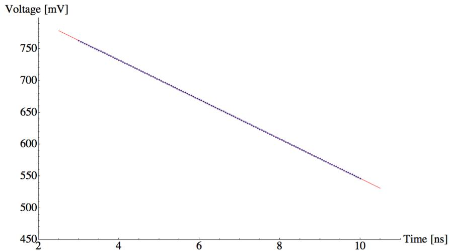
Figure 3.26: Different voltage value reached by the cascode amplifier for different duration of the discharging phase.
