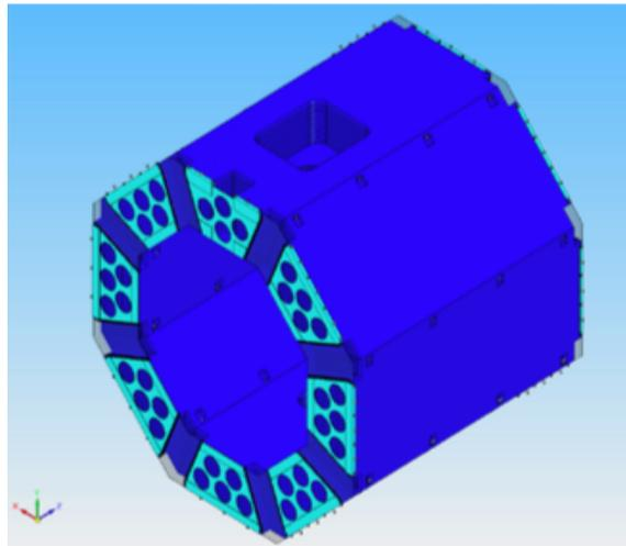
Figure 1.22: Layout of the Solenoid magnet [58].
