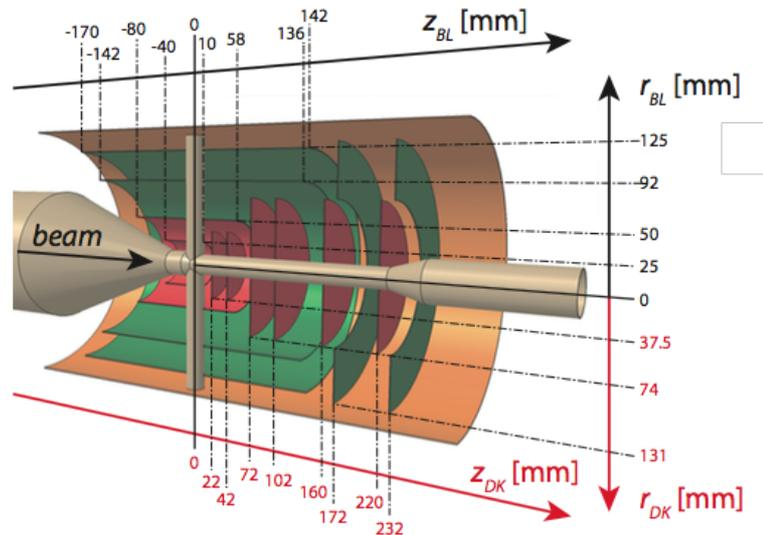
Figure 1.32: Geometrical layout of the MVD [69].
