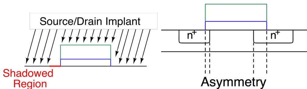
Figure 4.10: Representation of the gate shadow effect.
