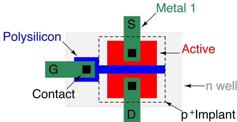
Figure 4.1: Layout of a p-mos transistor.
