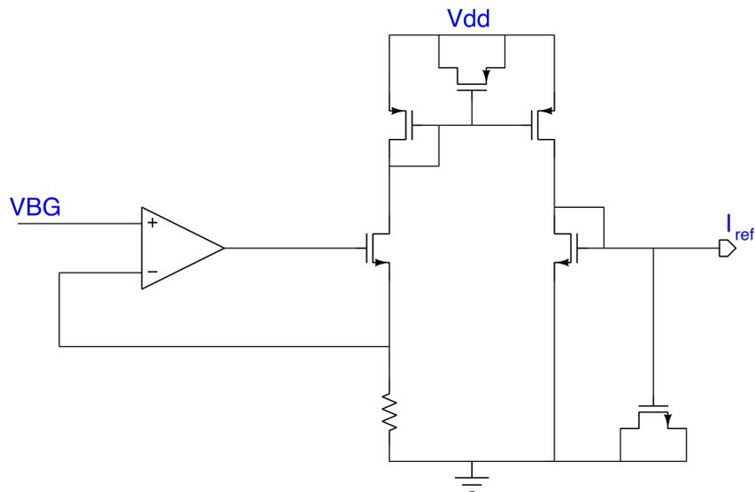
Figure 2.29: Structure that use an external voltage VBG to produce a very stable  $I_{ref}$  that is the current used from all the DACs in all the biasing cells.
