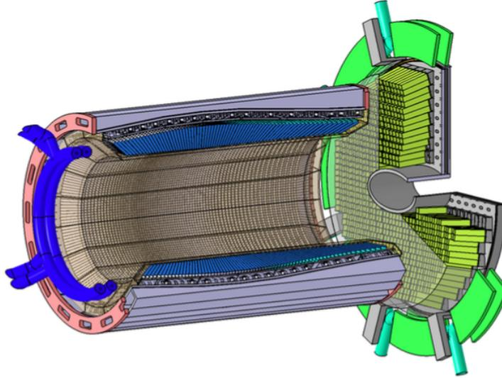
Figure 1.21: Layout of the Electromagnetic Calorimeter [56].
