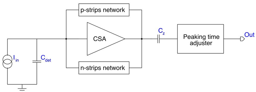
Figure 3.1: Representation of the building blocks of the preamplifier stage.
