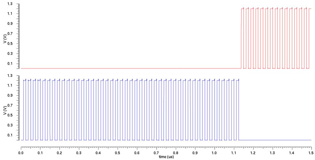
Figure 3.30: Output of the latched comparator (red the positive one, blue the negative one).
