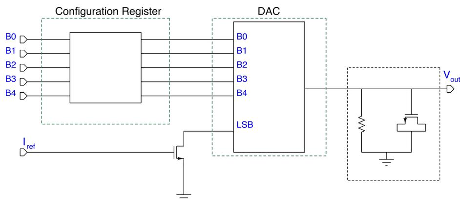
Figure 2.25: General *PASTA* bias cell schematic made by three structures. A configuration register necessary to buffer the configuration signals coming from the digital part, a DAC that set the needed current that has to be sent to the third group which can vary cell by cell.
