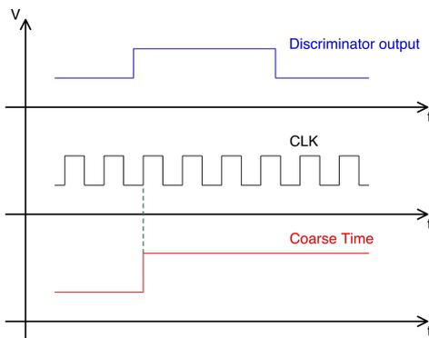
Figure 2.3: A coarse time measuring of an edge of the discriminator output is given by the clock.
