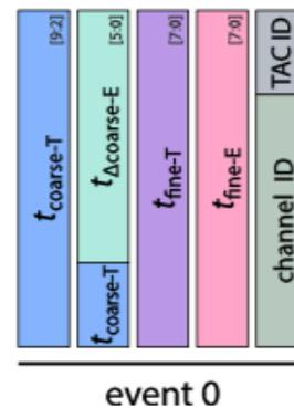
Figure 2.23: Compact event mode, useful during the normal operations. The data are pre-elaborated into the global controller reducing the redundancy.
