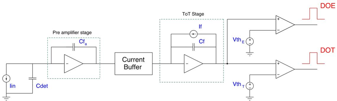
Figure 2.9: Schematic of the Front End chain used in PASTA, made by three stages and the comparators where the two different thresholds are applied.
