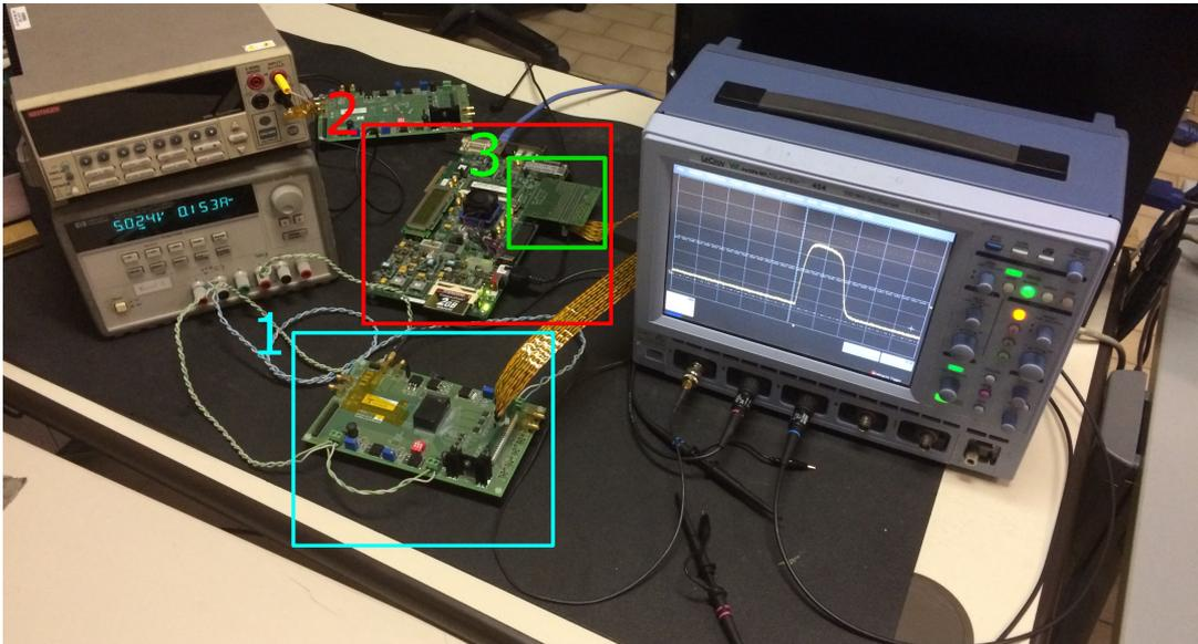
Figure 5.12: Photo of the laboratory setup used during the tests of **PASTA**. The **DISH** (azure box), the evaluation board (red box) and the breakout board (green box)
