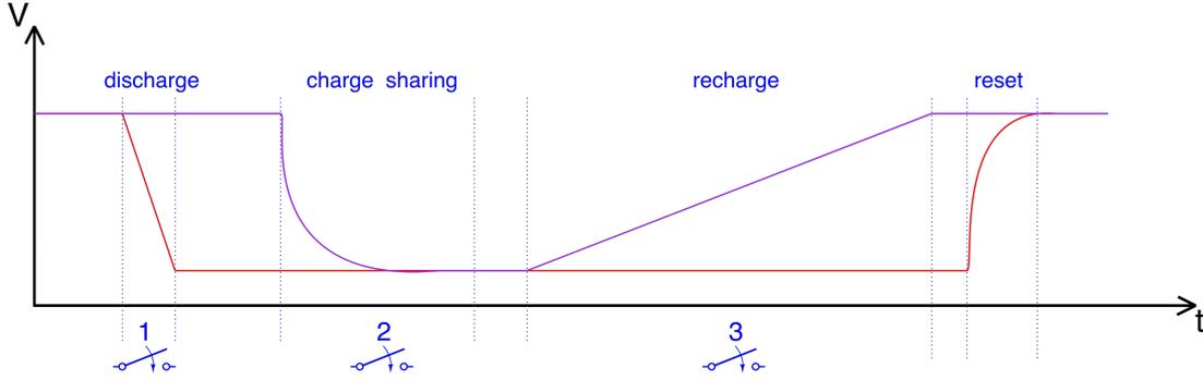
Figure 2.17: Complete process for the TDC, in red is reported the voltage value on the capacitor  $C_{TAC}$  while in violet on the capacitor  $C_{TDC}$ .
