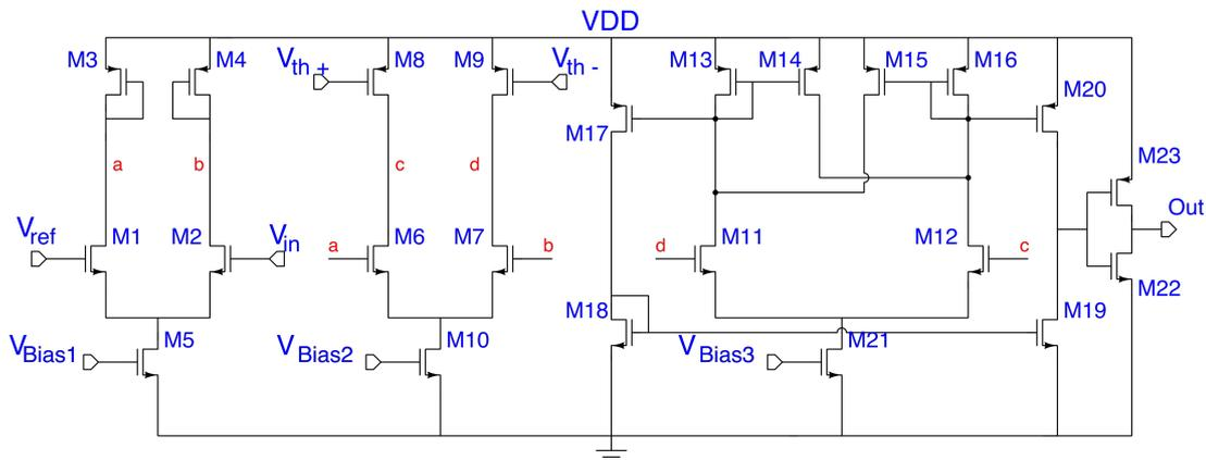
Figure 3.8: Schematic of the hysteresis comparator.
