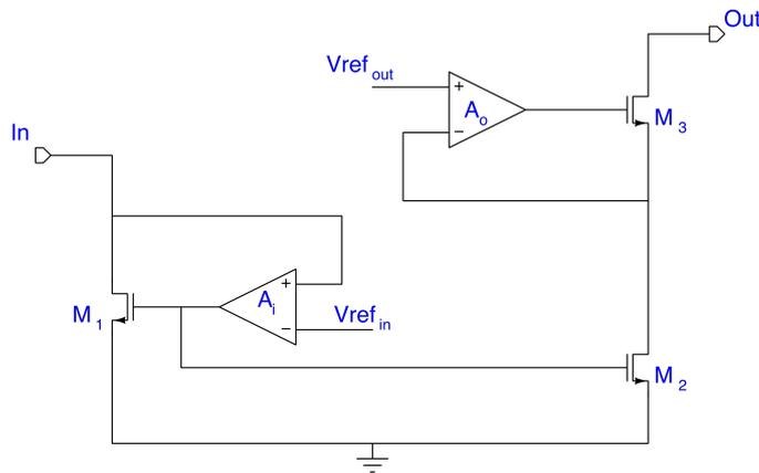
Figure 3.4: Current buffer architecture
