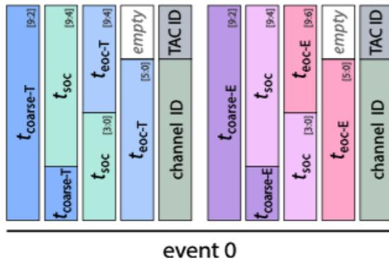
Figure 2.22: Full event mode, useful during the test phase. All the signals coming from the local controller are directly sent out with any modifications.
