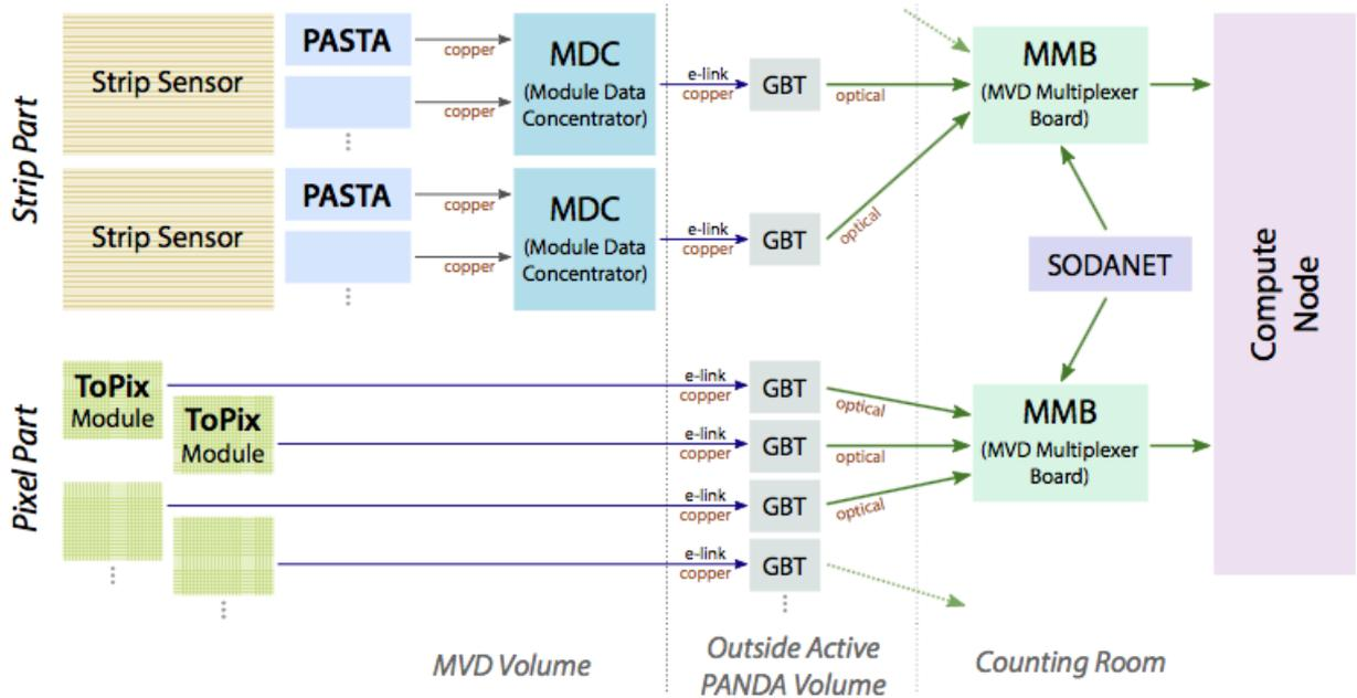
Figure 1.39: Block diagram for the MVD readout system from the sensor to the compute node.
