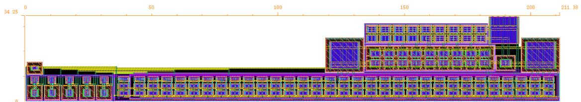
Figure 2.28: Layout of one bias cell, with a height equal to  $34.25 \mu\text{m}$  and a length of  $211.38 \mu\text{m}$ . In the bottom left there is the configuration register, then there is the DAC that cover all the bottom of the structure while in the upper right part there is the final stage.
