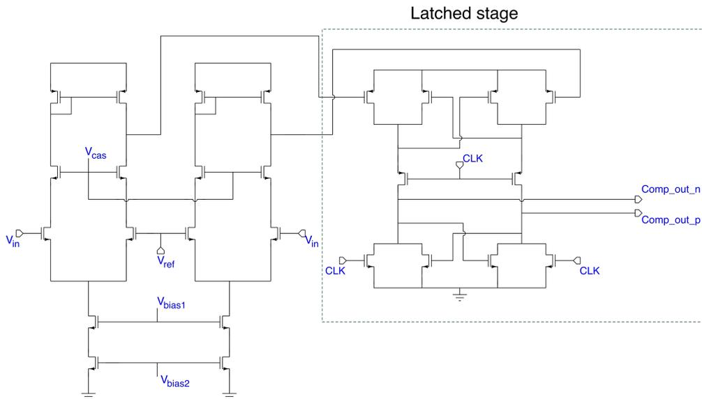
Figure 3.29: Schematic of the latched comparator.
