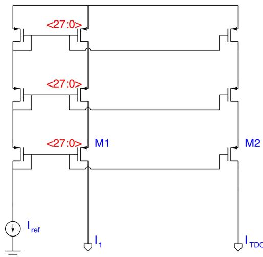
Figure 3.16: Schematic of the new current source based on the old structure.
