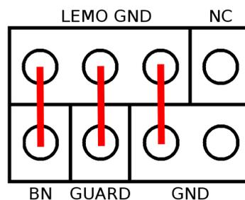
Figure 5.4: Pin header connections to select the biasing of the sensor. The LEMO GND is the ground of the HV used to bias the sensor. It is connected with the n-bulk of the sensor (BN) to the guard ring of the sensor (GUARD) and to the ground of the board (GND).
