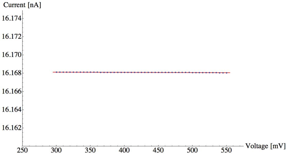
Figure 3.13: In blue the  $I_{TAC}$  current values for several voltage values are shown. The voltage range is the expected working region of the  $I_{TAC}$  branch. The red line is the best fit for the points.
