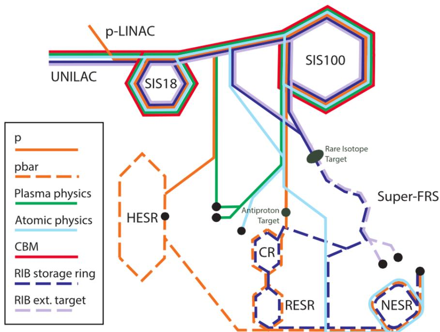
Figure 1.9: Several paths for the beam in the FAIR accelerators and storage rings [42].
