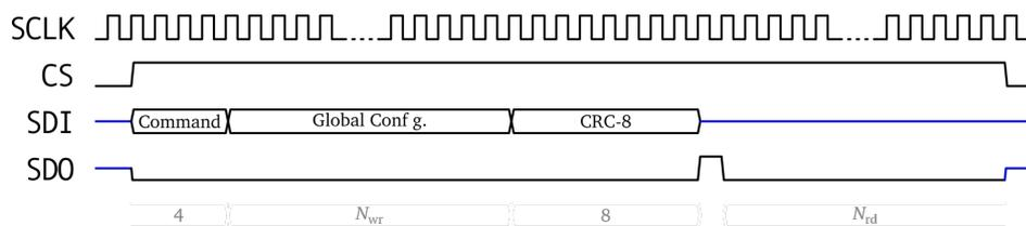
Figure A.3: Example of a write command for global configuration [78].
