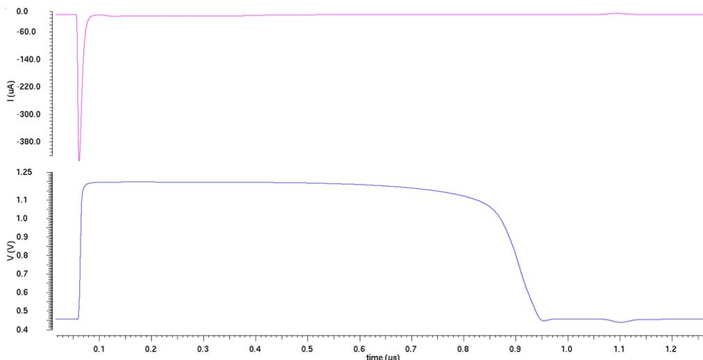
Figure 3.7: The input signal of the ToT amplifier stage is the purple signal while the blue one is the output that has to be processed by the comparators.
