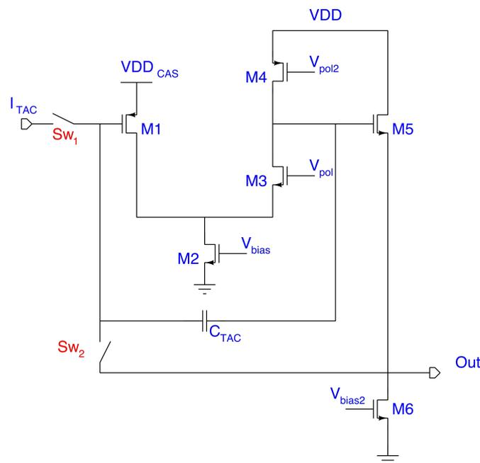
Figure 3.21: Schematic of a folded cascode amplifier.
