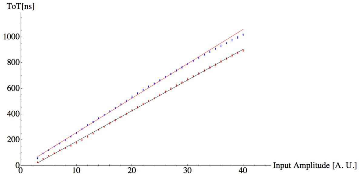
Figure 5.20: The blue (red) dots represent the  $ToT$  obtained as difference between “E coarse time” and “T coarse time”, in the case of p-type (n-type) strips, as a function of several input amplitudes of the test pulse. The red (black) line is the best fit of the data. The last five points of p-type configuration are not taken into account for the linear fit because there is a compression of the points for high charges.
