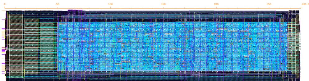
Figure 4.13: Layout of the local controller on which, in the left, there are the metal lines needed for the connections between the analog part of the channel and the local controller.
