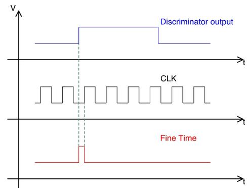
Figure 2.4: Fine time: time distance between the signal edge and the coarse time previously stored.
