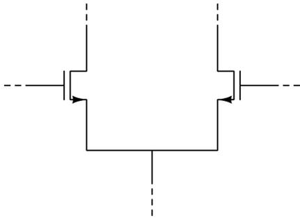
Figure 4.6: General differential input stage.
