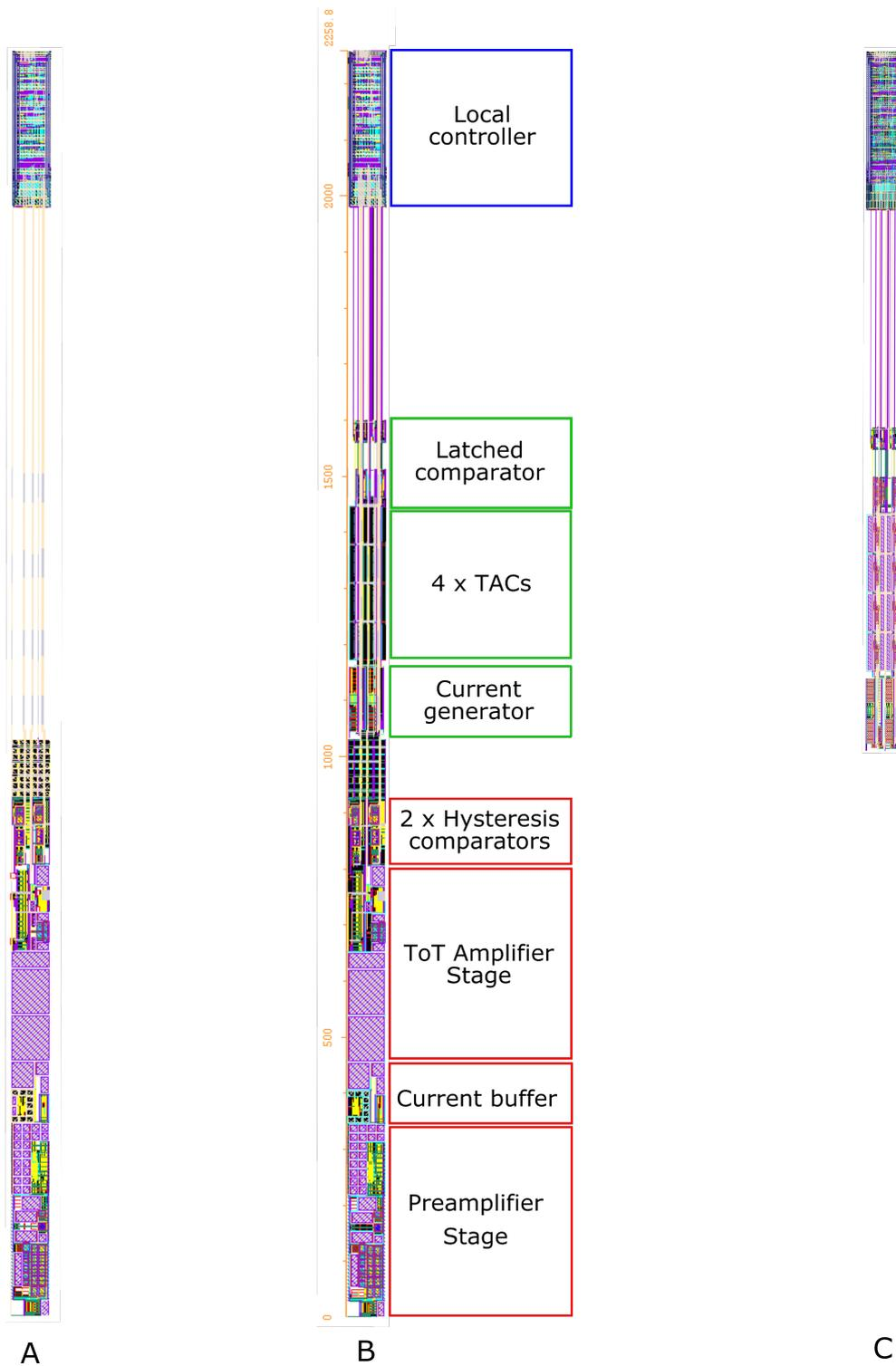
Figure 4.11: In figure B is shown the complete channel layout. The layout of the Front End with the connections to the local controller is shown in Figure A while the TDC and its connections to the local controller is shown in Figure C.
