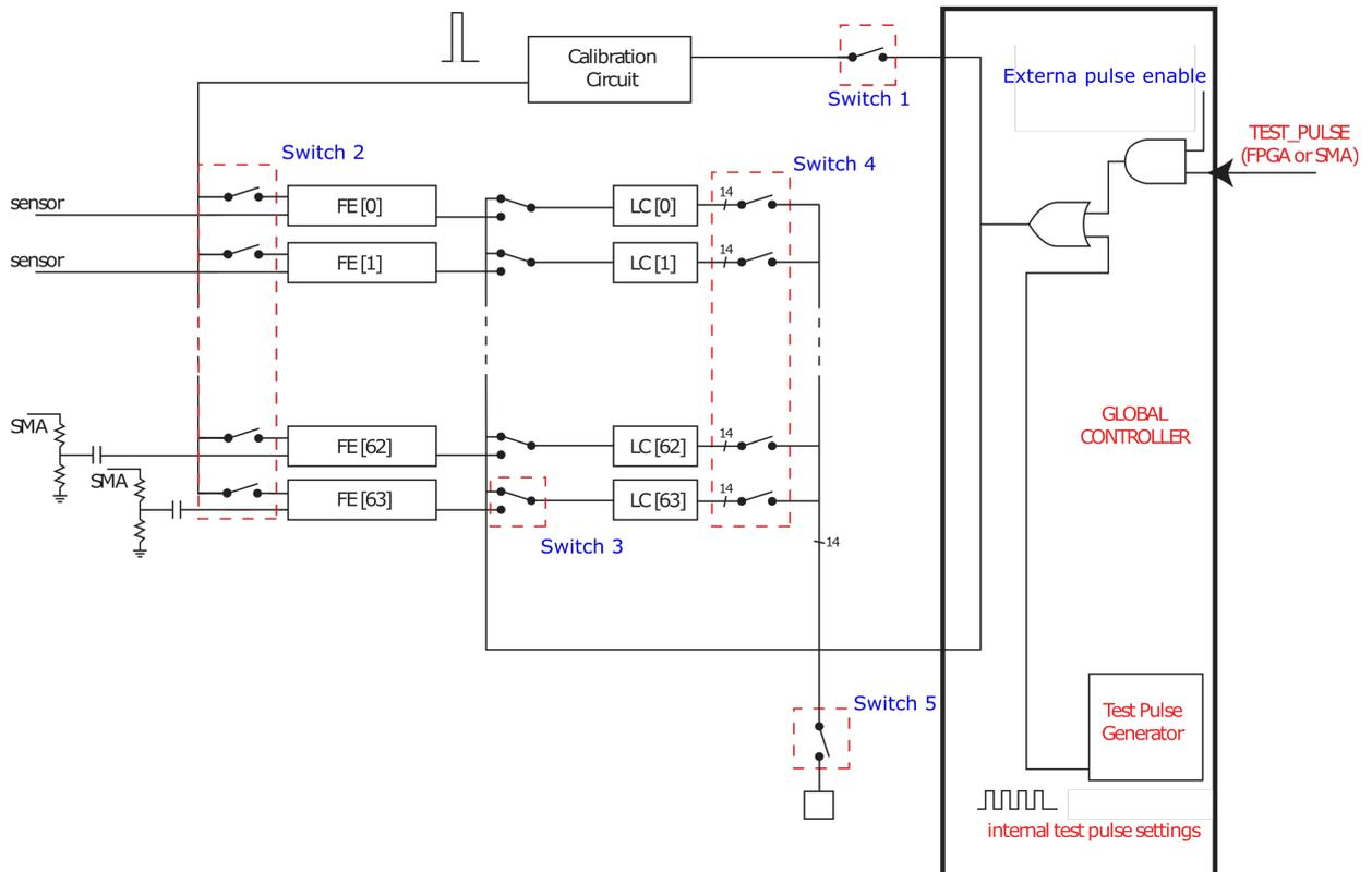
Figure 5.14: Schematic of the all possible test configurations in PASTA.
