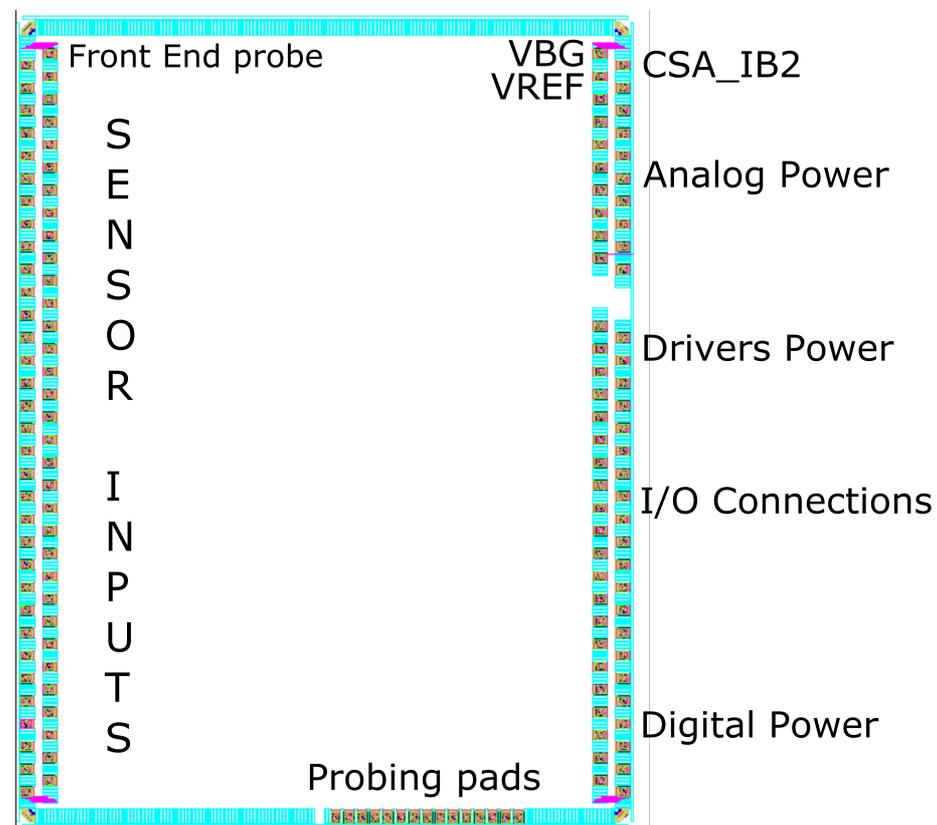
Figure 4.16: Final version of the layout of the pad ring and seal ring, placed on the [PASTA](#) edge.
