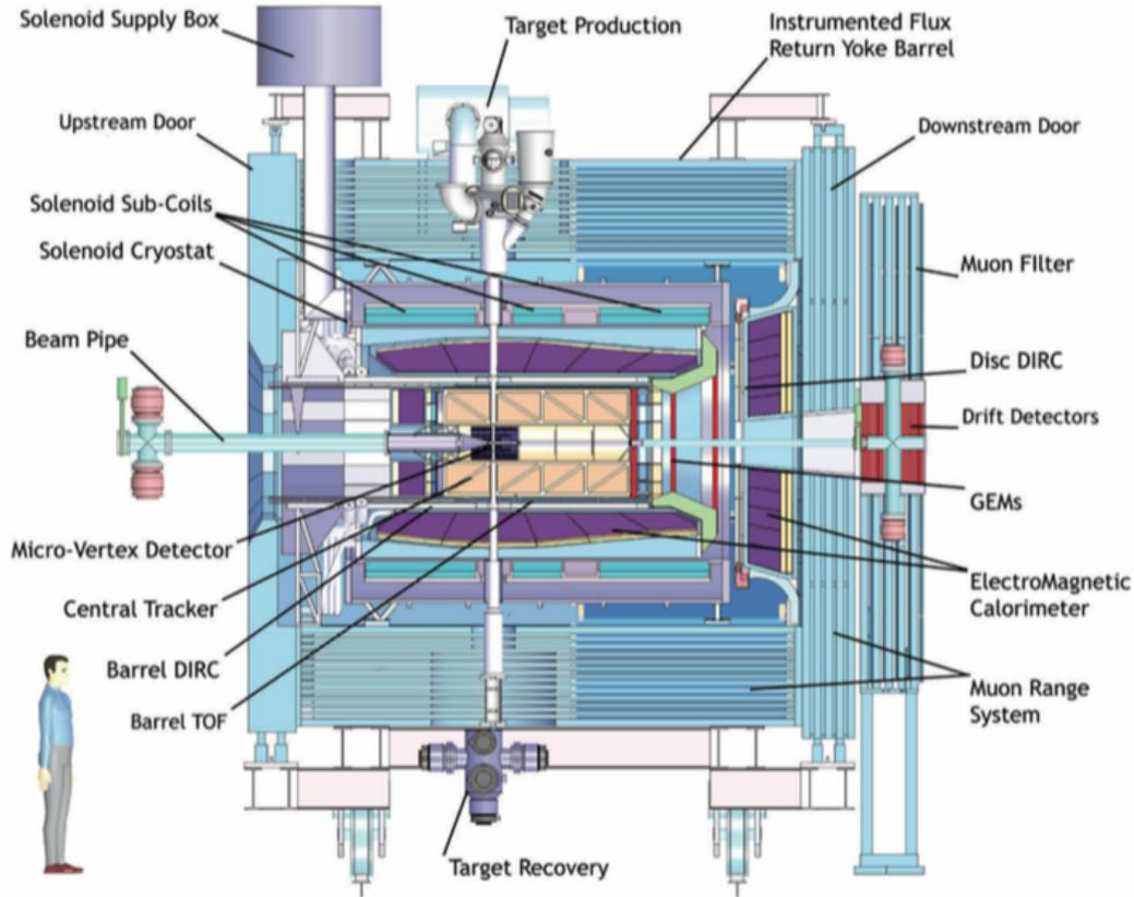
Figure 1.14: Layout of the Target Spectrometer.
