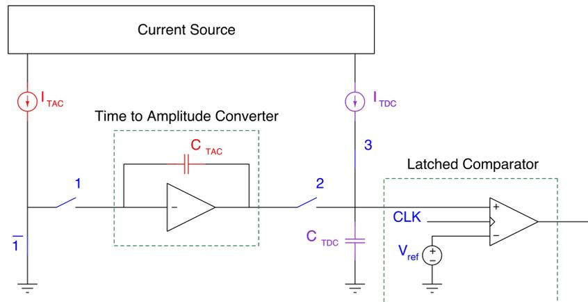
Figure 2.15: In the recharging phase the switch number 3 is close in order to recharge  $C_{TDC}$  with the current  $I_{TDC}$ .
