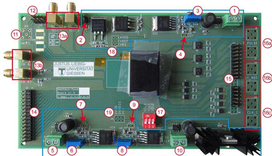
Figure 5.3: Photo of an assembled DISH with PASTA bonded on it. The chip is situated under the black box in the middle of the board. Details see text.
