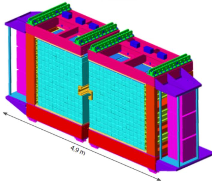
Figure 1.29: Layout of the forward calorimeter [63].
