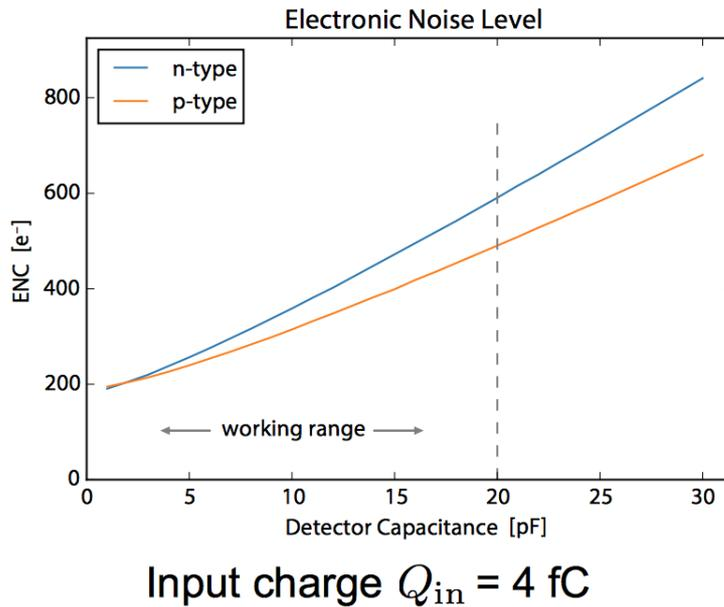
Figure 3.11: Different noise values expressed in terms of ENC for different capacitance with an input charge in the minimum ionising particle region [80].
