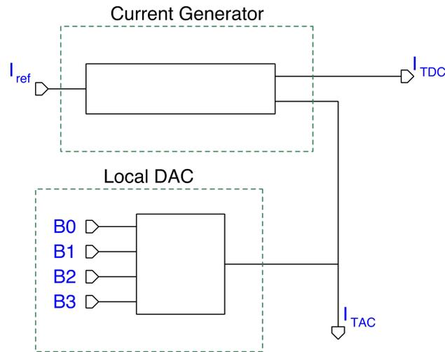
Figure 3.17: Structure needed to have the ratio 32 between the two currents and to tune the current  $I_{TAC}$ .
