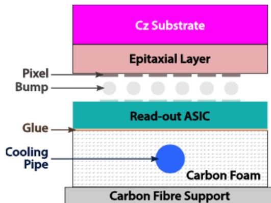
Figure 1.34: Cross-section of the hybrid pixel detector[45].
