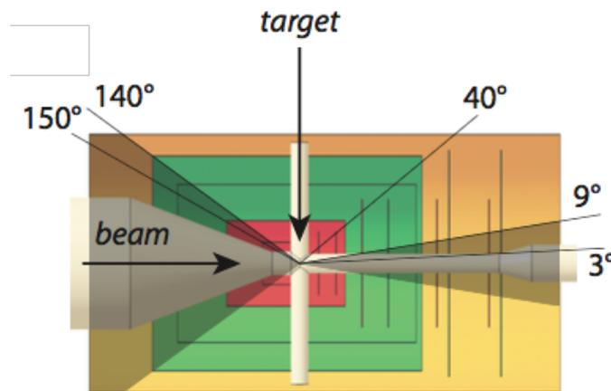
Figure 1.33: Geometrical layout of the MVD [69].
