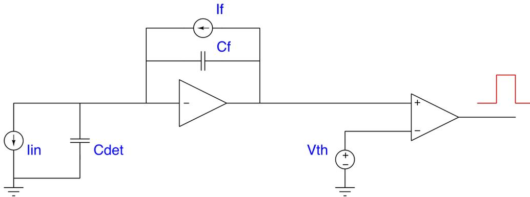
Figure 2.7: General Front End based on a **ToT** measurement, composed by an amplifier and a comparator.
