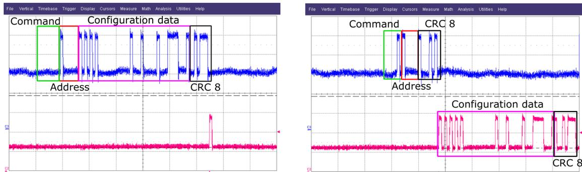
Figure 5.13: The left picture shows the **SDI** (blue) and the **SDO** (magenta) when the command “Write channel configuration” is sent to the chip. In the right picture the **SDI** and **SDO** are shown when the command “Read channel configuration” is sent.
