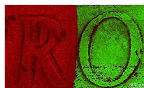
Figure 4. 3D-surface red-green overlay MS image of m/z 207.8941 (red, [\text{C}_4\text{HO}_3\text{NNi} + \text{K}]^+ ), and m/z 116.9527 (green, [\text{CH}_2\text{NZn} + \text{Na}]^+ ). MS images of the two signals were generated from a cleaned 1-Euro coin (2002, Germany) with 320 \times 189 pixels; 15 \mu\text{m} pixel size; m/z bin width: \Delta(m/z)/(m/z) = \pm 5 \text{ ppm} .
