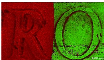
Figure 5. 3D-surface red-green overlay MS image of m/z 207.8941 (red, [\text{C}_4\text{HO}_3\text{NNi}+\text{K}]^+ ), and m/z 116.9527 (green, [\text{CH}_4\text{NZn}+\text{Na}]^+ ). MS images of the two signals were generated from a cleaned 1-Euro coin (2002, Germany) with 320 \times 189 pixels; 15 \mu\text{m} pixel size; m/z bin width: \Delta(m/z)/(m/z) = \pm 5 ppm.
