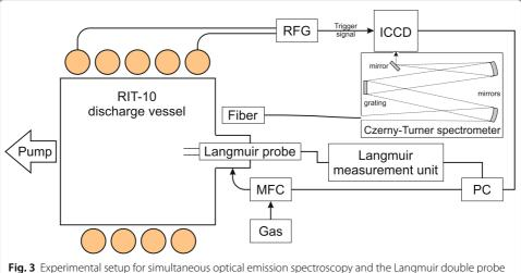
**Fig. 3** Experimental setup for simultaneous optical emission spectroscopy and the Langmuir double prob measurements
