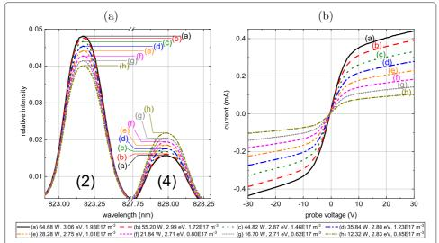
**Fig. 5** The two strongest lines (see Fig. 4) of intensity-normalized xenon spectra for a measurement series at 0.1 sccm gas flow at different operating points (see also Fig. 6) (**a**) together with the corresponding Langmuir double probe measurements (**b**). This series of spectra is part of the reference data set
