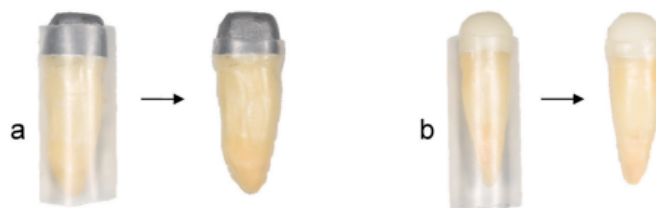
Fig. 4. Simulation of periodontal ligament using a shrink tube (a: sample teeth for group C; b: sample teeth for group D).
