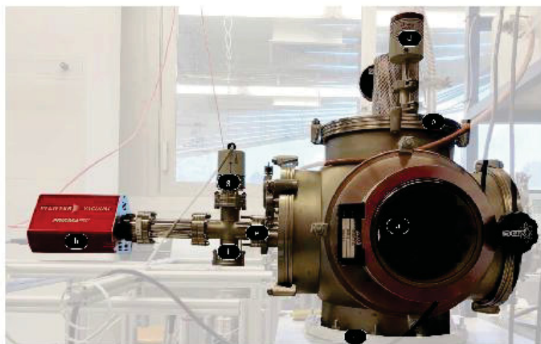
Figure S1: The plasma apparatus consisting of the main chamber (a), gas inlet (b), rotatory pump (below c), pressure sensor (d), double blind flange with capillary (e), turbomolecular pump (f), second pressure sensor (g) and quadrupole mass spectrometer (h).
