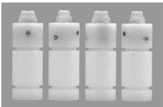
Fig. 3 CAD/CAM-milled human test abutment in the sample holder
