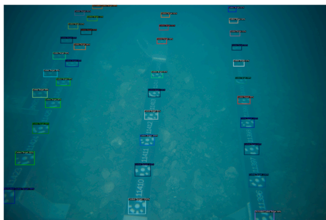
Fig. 3. Bounding-boxes, class and probability-score superposed on an original image. Haze appears frequently in underwater images.
