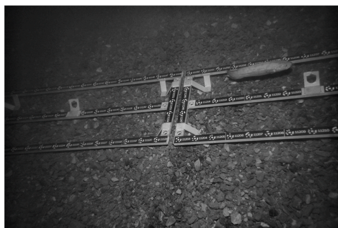
Fig. 5. CLAHE-processed gray-scale image. The enhanced contrast reveals additional markers close to the image border.
