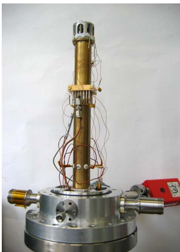
Fig.(2-5): A photo of the RFQ assembly mounted on a flange. The red box is a PIRANI-gauge. On the front side of the flange a gas inlet is mounted. Two feedthroughs are needed for DC and RF power supply.
