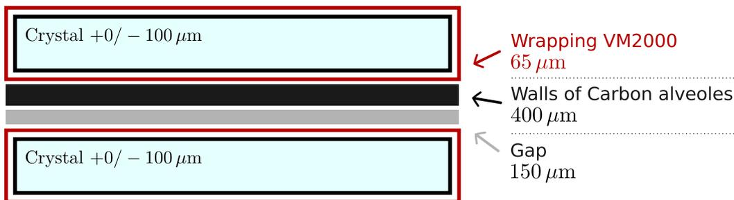
**Figure 3.2:** Each crystal has a geometrical tolerance of  $+0/ - 100\ \mu\text{m}$ . The gap of  $150\ \mu\text{m}$  considers mechanical tolerances ( $50\ \mu\text{m}$ ) and deformation of the alveoles ( $100\ \mu\text{m}$ ). Altogether the distance between the borders of two neighbouring crystals is in the order of  $680\ \mu\text{m}$  [34].
