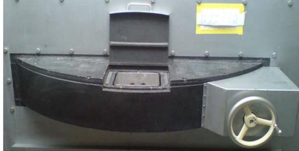
**Figure 2.14:** A compartment, which is installed in a circular moveable for irradiating different kind of samples. After a rotation of 180 the samples are exposed to a  $^{60}\text{Co}$  source.
