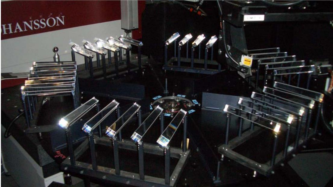
**Figure 2.10:** The moveable server of the ACCOS machine has a diameter of 1.1 m and is able to carry several crystals, including reference crystals, at the same time.
