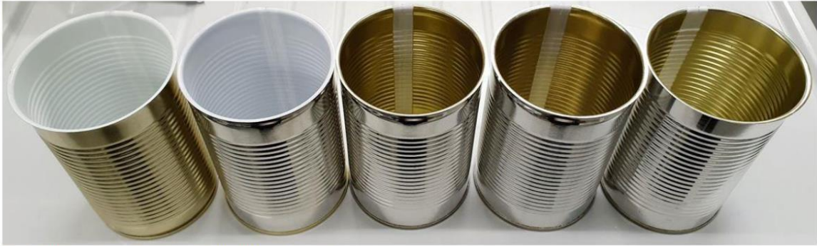
Fig. S3: Investigated tin cans with different coatings FCM model studied consisting of five different tin can coatings (ID 35-37, 39 and 65), kindly provided for research purposes by the packaging supplier to Nestlé Research, Switzerland.
