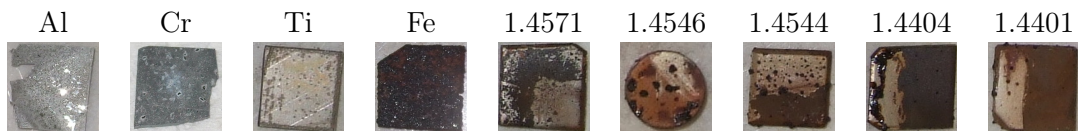
Figure 4.21: Samples treated according to scenario 4 and after a few days of exposure to ambient conditions, i.e., humid air.
