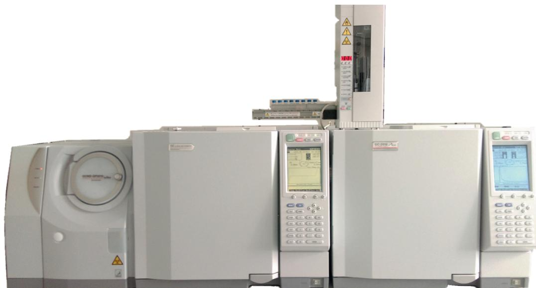
Figure 5: Multidimensional gas chromatography system (Shimadzu MDGC-2010) with two dimensions (first dimension: right, second dimension: middle) and mass spectrometer (left) (source: Florian Birk)
