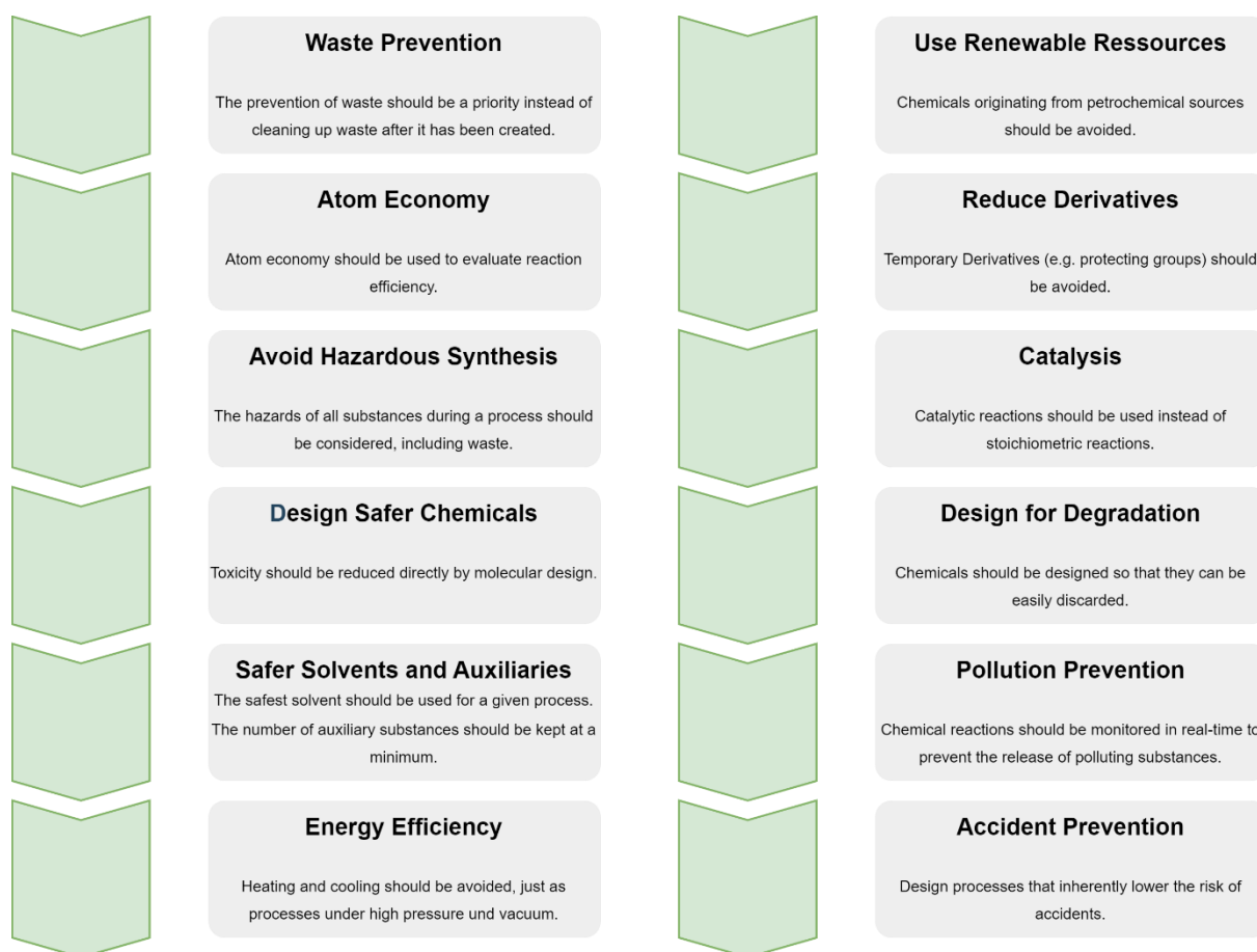
Figure 13: The twelve principles of green chemistry as described by Paul Anastas and John Warner .
