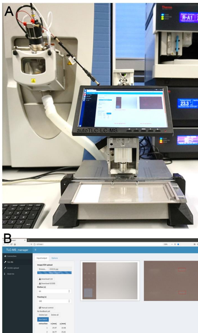
Fig. 1. autoTLC-LC-MS: Open-source add-on hardware (A) and software (B) of the multi-purpose autosampler for LC-MS.
